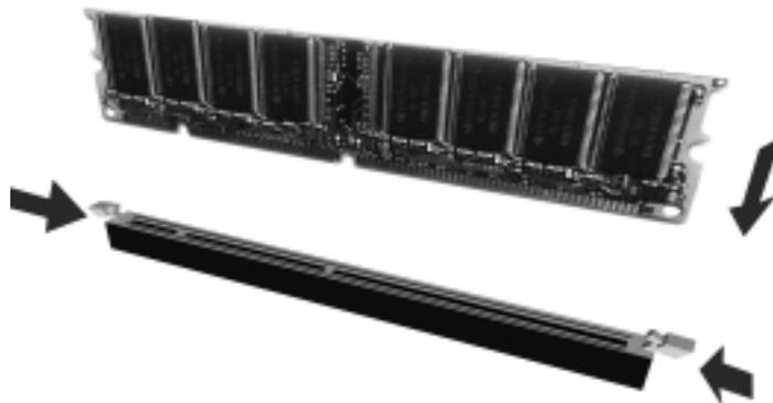
3. Position the DIMM above the connector so that the two notches on the bottom edge of the module align properly with the empty connector.
