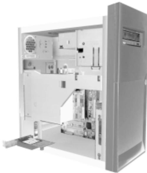
3. Remove the adapter from its static-protective package.
