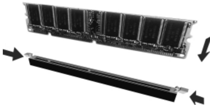
4. Firmly push the module straight down into the connector until the retaining clips pop up and fit snugly around both ends of the module.
