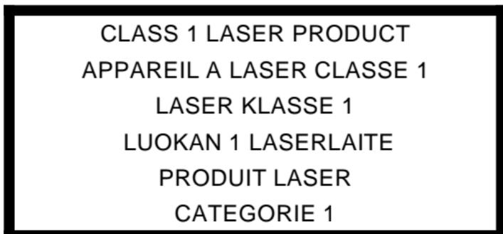
The CD-ROM drive is certified in the U.S. to conform to the requirements of the Department of Health and Human Services 21 Code of Federal Regulations (DHHS 21 CFR) Subchapter J for Class 1 laser products.
