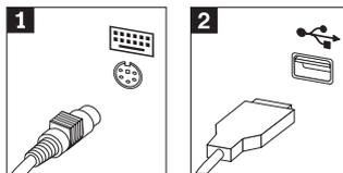
3. Your mouse cable might have a standard mouse connector **1** or a USB connector **2**. Connect the mouse cable to the appropriate mouse connector.
