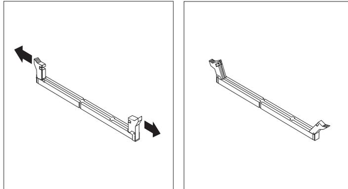
4. Make sure the notches in the DIMM align with the tabs on the connector. Push or insert the DIMM straight down into the connector until the retaining clips close.
