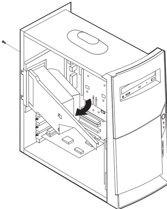
4. Remove the power supply and carefully lay it to the side.
