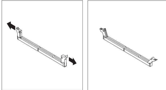
5. Make sure the notches in the DIMM align with the tabs on the connector. Push or insert the DIMM straight down into the connector until the retaining clips close.
