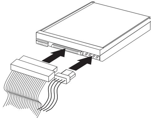
The steps to connect an IDE drive are different depending on the type of drive you are connecting. Locate the procedure below for your drive connection.
