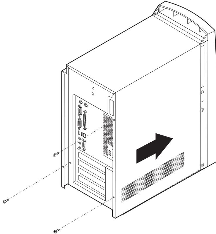
4. Lower the cover down over the chassis so that the rail guides engage the rails.
