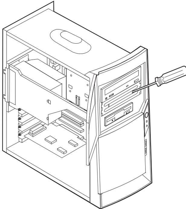
4. Make sure the drive that you are installing is set correctly as either a master or a slave device.
