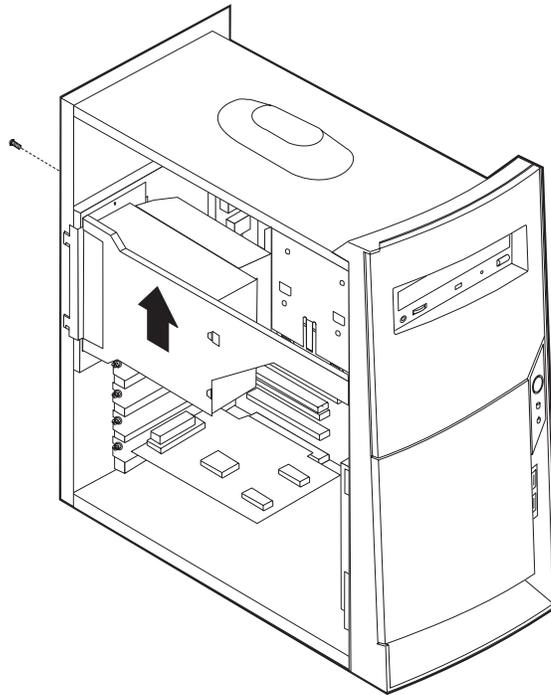
3. Rotate the power supply outward as shown.
