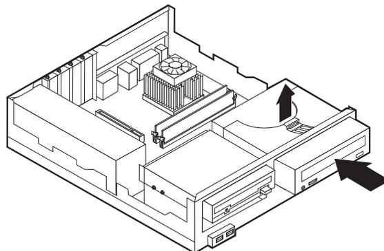
7. Each integrated drive electronics (IDE) drive requires two cables; a four-wire power cable that connects to the power supply, and a signal cable that connects to the system board. You might also have an audio cable to connect. To connect a CD drive or DVD drive to your computer, follow these steps.
