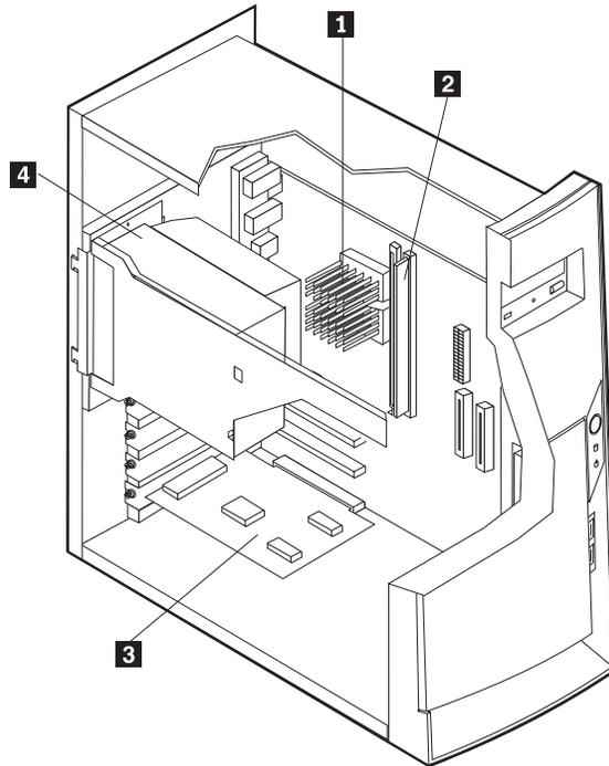
**1** Microprocessor and heat sink
