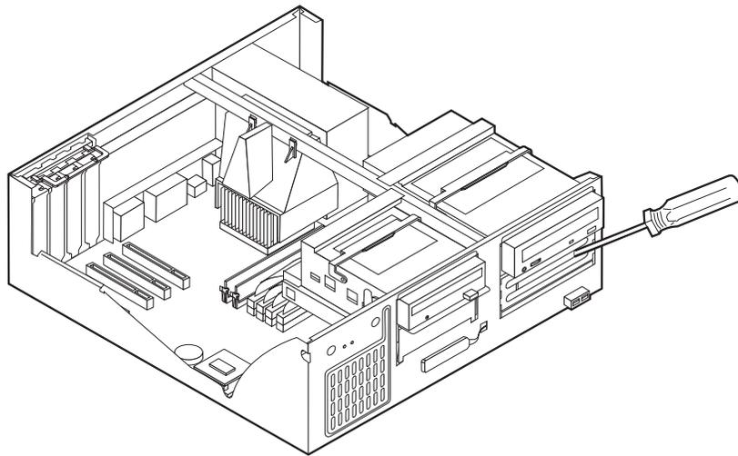
5. Pivot the drive bay latch handle toward the front of the computer and pivot the drive bay cage toward the front of the computer until the drive cage latch catches to the chassis.
