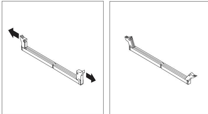
4. Make sure the notch in the DIMM aligns with the tab on the connector. Push or insert the memory module straight down into the connector until the retaining clips close.
