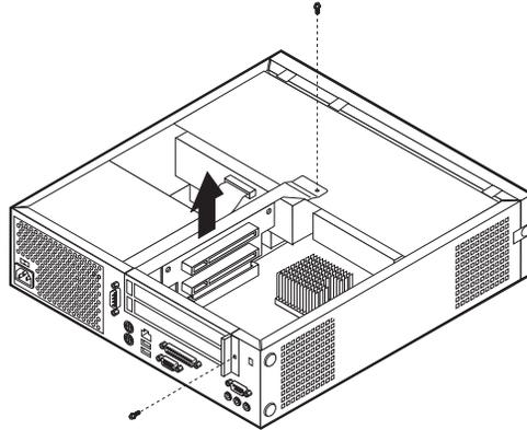
3. Remove the adapter-slot-cover latch and the slot cover for the appropriate expansion slot.
