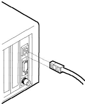
Connect the other end of the cable to the network.
