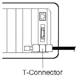
If the computer you are installing is not the last in the Ethernet network, attach cables from the Ethernet network to both ends of the BNC T-connector. (See the following figure.)
