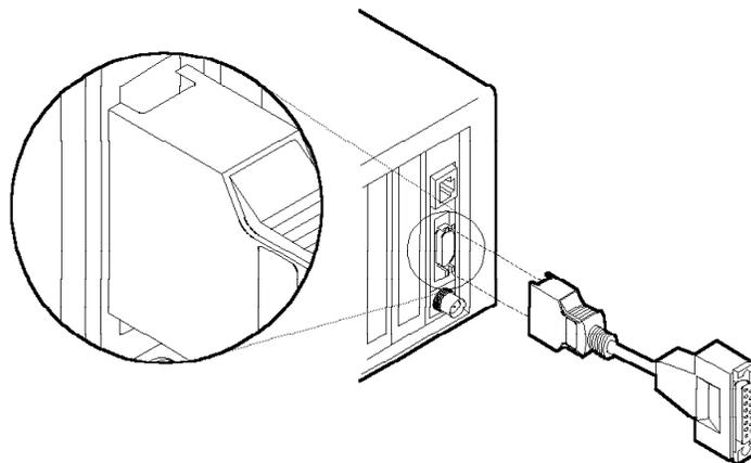
Connect the other end of the Mini AUI-to-AUI adapter cable to the AUI drop cable connected to the network.
