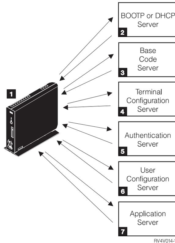
Figure 1. Network Station Power-On Sequence
