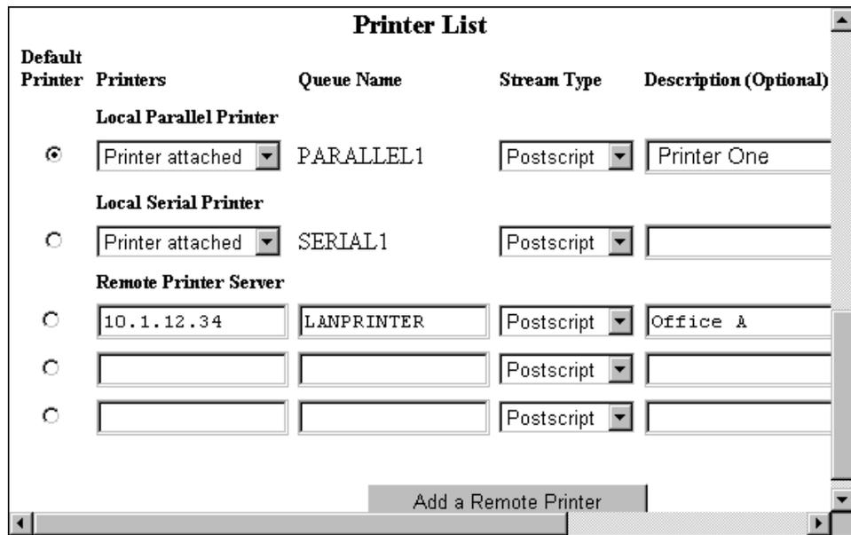
Figure 45. Configuring a LAN-attached Printer
