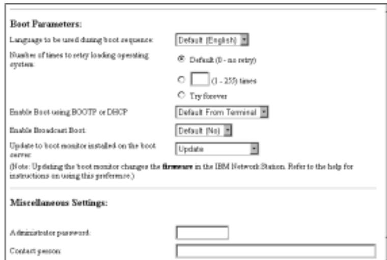
Figure 44. Overriding the Network Station Boot Setting
