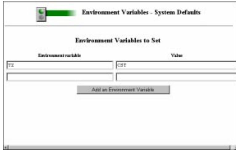
Figure 50. Setting the Time Zone (TZ) Environment Variable
