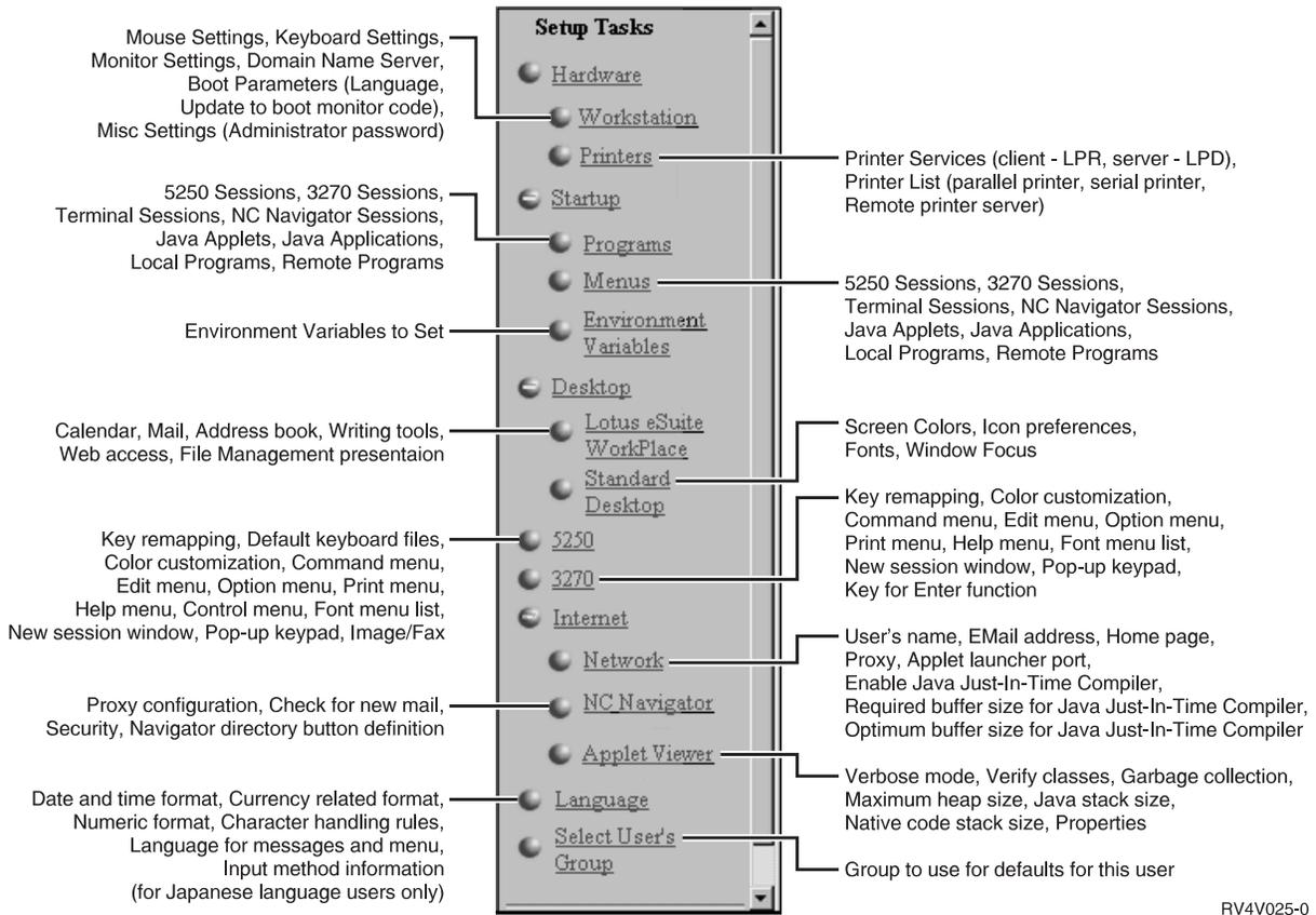
Figure 29. Setup Tasks Supported by the IBM Network Station Manager Program
