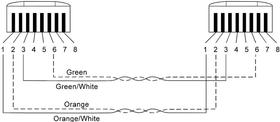
Figure A-2. Straight-Through UTP Cable (RJ-45 to RJ-45), T568-B
