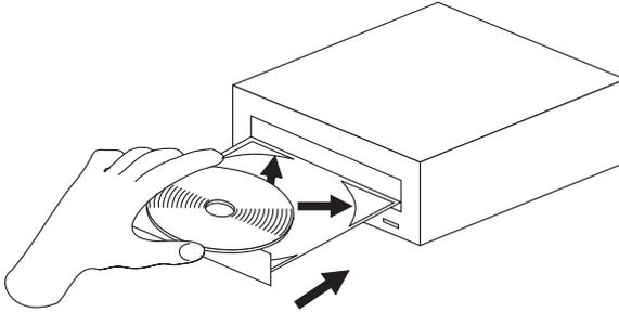
1. Press the Eject/Load button. The tray slides out of the drive.
