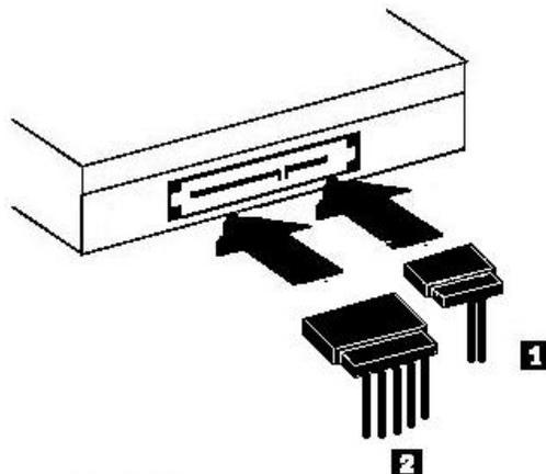
1. Attach a 7-pin Serial ATA data cable connector **1** to the Serial connector on the drive.
