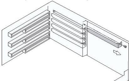
5. Make sure that you remove the antenna from the card, and gently insert the connector of the PCI card into the slot.
