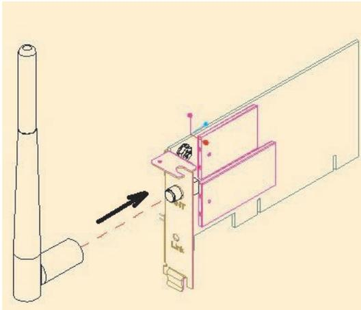
3. Install the antenna by threading it clockwise until it is firmly seated. Do not overtighten.
