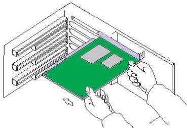
6. Secure the card into place with the screw that you removed in step 4.
