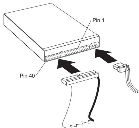
The cable connector is keyed and fits only one way. Be sure that the cables will not be pinched or crowded by the computer cover and that all other cable and power connections are secure.
