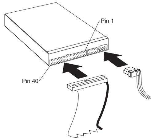
3. Find an unused power connector on a cable coming from the computer power supply and attach it to the four-pin DC power connector. The power connector is keyed so that it attaches one way only. Do not force it. If the connector does not attach using reasonable pressure, recheck the orientation of the cable connector to the drive connector, and try again.
