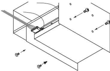
(If the drive is held in place securely by rails, you will not need to use the mounting screws.)
