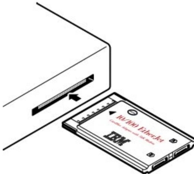
Figure 1-1. Inserting the CardBus Adapter into the Computer
