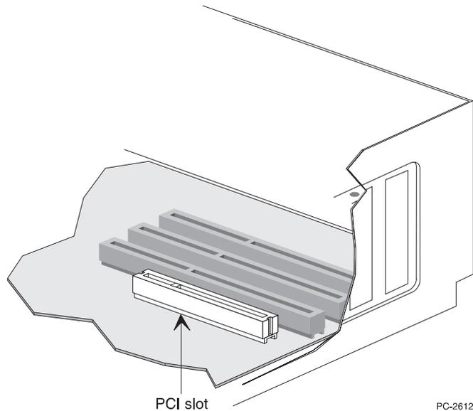
Figure 1-5. PCI Slot Illustration
