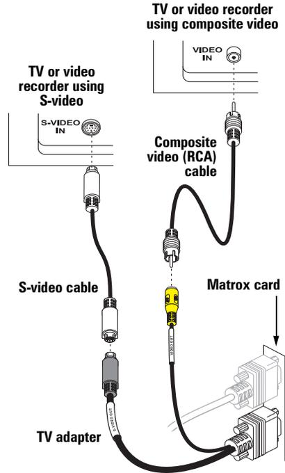
(Note: Using the Matrox composite video and S-video connectors at the same time is optional.)
