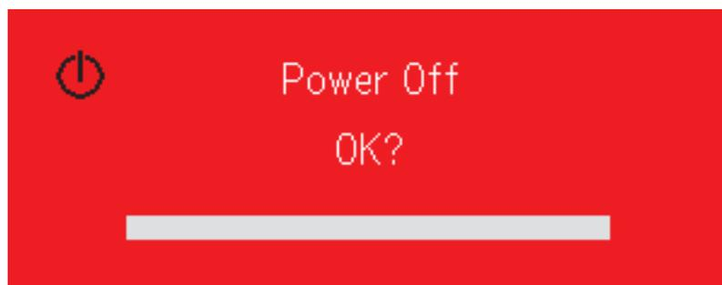
**Note:** Leave the power cable plugged in for at least 2-5 minutes until the projector returns to room temperature before placing the projector inside the soft case. Placing the projector into the case too soon after switching off the power could cause the projector to overheat.
