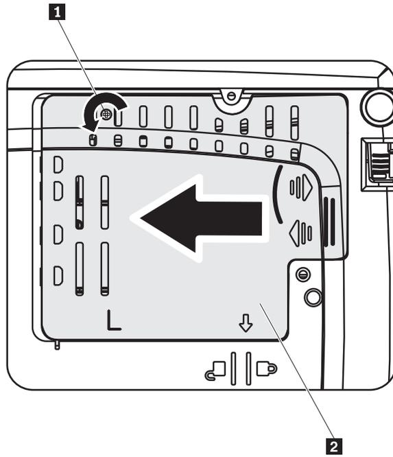
4. Remove the two screws from the lamp module as shown in **3**.
