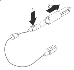
2. Plug the smaller end of the DC power cord here (see the illustration below). The DC power cord is fully inserted when a click is heard.
