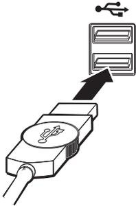
Attach the keyboard cable to the USB port as shown above.
