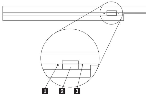
**1** Power light: This light is visible when the drive is in use.
