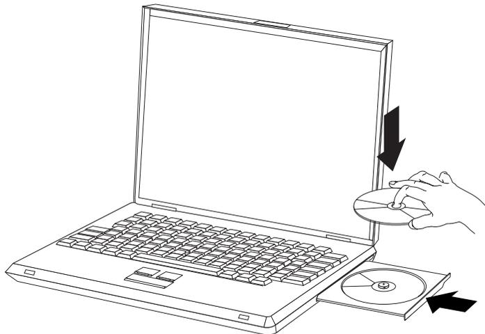
1. Press the Eject button. The tray slides out of the drive.
