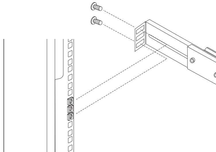
10. Tighten the two rail-adjustment screws on each of the outer rails that you loosened in step 7 on page 22.
