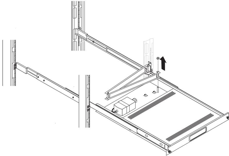
6. Route the video, power, and keyboard-and-mouse cables along the new cable-management arm and secure them along the way with cable straps.
