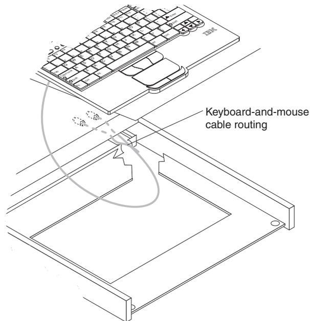
8. Secure the keyboard-and-mouse cable to the cable-management arm using the existing cable straps.
