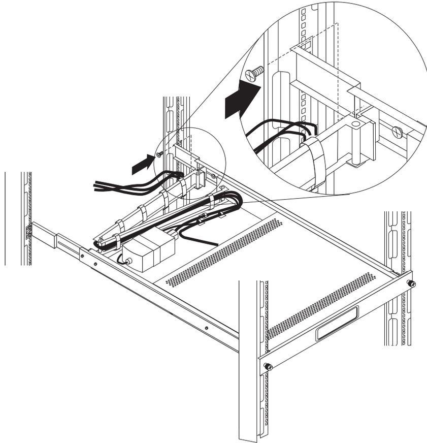
17. Connect the video, keyboard, and mouse connectors to either a server or a console switch in the rack cabinet. Connect the power cord to the short jumper cord on the cable-management arm; then, connect the power cord to a properly grounded electrical outlet or power distribution unit (PDU).
