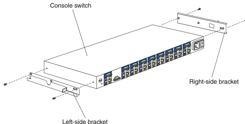
2. Install the console switch behind the flat-panel monitor and keyboard tray using two screws from the miscellaneous hardware kit.
