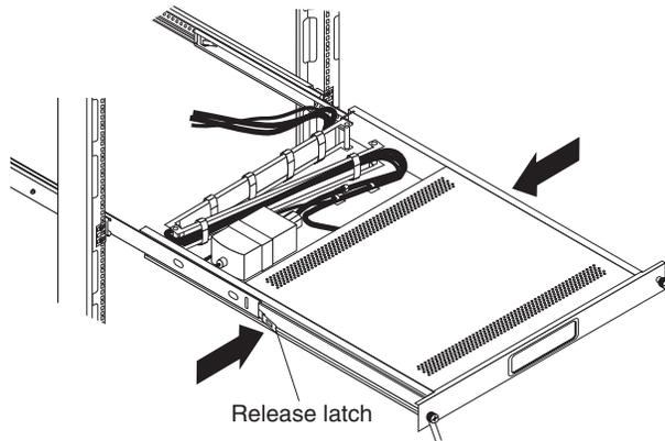
15. Push the tray in the rack; then, tighten the four rear slide-rail bracket screws.
