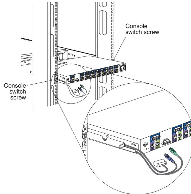
3. Route the power, video, and keyboard-and-mouse cables through the channel in the left-side bracket on the console switch; then, connect the video, keyboard, and mouse connectors to the console switch.
