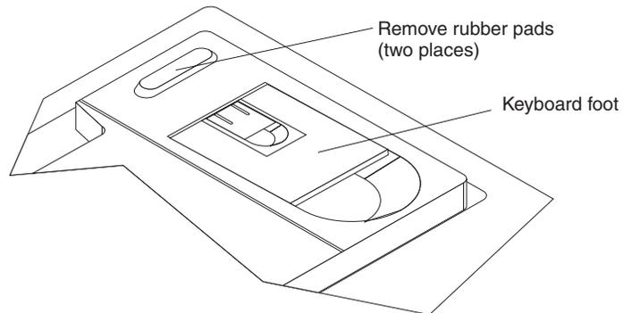
**Attention:** Do not extend the keyboard feet. The flat-panel monitor screen might be damaged if the feet are extended when the monitor is closed.
