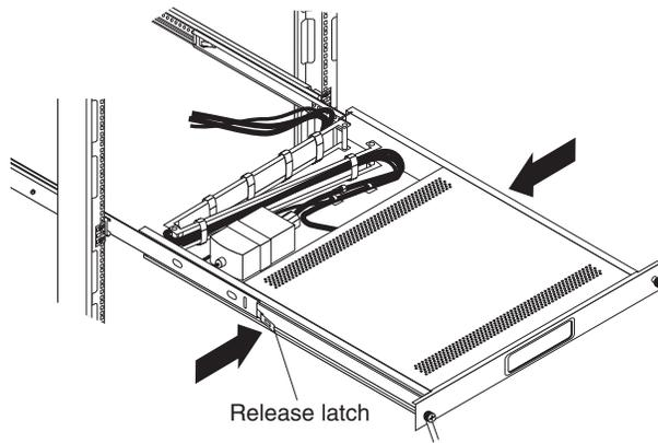
6. Remove the eight screws that attach the outer slide rails to the rack cabinet; then, remove the old outer slide rails from the cabinet.
