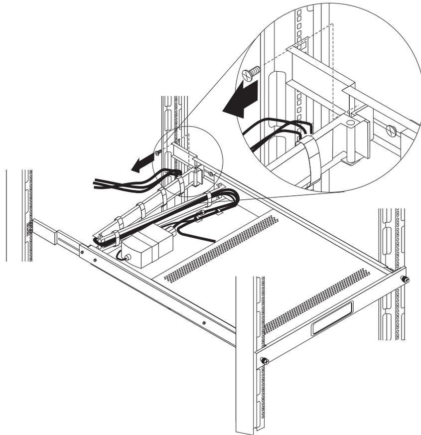
5. Fully extend the monitor and keyboard tray from the front of the rack cabinet; then, push in the release latch on each side of the tray and slide the monitor
