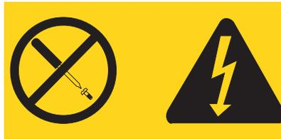
Hazardous voltage, current, and energy levels are present inside any component that has this label attached. There are no serviceable parts inside these components. If you suspect a problem with one of these parts, contact a service technician.
