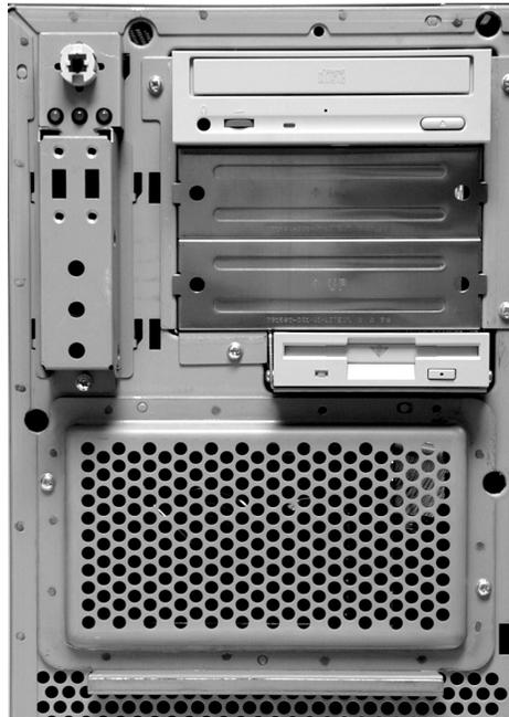
4. Slide the hard disk drive cage from the chassis.
