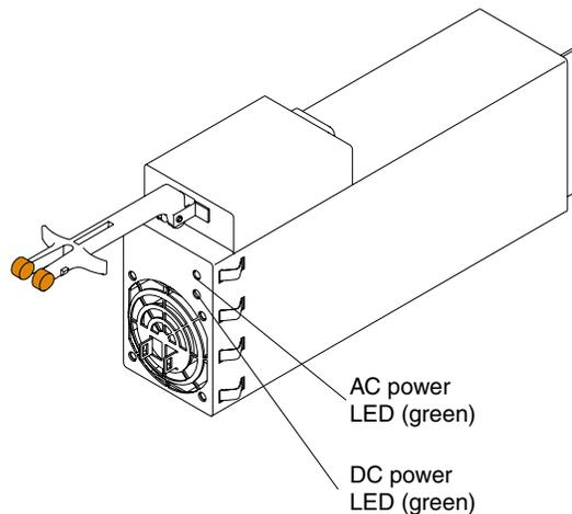
**AC power light:** This green light on the power supply (behind the bezel) provides status information about the power supply. During normal operation, both the ac and dc power lights are on. For any other combination of lights, see “Power-supply LEDs” on page 103.
