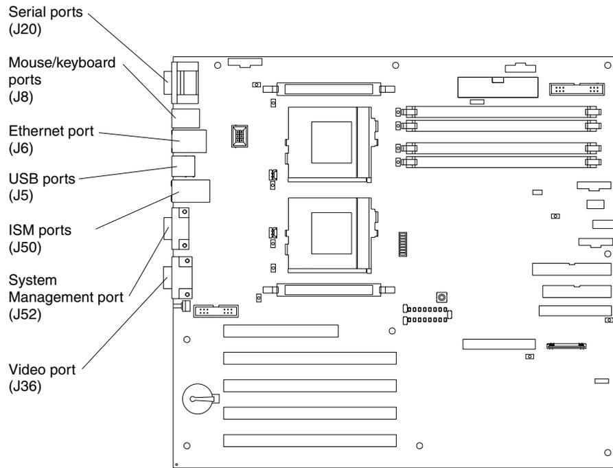
Future releases of the Integrated System Management (ISM) firmware code will enable the Integrated System Management processor to send or forward alerts to IBM system management adapters using the ISM ports.
