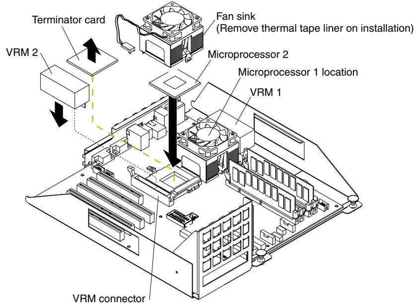
6. Store the terminator card in a safe place in the static-protective package that your new microprocessor comes in; you will need to install it again, if you ever remove the microprocessor and do not replace it.
