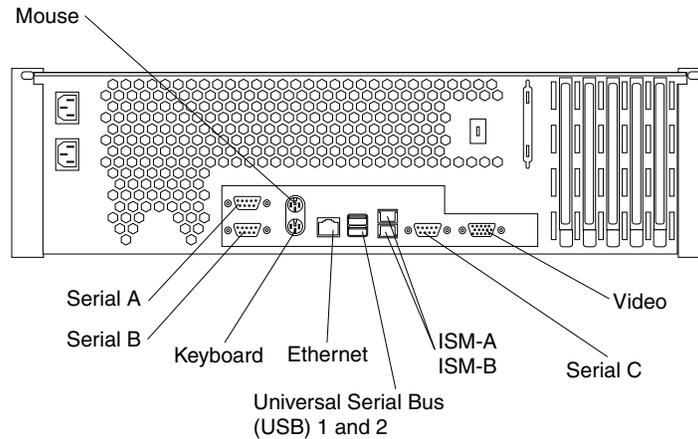
Future releases of the Integrated System Management (ISM) firmware code will enable the Integrated System Management processor to send or forward alerts to IBM system management adapters using the ISM ports. Future releases of the Integrated System Management (ISM) firmware code will enable the Integrated System Management processor to send or communicate using a modem and this dedicated serial port.
