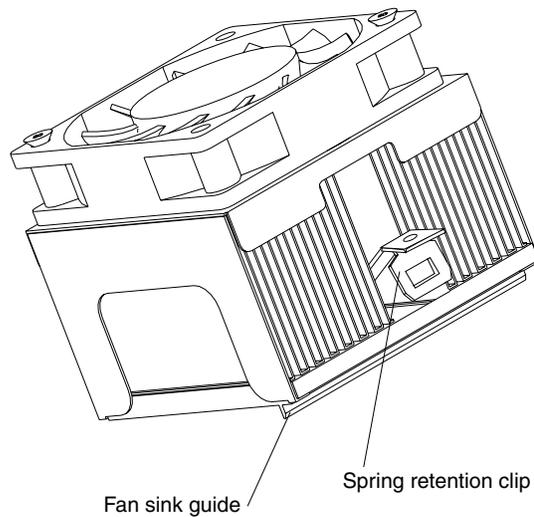
11. Press down and latch the spring retention clip on the back of the fan sink (the side facing the back of the server).
