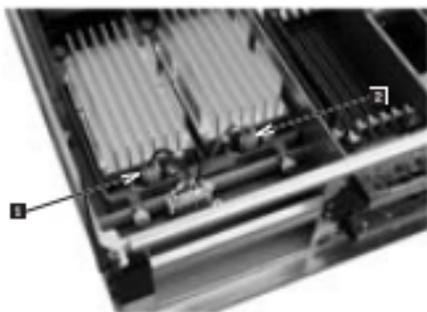
6. If you are removing a thermal blank, skip this step. Otherwise, remove the Y cable to the power pods by releasing the connectors (1 and 2).
