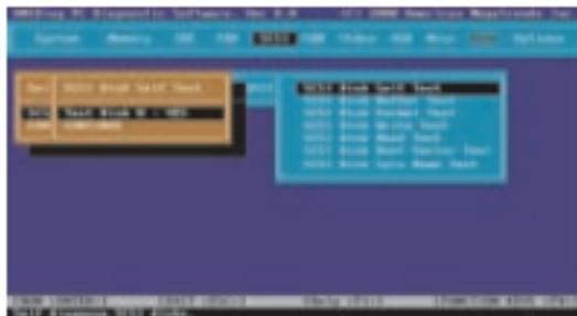
To run the test, select SCSI Disk Self Diagnostic Test and press <Enter>. Choose the parameters on the screen and choose Continue. The SCSI Disk Self diagnostics test cannot be aborted. You must wait until the entire disk self test completes.
