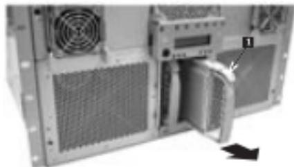
4. Remove each hard disk drive from the drive bay by first grasping its handle and depressing the drive locking tab (1), and then sliding the drive out of the bay.
