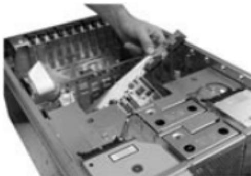
16. Grasp the T-Docking board by the right-rear edge and lift up to remove it from the chassis.
