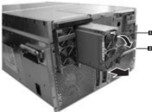
2. Push the thumb latch (1) to unlock the power supply handle and pull the handle (2) down to undock the supply.
