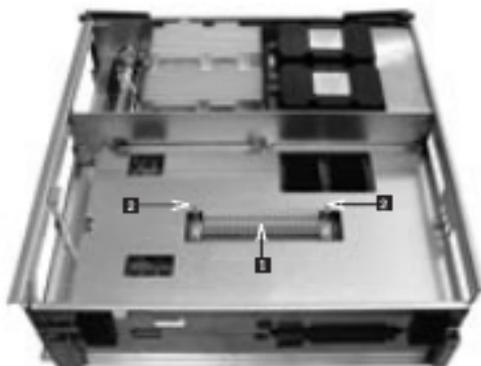
2. While holding the extraction levers in the raised position, place the memory board over the Processor Baseboard connector (1) and guide pins (2). The extraction levers must be raised so that they can engage the guide pins.
