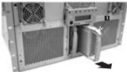
3. Push on the drive carrier latch (1) of the failed drive and use the handle to pull the assembly toward you.
