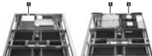
Each processor ( **1** ) has its associated power pod ( **2** ). Processors and power pods should only be removed or installed in pairs. Be sure that you install a thermal blank ( **3** ) if you intend to leave removed any processor/power pod pair.
