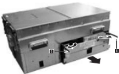
8. Rotate the two extraction levers ( 8 ) on the sides of the module to eject it from the Sideplane connector.
