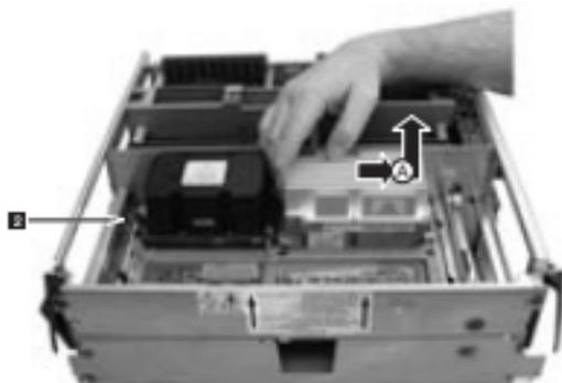
9. To remove the power pod associated with the processor, pull the power pod back ( **A** ) to disengage it from its connector. Then, lift the power pod out of the system. If you are only removing a power pod, stop here. To install a power pod, start with Step 6, and continue through Step 10 on page 184.
