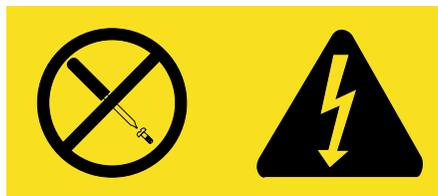
**Hazardous voltage, current, and energy levels are present inside any component that has this label attached. There are no serviceable parts inside these**
