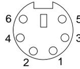
Table 7. Keyboard-connector (6-pin female) pin-number assignments .
