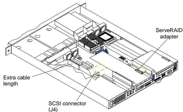
10. Replace the cover on the server; then, reinstall the server in the rack and connect all external cables. For more information, see “Installing the cover” on page 49 for instructions.
