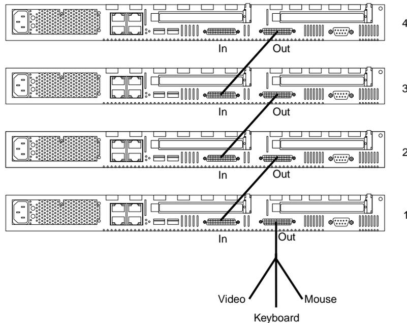
**Note:** Server 1 (usually the server at the bottom of the rack) is the server to which you connect the device breakout cable.
