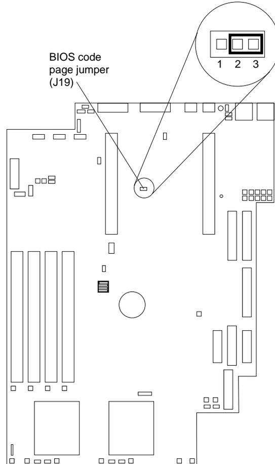
3. Move the jumper from pins 2 and 3 to pins 1 and 2 to enable BIOS back page.
