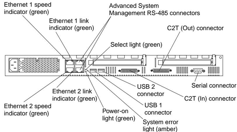
The ASM connectors on the back of the server are referred to in this book as RS-485 (A) and RS-485 (B).
