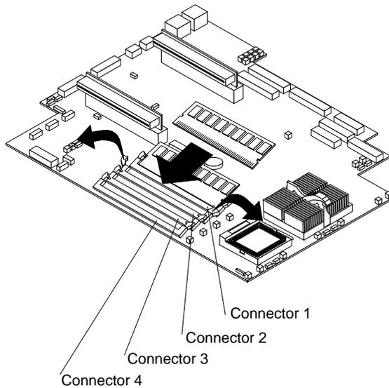
Complete the following steps to install a DIMM:
