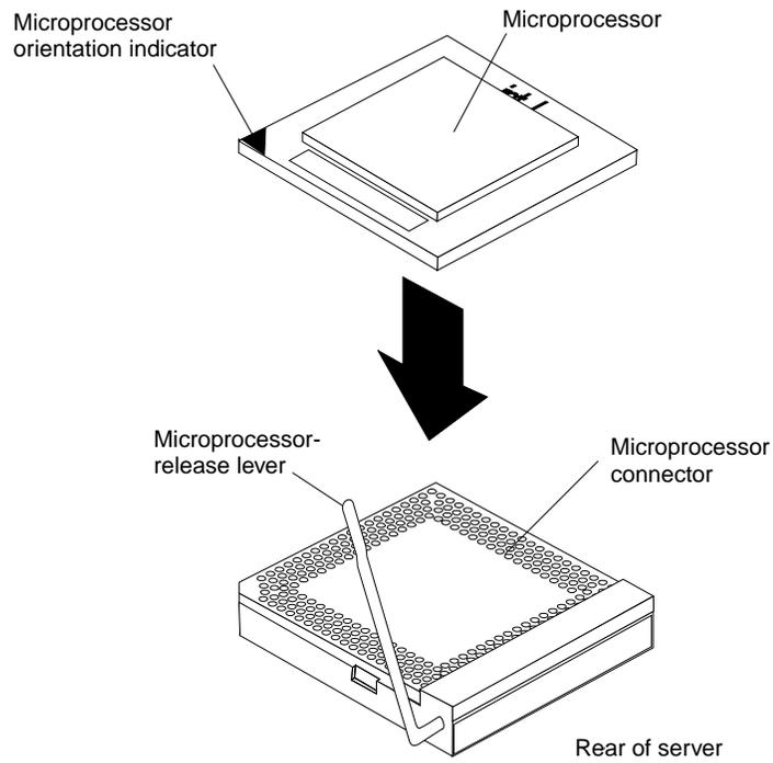
7. Push the microprocessor-release lever down to lock the microprocessor in place.
