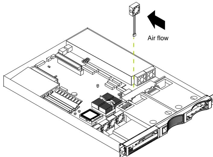
8. Connect the fan cable to the system board.
