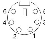
Table 9. Auxiliary or pointing-device-connector (6 pin female) pin-number assignments .
