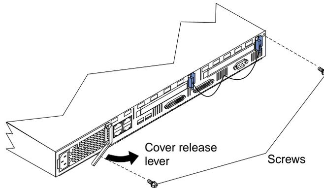
**Note:** You might need to remove the clear plastic shield to reach some parts in the server. For proper cooling and airflow, replace the clear plastic shield before replacing the cover.
