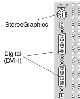
Note that the Wildcat III 6110 adapter occupies the AGP slot and the adjacent PCI slot.
