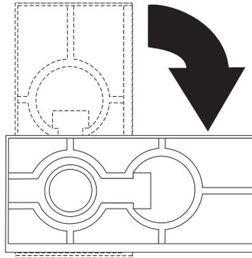
When you are finished and have reinstalled the side cover, turn the two front stabilizing feet a quarter turn outward and set the computer carefully back on its feet.
