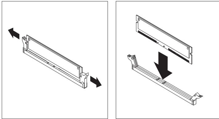
7. Insert the RIMM into the connector by aligning the RIMM edges with the slots at each end of the RIMM connector. Firmly press the RIMM straight down into the connector by applying pressure on both ends of the RIMM simultaneously. The retaining clips snap into the locked position when the RIMM is firmly seated in the connector.
