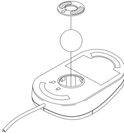
4. Turn the mouse right-side up, and the retainer and ball will drop out.
