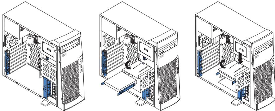
**Note:** Clear any cables that might impede the replacement of the drive cage.
