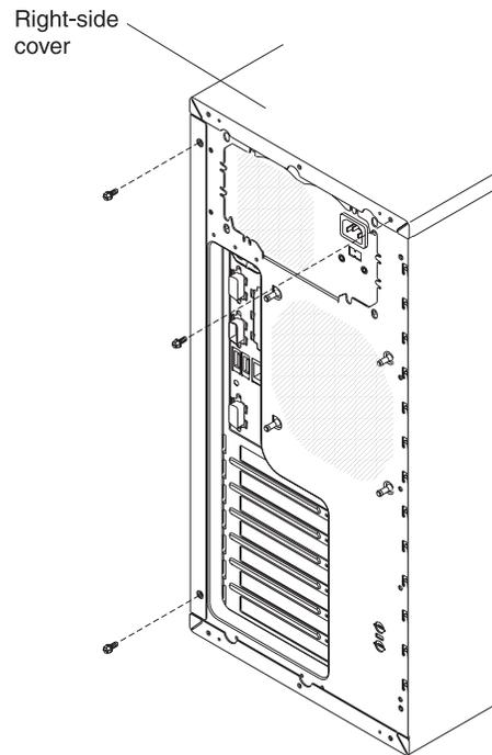
*Figure 7. Removing the right-side cover*
