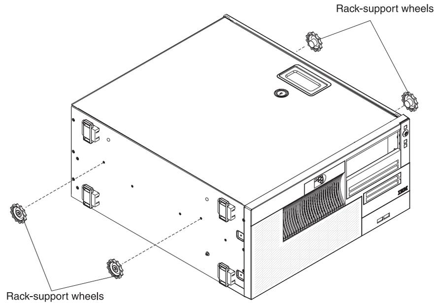
*Figure 15. Attaching the rack-support wheels*
