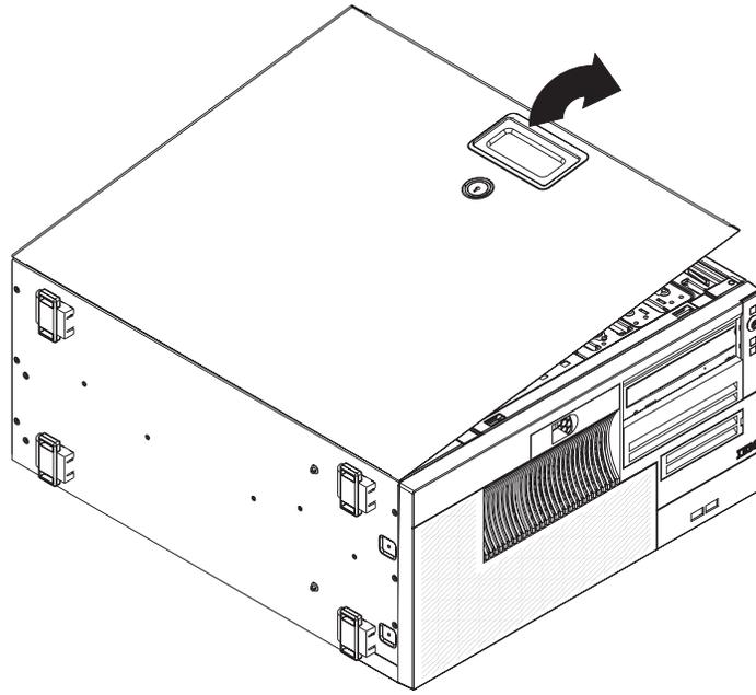
*Figure 13. Installing the top cover*
