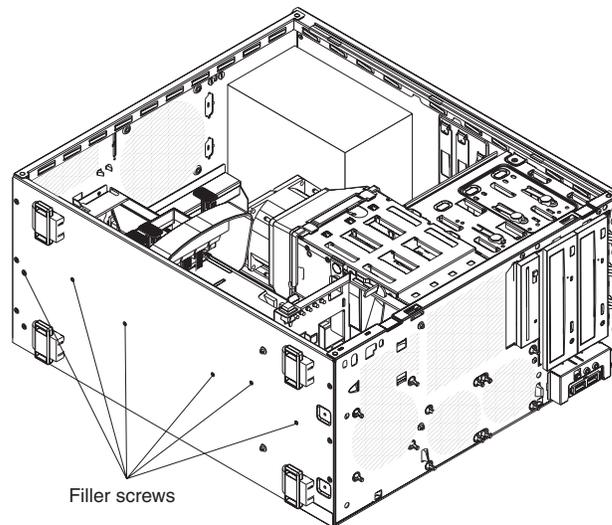
Figure 6. Removing the six screws from the bottom of the system
