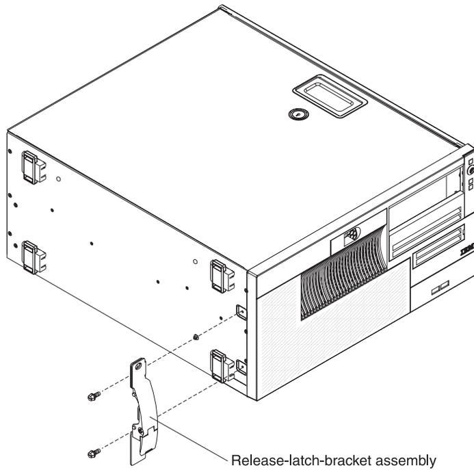
*Figure 14. Installing the release-latch-bracket assemblies*
