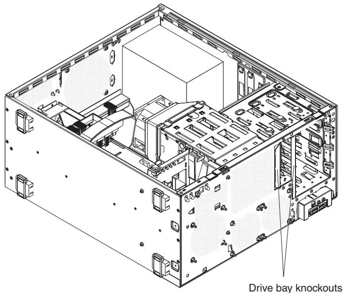
Figure 9. Reinstalling the removable-media drives and hard disk drive to a rack orientation
