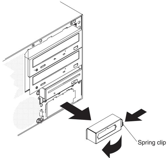
*Figure 8. Removing the front USB housing*
