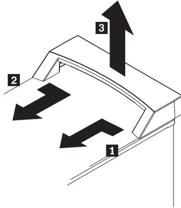
Figure 5. Removing the top handle
