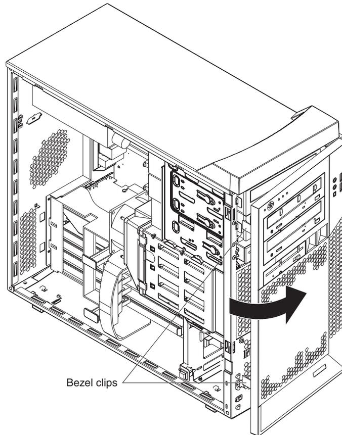
*Figure 4. Removing the one-piece bezel*
