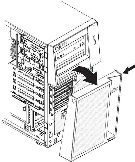
*Figure 2. Removing the lower bezel*
