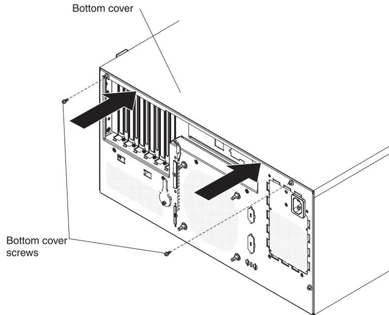
Figure 10. Installing the new bottom cover
