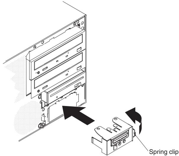
*Figure 11. Reconnect the front USB housing*
