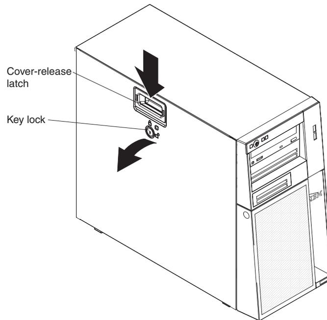
*Figure 1. Removing the left-side cover*
