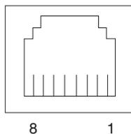
Connect a Category 3, 4, or 5 unshielded twisted-pair cable to this connector. The 100BASE-TX and 1000BASE-T Fast Ethernet standards require Category 5 or higher cabling.
