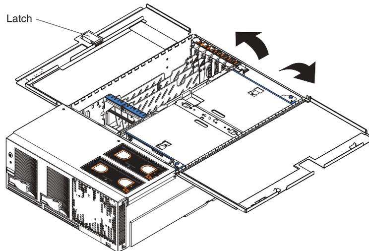
3. Pull the release latch on the left side of the top cover to the right.
