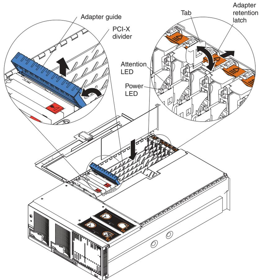
4. Follow the cabling instructions, if any, that come with the adapter. Route the adapter cables before you install the adapter.
