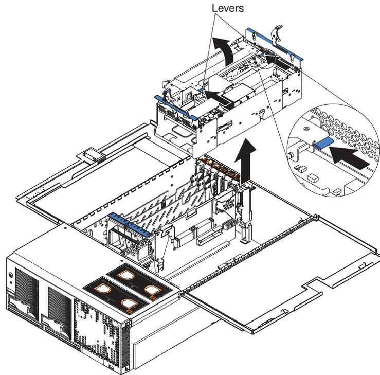
7. Install the microprocessor and power module:
