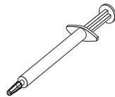
**Note:** 0.01mL is one tick mark on the syringe. If the grease is properly applied, approximately half (0.02 mL) of the grease will remain in the syringe.
