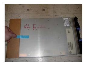
1.3- Place the Blade in ESD bag 37L8109, as shown below, and seal it closed using ESD label 6937292.
