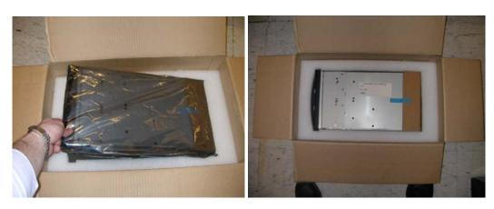
1.7- Remaining Urethane Cushion 22K8229 is placed on top of Blade. Top U-Tray 22K8231 is set on top of Cushion.
