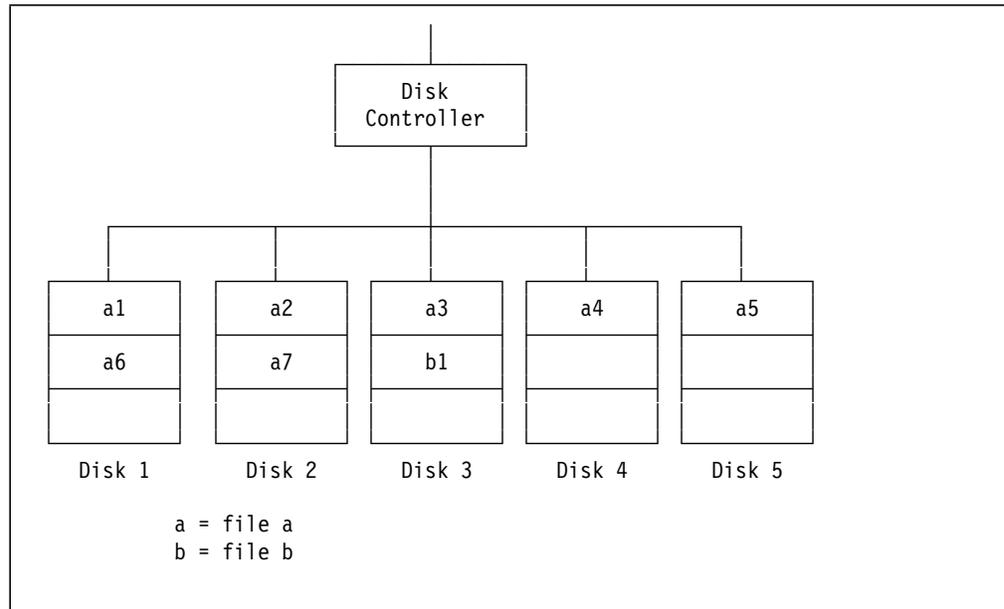
Figure 22. RAID-0 (Block Interleave Data Striping without Parity)
