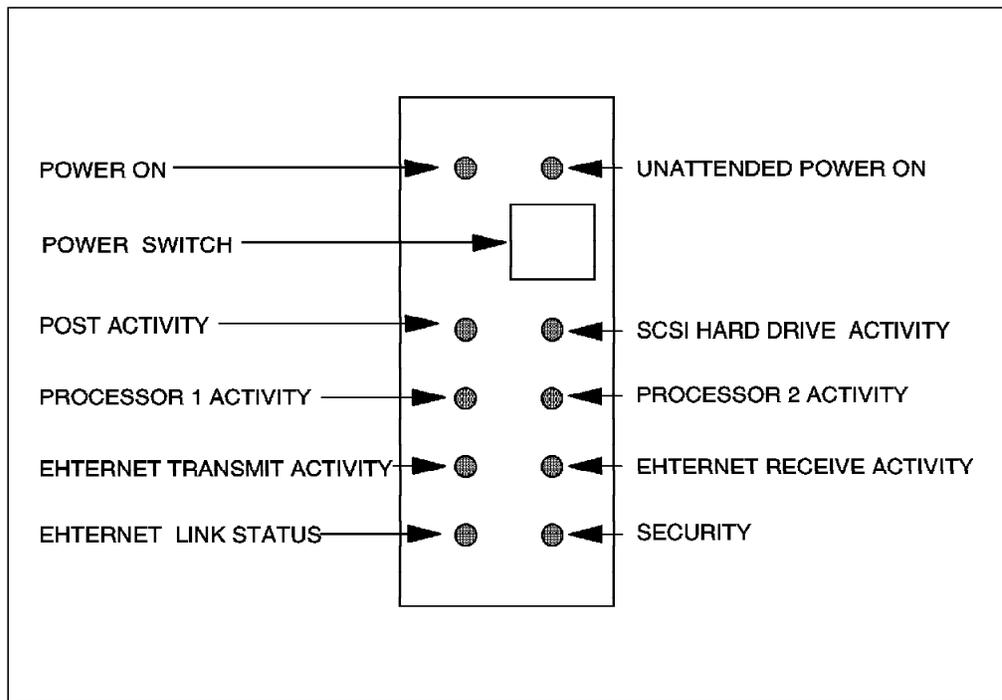
Figure 45. View of the IBM PC Server 300 Operator Panel
