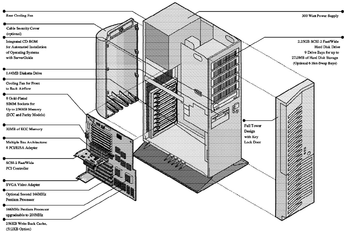
Figure 36. Covers Off Front and Side Views of the PC Server 320
