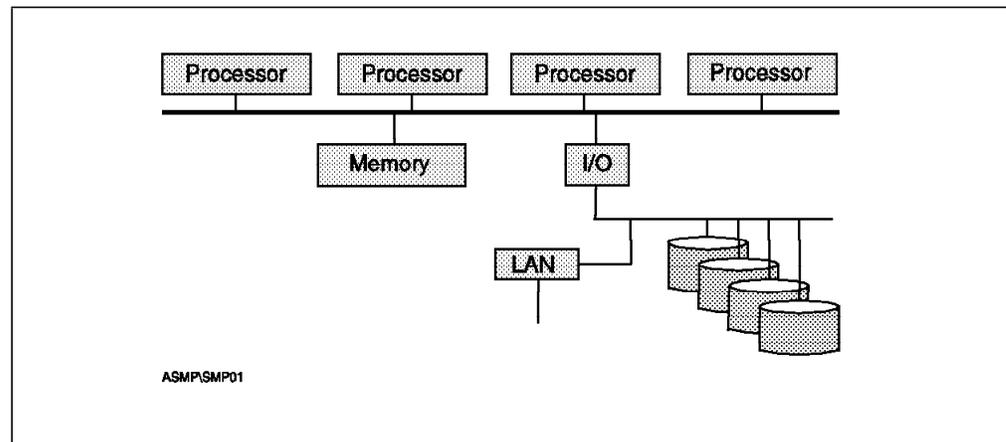
Figure 5. A Typical SMP Configuration
