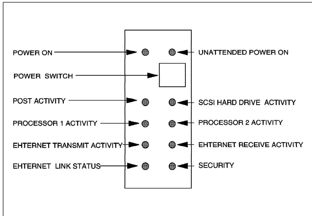
Figure 42. IBM PC Server 325 Operator Panel
