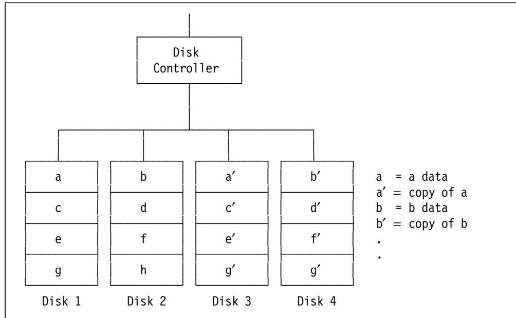
Figure 25. RAID-10 - Mirroring of RAID-0 Drives
