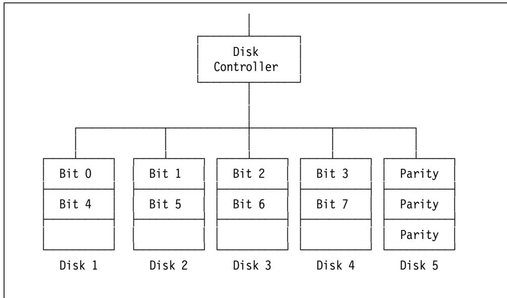
Figure 27. RAID-3 (Bit Interleave Data Striping with Parity Disk)
