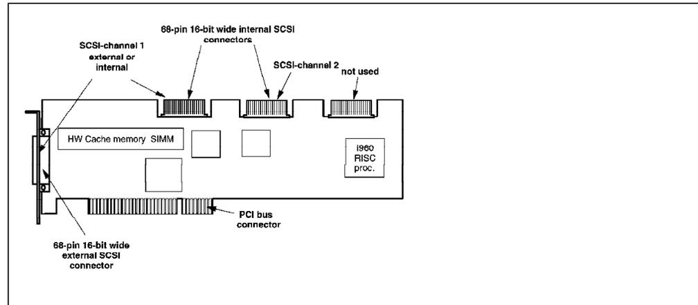
Figure 54. PCI SCSI-2 Fast/Wide Adapter
