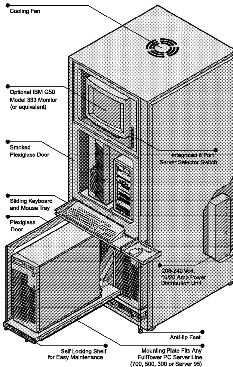
Figure 59. Exploded View of the IBM 9306 PC Server Rack Enclosure
