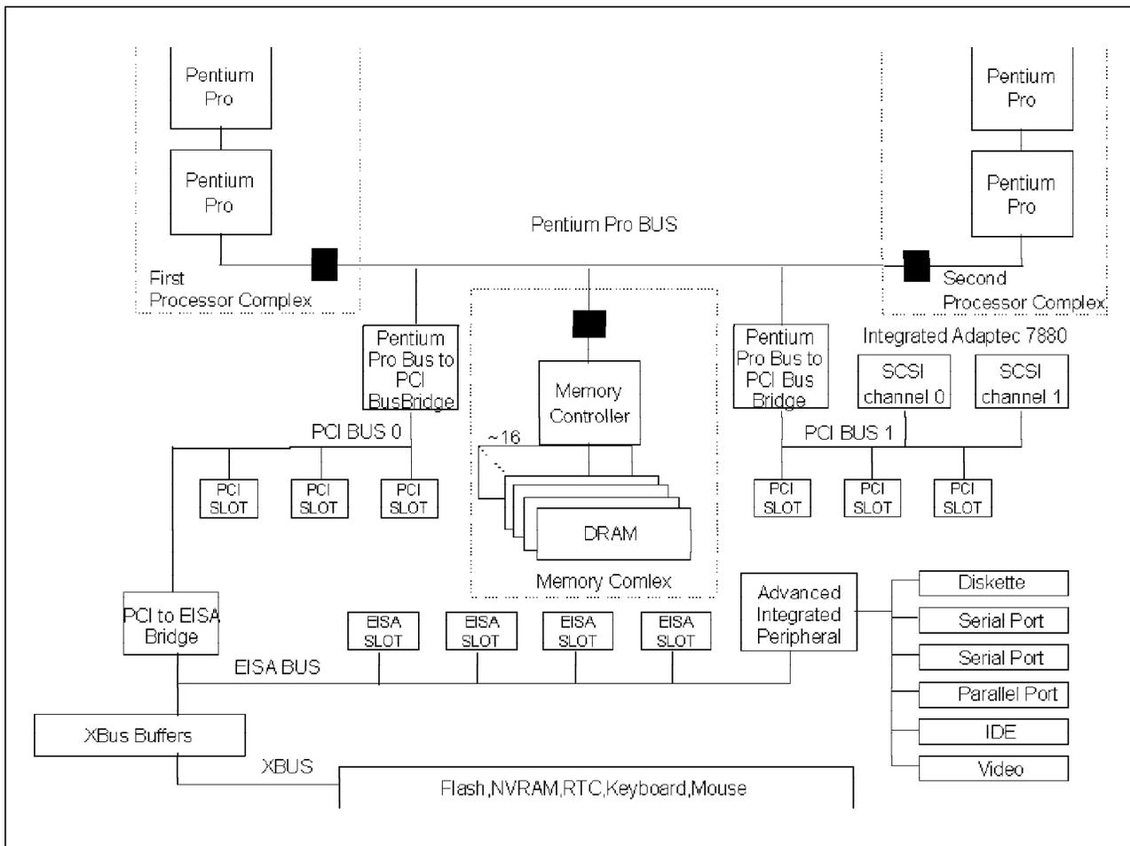
Figure 8. PCI Configuration in the PC Server 704
