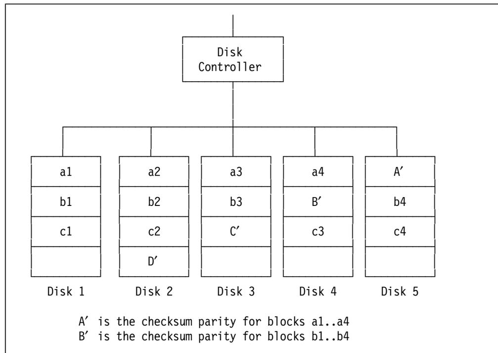
Figure 29. RAID-5 (Block Interleave Data Striping with Skewed Parity)
