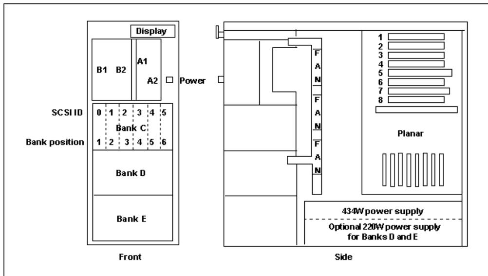
Figure 47. Side View of Server 520. This diagram shows the layout of the bays in the Server 520 system unit and the layout of the adapter slots on the planar board. Note there are four fans to provide sufficient circulation of air throughout the complex, three as shown and one in the power supply.
