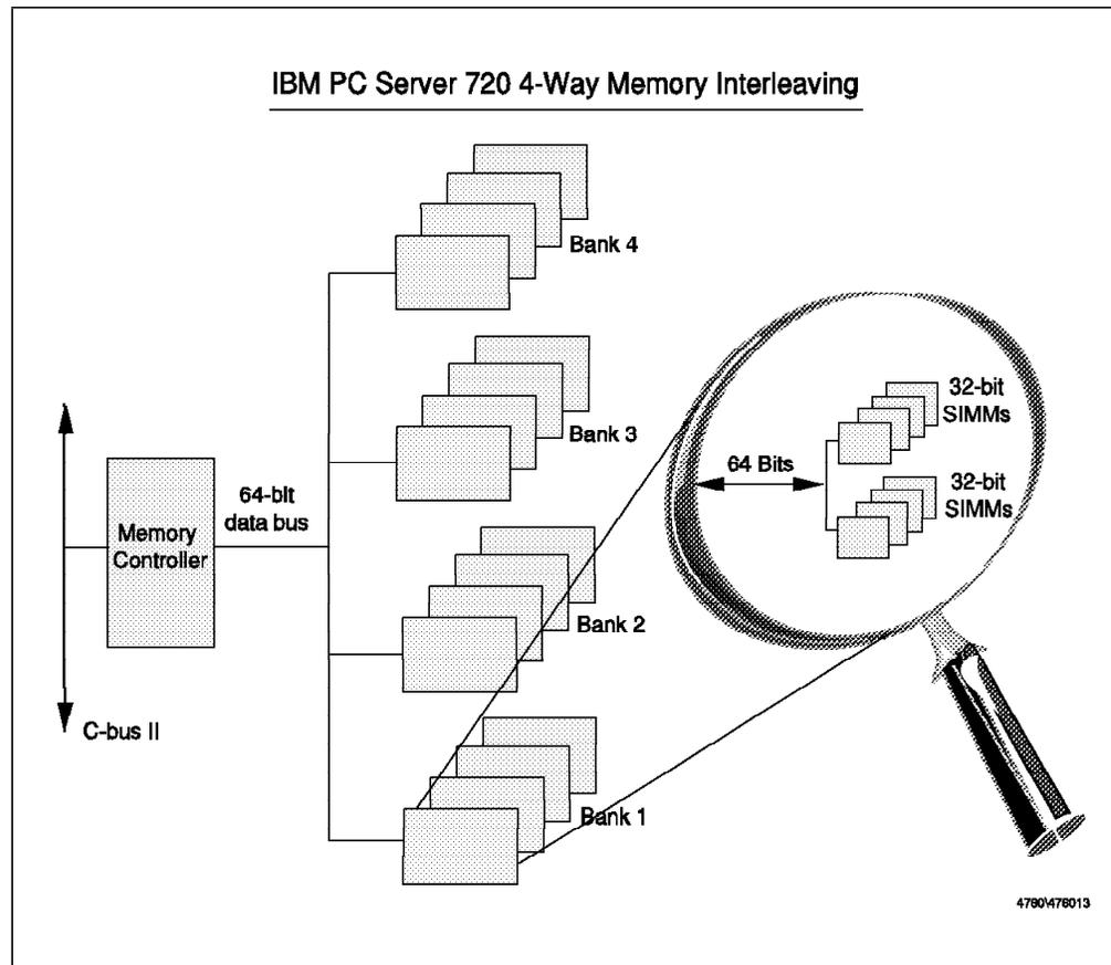
Figure 15. Four-way Interleaving in the IBM PC Server 720
