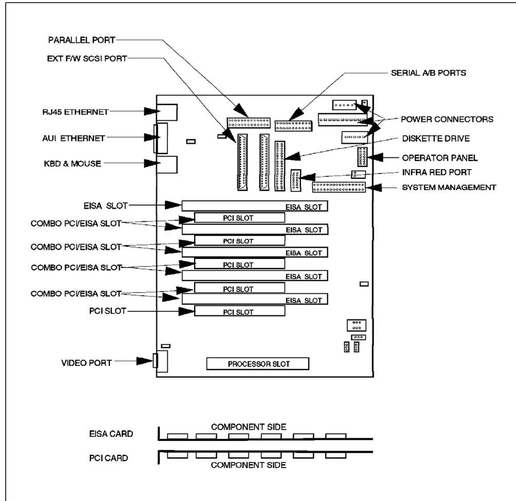
Figure 40. IBM PC Server 325 System Board
