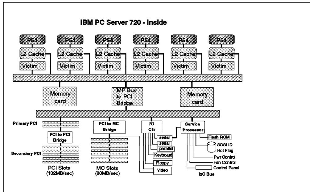
Figure 50. The Architecture of the IBM PC Server 720
