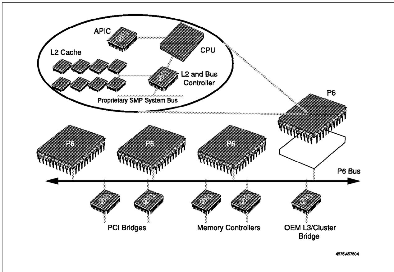
Figure 2. The Pentium Pro in a Four-Way SMP Configuration
