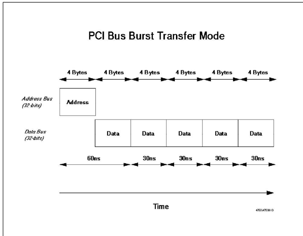
Figure 6. PCI Bus Burst Transfer at 33Mhz
