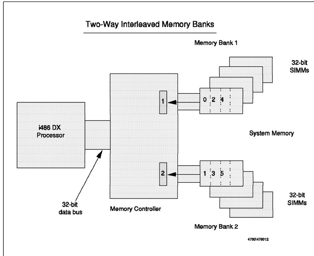
Figure 14. i486-based Two-Way Interleaved Memory System
