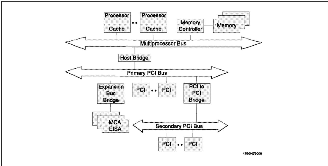
Figure 9. PCI Configuration in the PC Server 720
