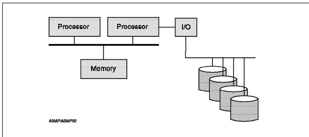
Figure 4. Asymmetric Multiprocessing Example 2. This configuration has one processor doing all I/O.
