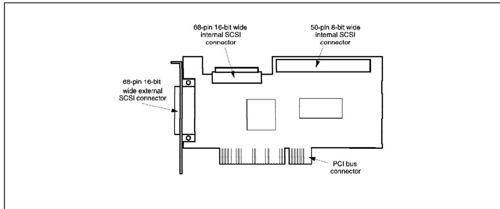
Figure 53. PCI SCSI-2 Fast/Wide Adapter
