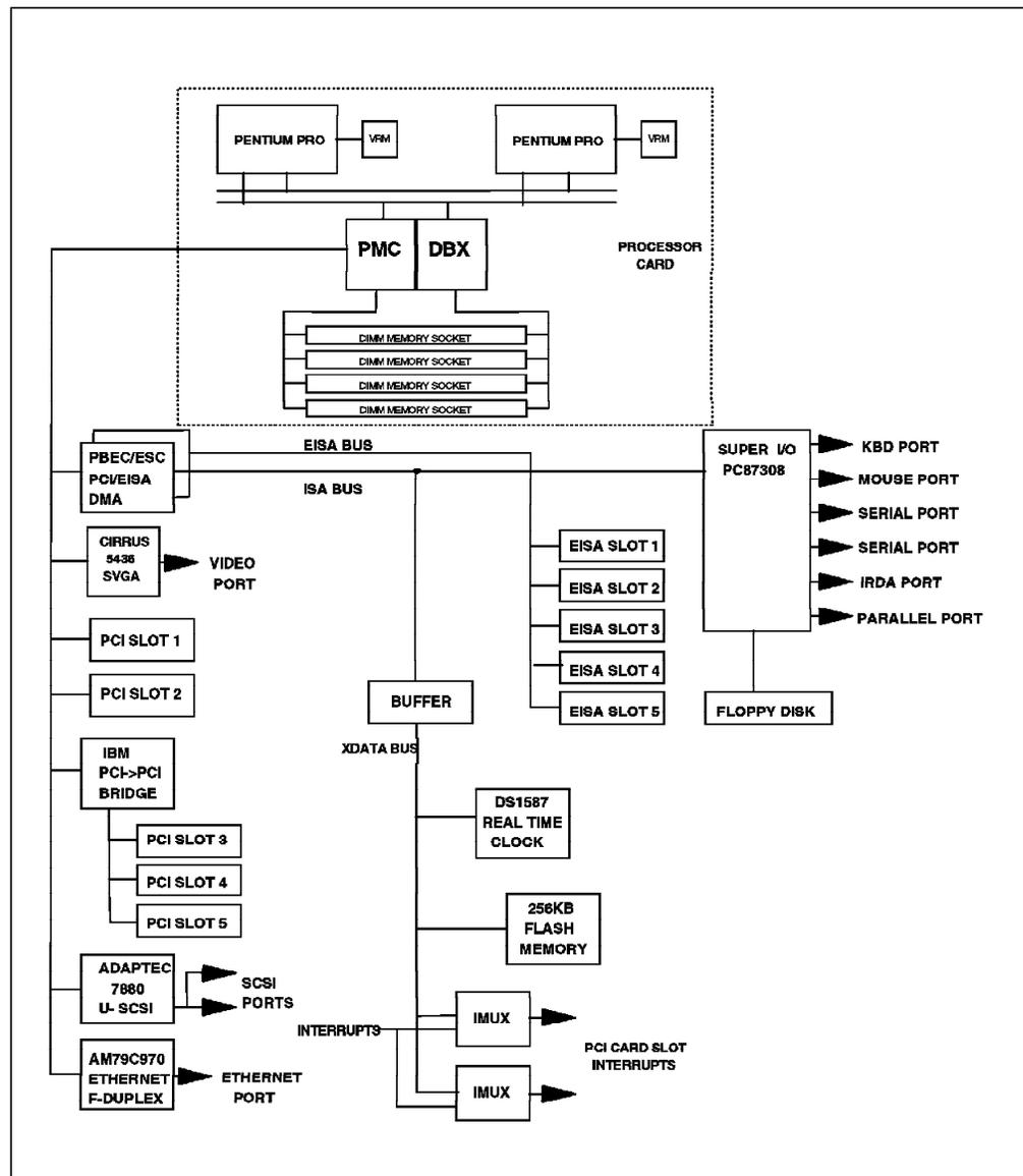
Figure 39. IBM PC Server 325 System Architecture
