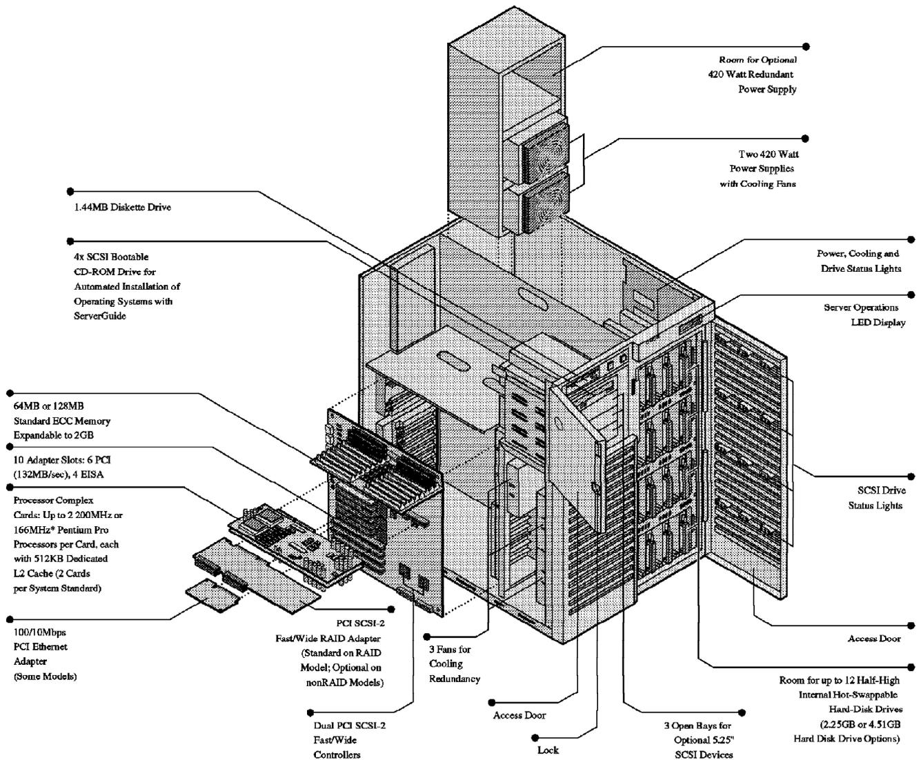
Figure 48. Exploded View of the Server 704 200 MHz
