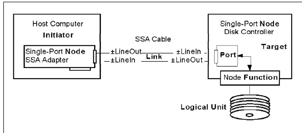
Figure 18. SSA Link - a Closer View
