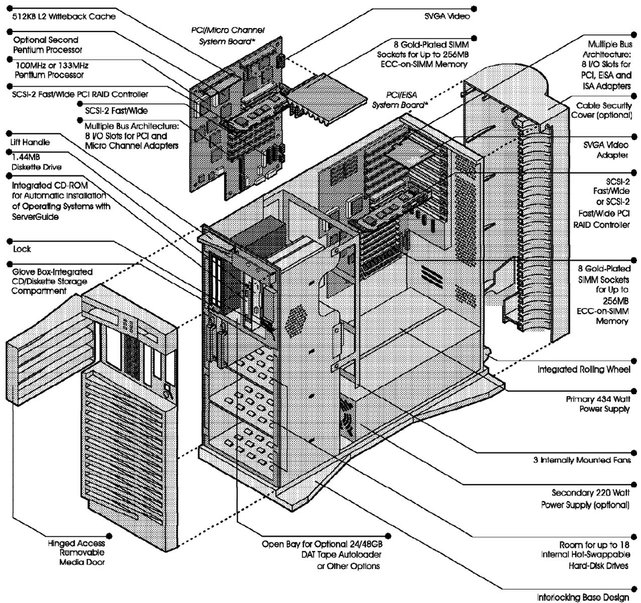
Figure 46. Exploded View of the IBM PC Server 520. The PC Server 520 ships with either a PCI/EISA or PCI/MCA system board.
