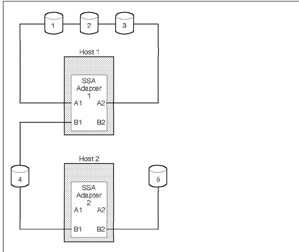
Figure 20. An Example of an SSA Loop and an SSA String. Disks 1, 2 and 3 form a loop with Host 1; Disk 5 forms a string with Host 2; Disk 4 forms a string with both Host 1 and 2 providing multi-host access to its data.
