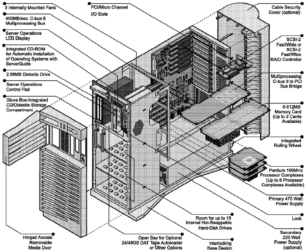
Figure 49. Exploded View of the IBM PC Server 720
