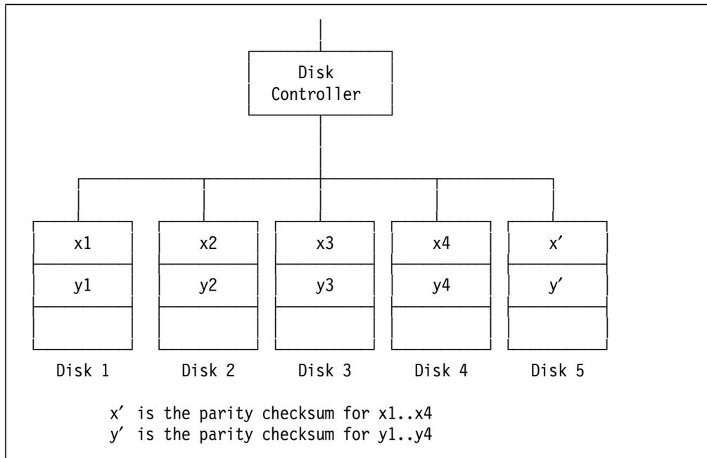
Figure 28. RAID-4 (Block Interleave Data Striping with One Parity Disk)
