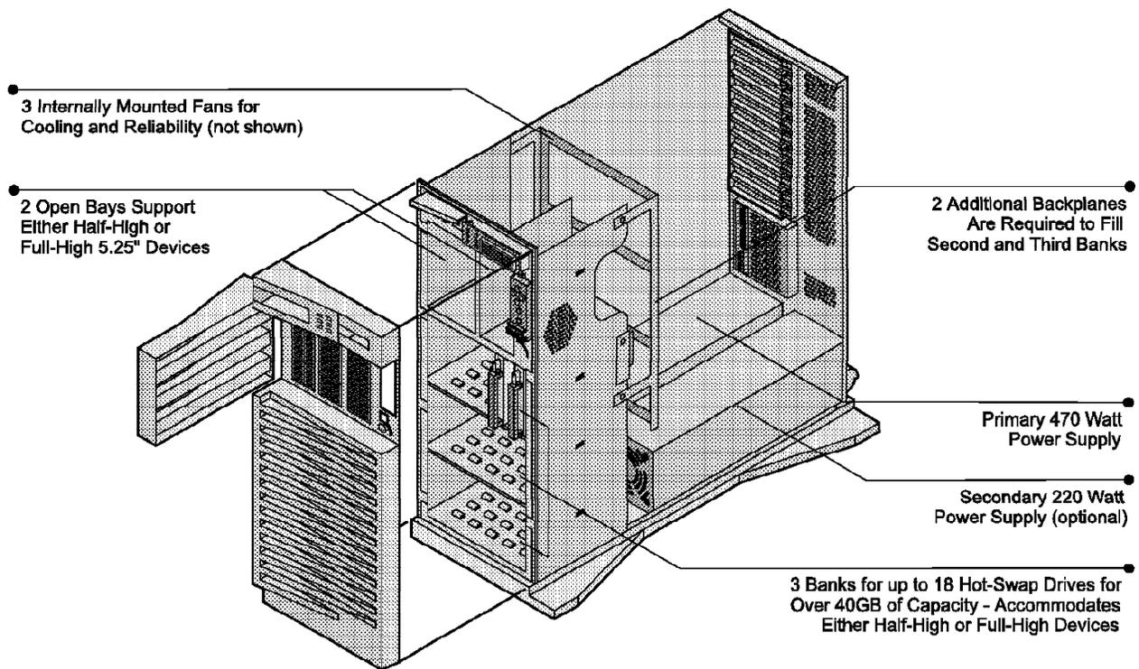
Figure 61. Exploded View of the IBM 3518 PC Server Enterprise Expansion Enclosure
