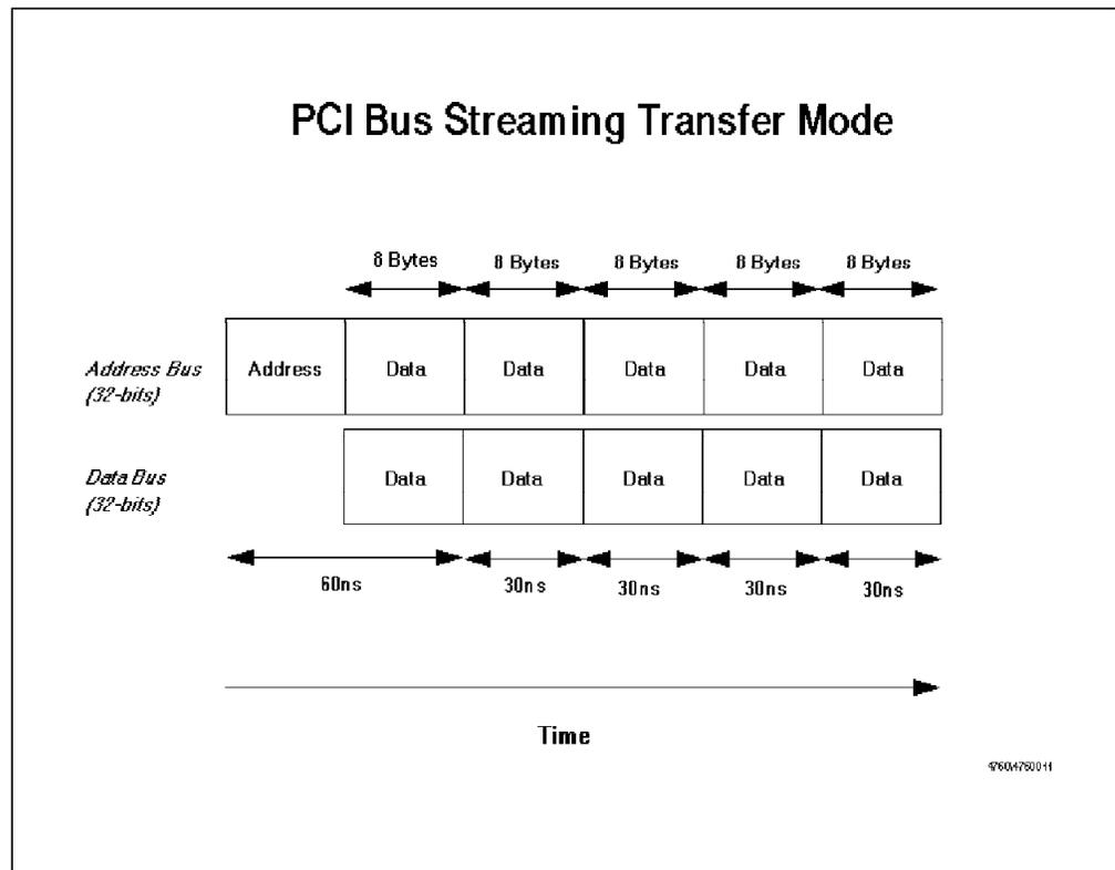
Figure 7. PCI Bus Streaming Mode at 33 Mhz
