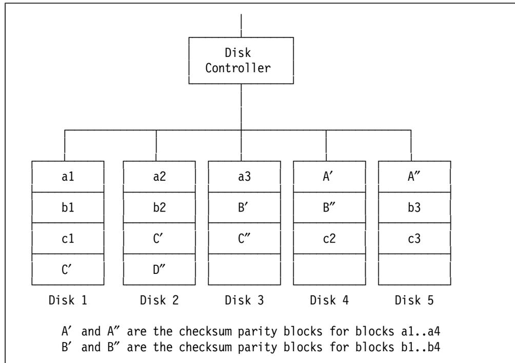
Figure 30. RAID-6 (Block Interleave Striping with Double Skewed Parity)
