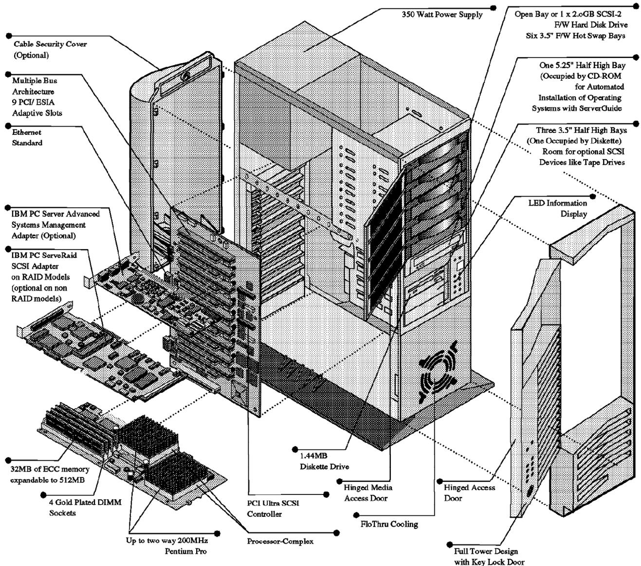
Figure 43. Exploded View of the IBM PC Server 330
