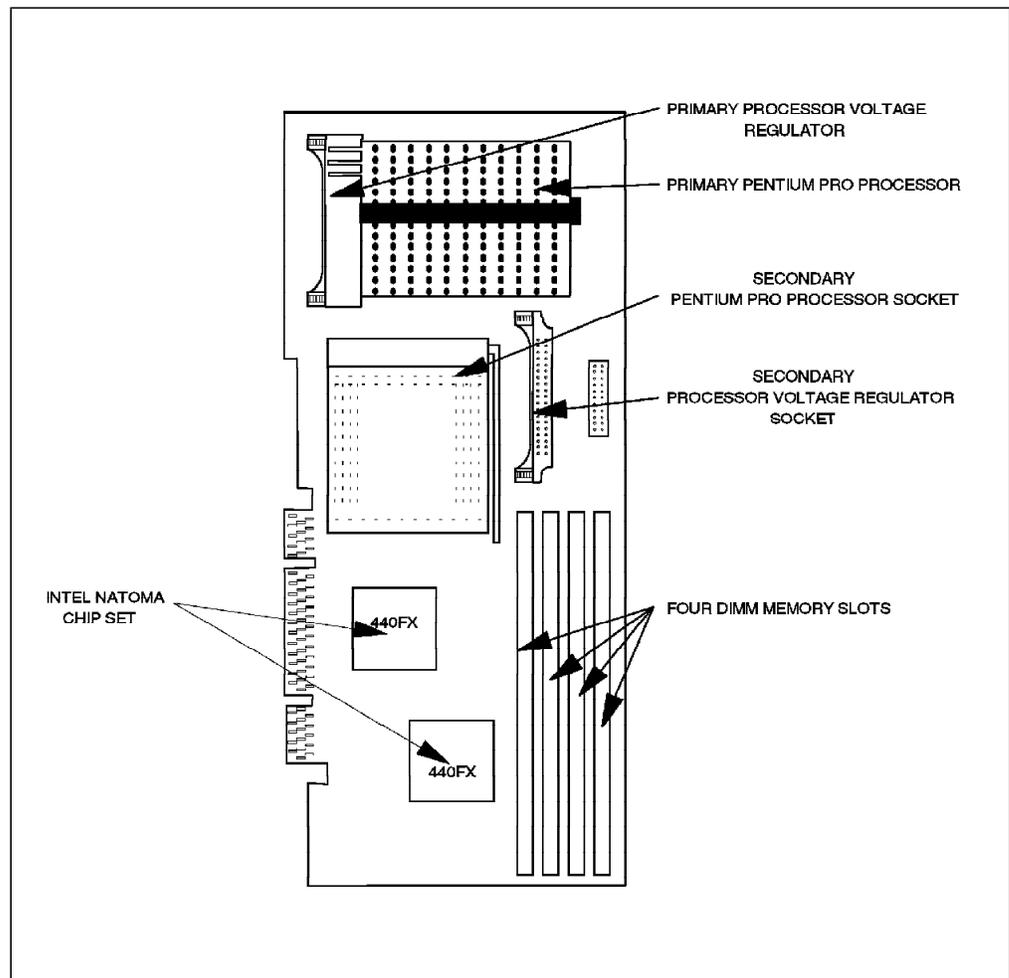
Figure 38. IBM PC Server 325 Processor Board
