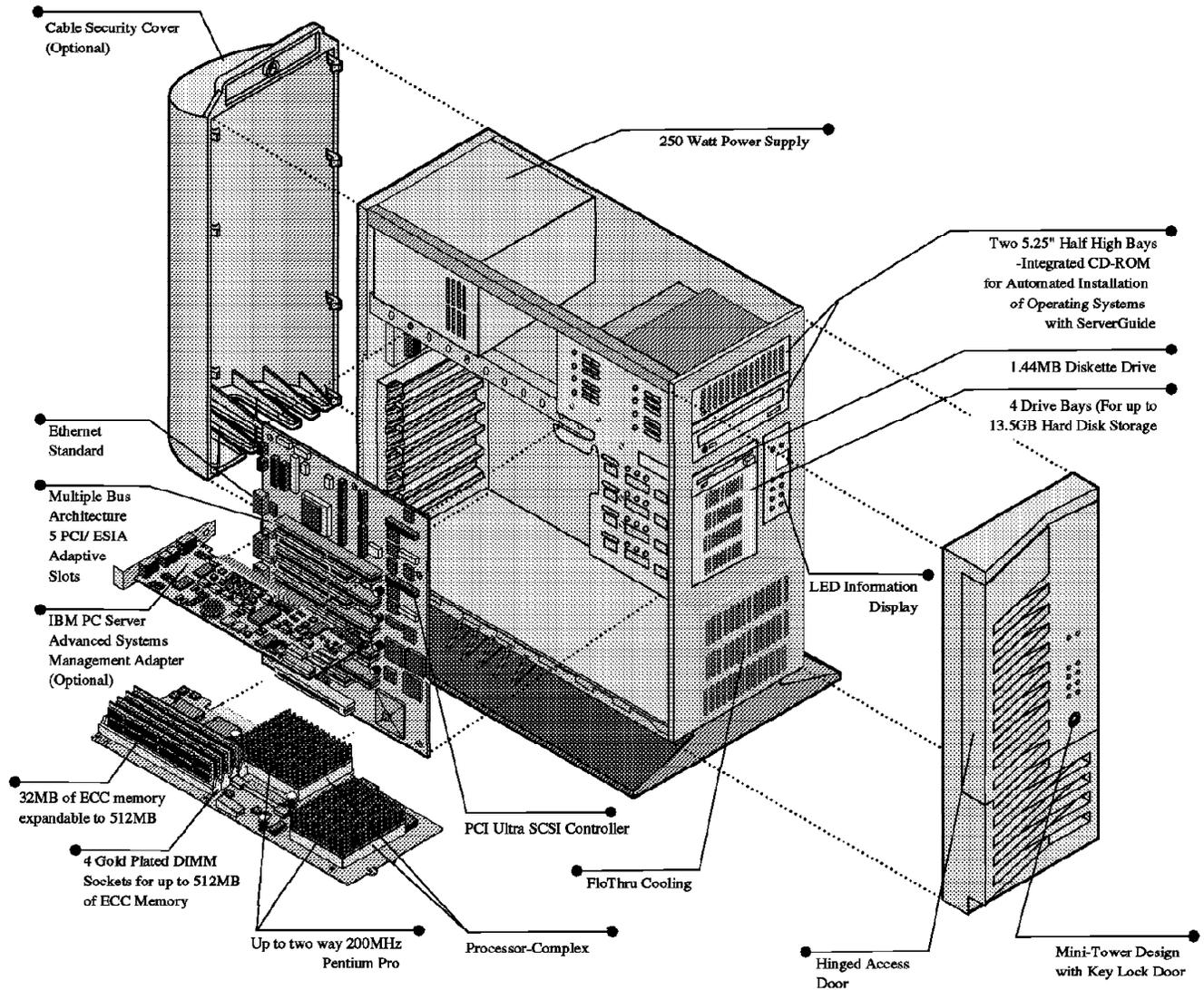
Figure 37. Exploded View of the IBM PC Server 325 Mini Tower Model
