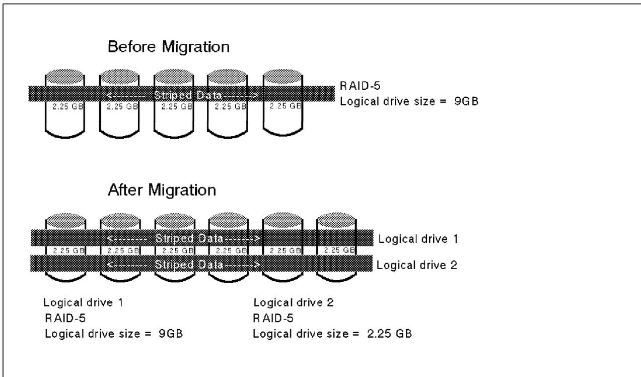
Figure 58. Addition of One Disk to a RAID-5 Array
