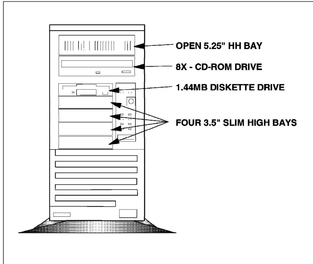
Figure 41. IBM PC Server 325 Expansion Bays
