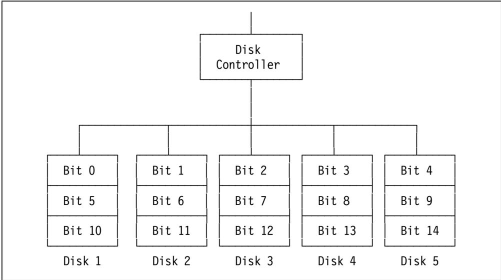
Figure 26. RAID-2 (Bit Interleave Striping with Hamming Code)
