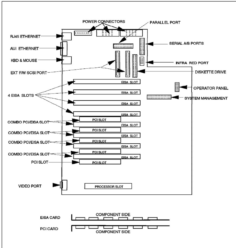
Figure 44. View of the IBM PC Server 330 System Board
