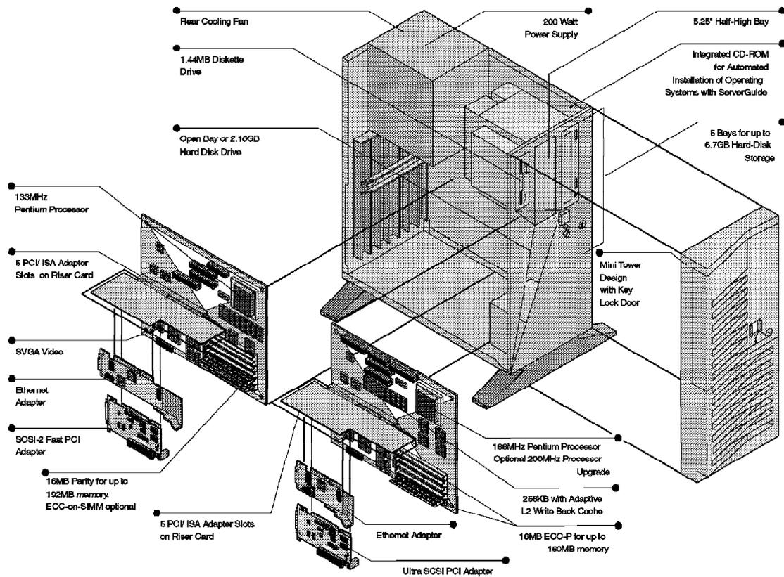
Figure 35. Exploded View of the IBM PC Server 310
