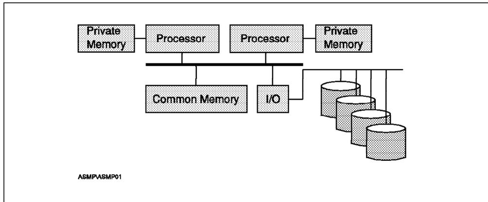
Figure 3. Asymmetric Multiprocessing Example 1. This configuration has multiple memory units with some of those not shared by all processors.
