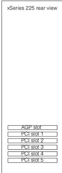
Slot 1: Bus C, 32-bit, 33MHz, 5v, half-length
