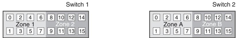
Figure 49. Switch zoning for the Intra-site configuration
