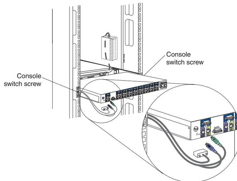
6. Route the keyboard, video, and mouse cables through the channel in the left-side bracket on the console switch; then, connect the keyboard, video, and mouse connectors to the console switch.
