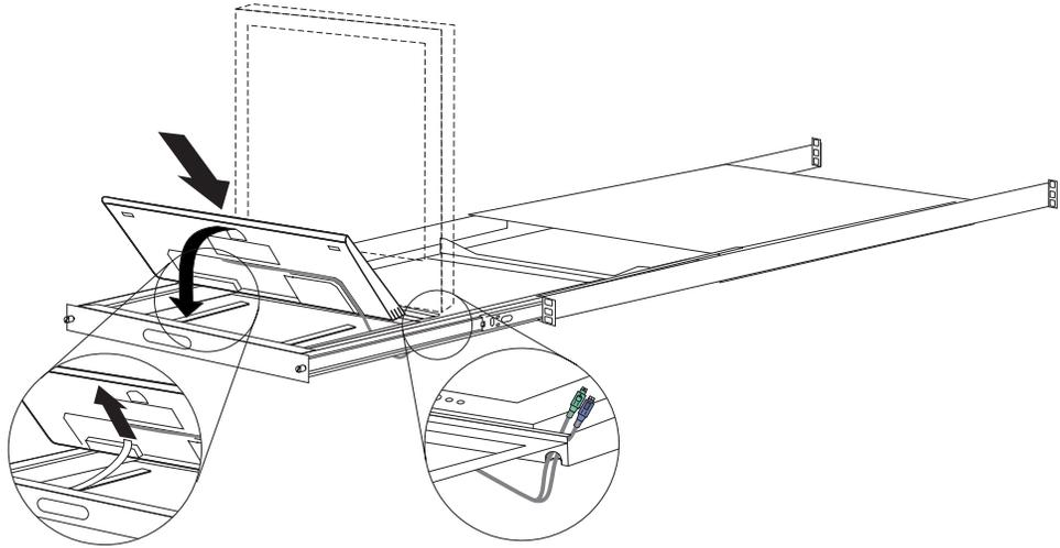
7. Carefully set the keyboard into the tray; then, route the keyboard and mouse cable beside the video cable and towards the cable-management arm.
