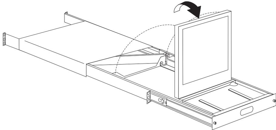
5. To remove the cable cover from the tray, remove the cable-cover screw from underneath the tray; then, slide the cover toward the rear of the tray until the tab on the cover is out of the slot in the front of the tray. Lift the cable cover from the tray and set it aside to install later in this procedure.
