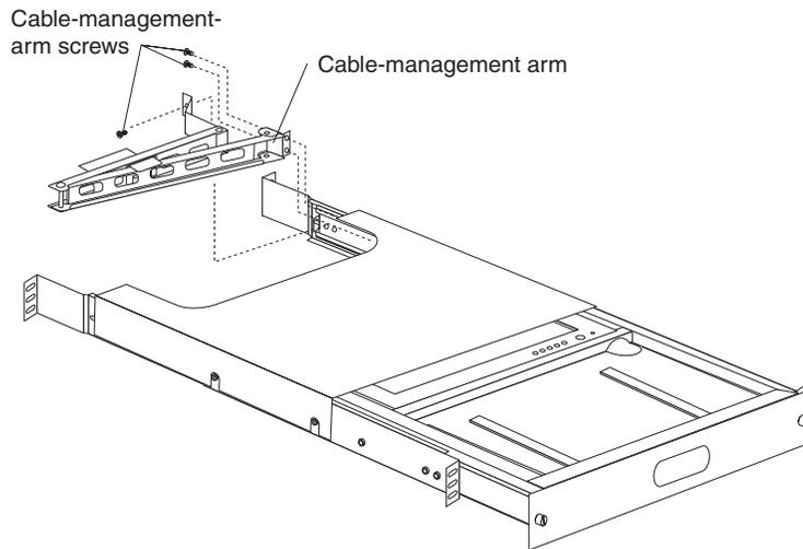
6. Route the keyboard, mouse, video, and power cables through the new cable-management arm and secure them along the way with cable straps.
