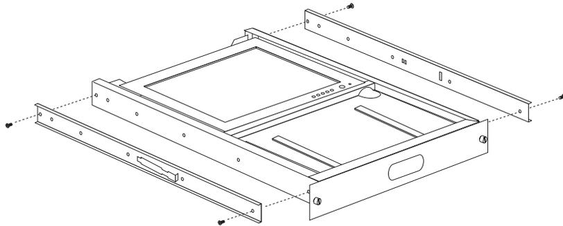
7. Slide the new slide rail assemblies onto each side of the tray.
