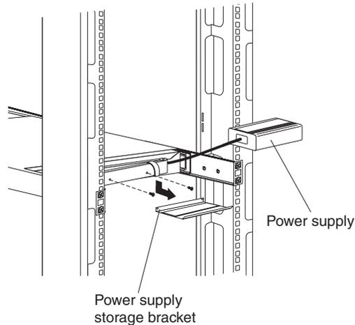
4. To remove the power supply storage bracket from the cable-management arm, remove the two screws and pull the bracket away from the arm. Store the parts in a safe place for possible future use.
