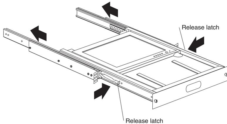
6. Remove the two screws per side that attach the remaining slide rail pieces to the tray; then, attach the corresponding new slide rail pieces to the tray using the same screws.
