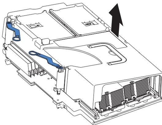
Figure 28. Lifting the cover off
