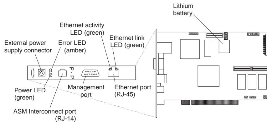
Figure 8. Remote Supervisor Adapter connectors and LEDs
