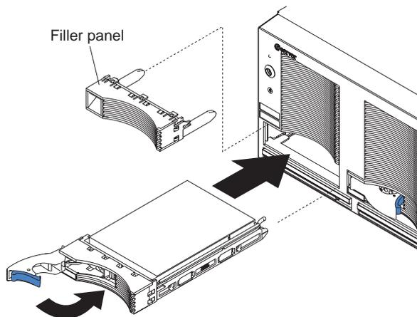
Figure 21. Installing a hard disk drive
