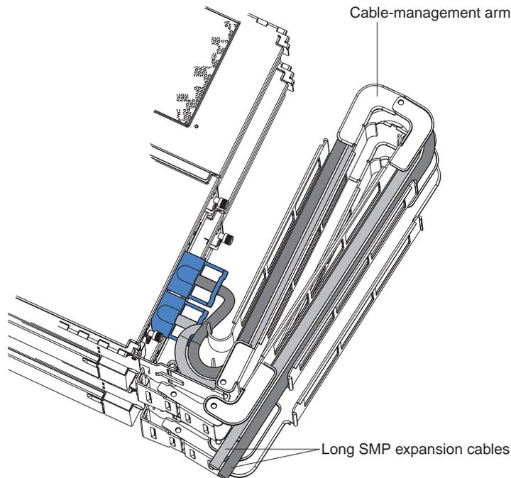
Figure 60. Routing cables through the cable management arm
