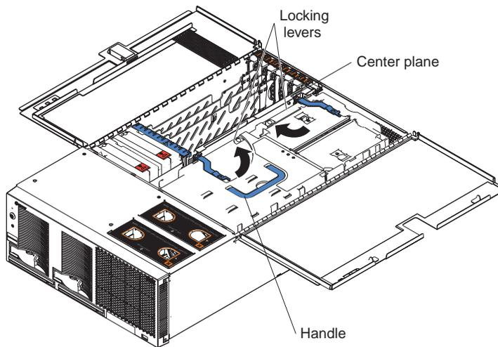
Figure 31. SMP Expansion Module locking lever position
