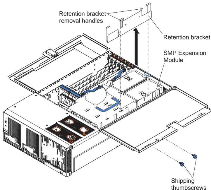
Figure 24. Removing the retention bracket and shipping thumbscrews
