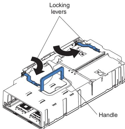
Figure 30. Locking lever position for installing the SMP Expansion Module
