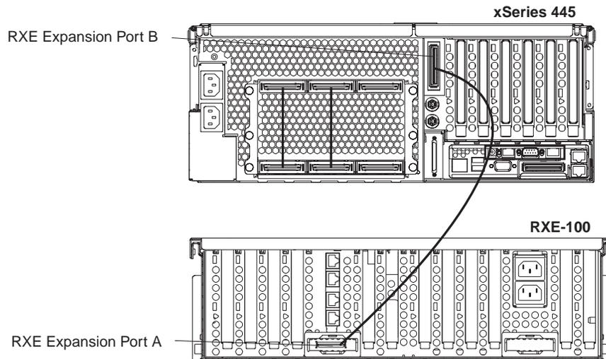
Figure 64. RXE Expansion port cabling a server with two SMP Expansion Modules
