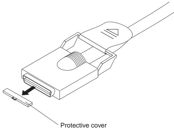
Figure 61. RXE Expansion cable with protective cover
