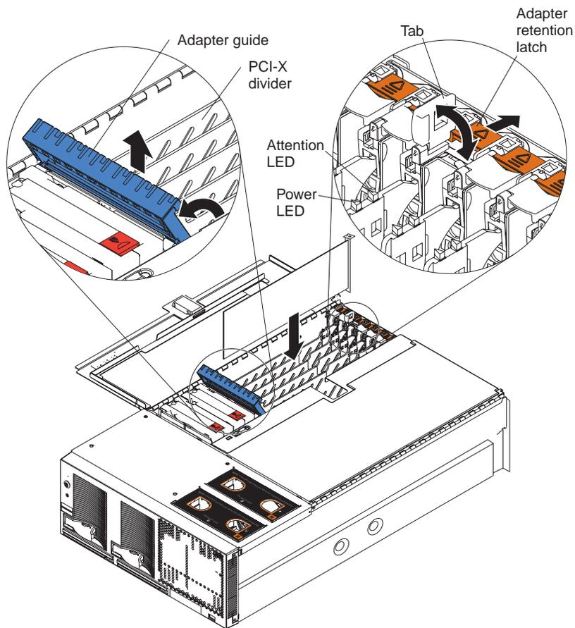
Figure 15. PCI-X slot components
