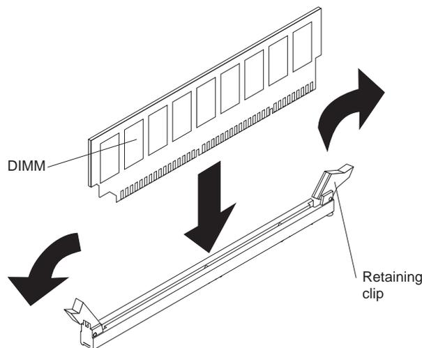
Figure 37. Inserting a DIMM into a DIMM slot
