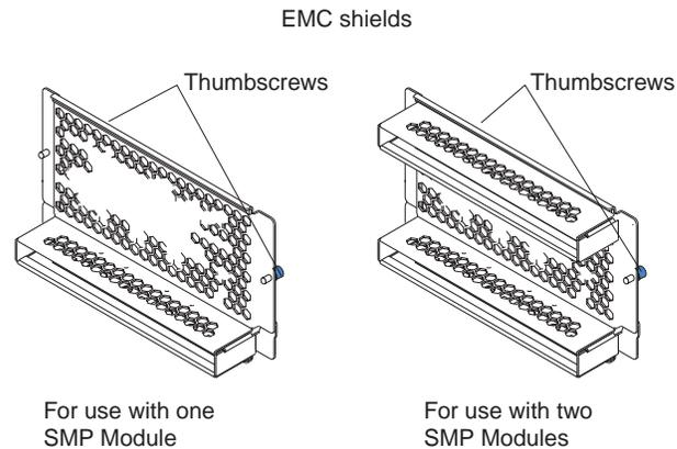
Figure 25. EMC shields
