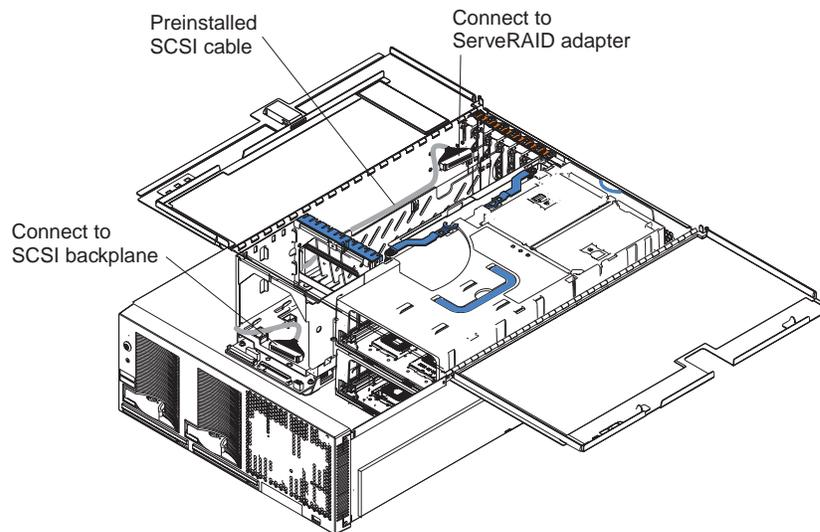
*Figure 16. Location of preinstalled SCSI cable*
