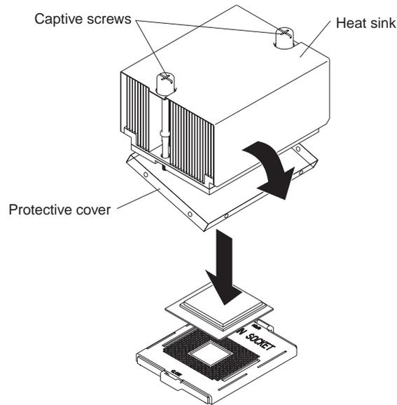
Figure 47. Aligning the heat sink over the microprocessor
