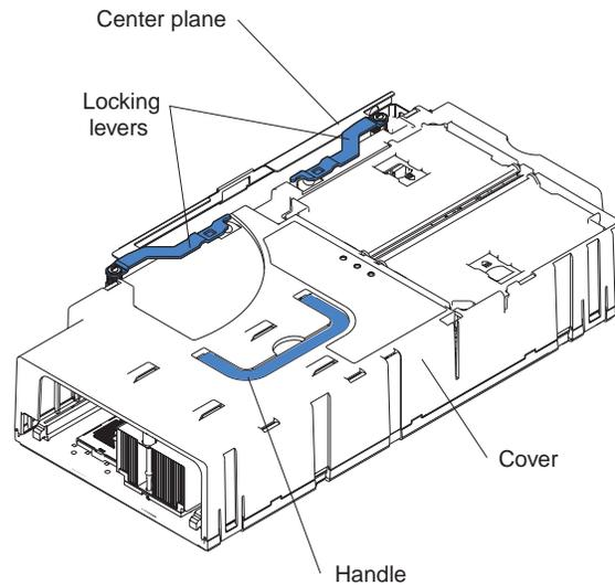
Figure 32. Locking lever position when the SMP Expansion Module is installed
