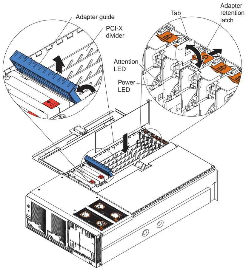
Figure 18. PCI-X slot components
