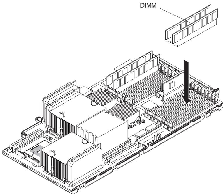
Figure 35. DIMM installation
