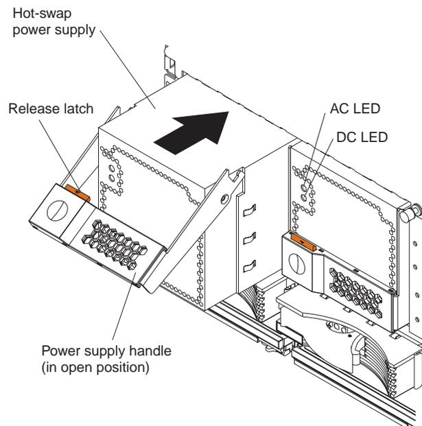
Figure 13. Installing a power supply
