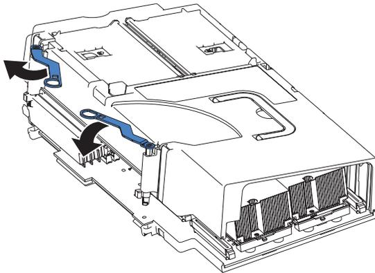
Figure 27. Fully extending the locking levers to remove the SMP Expansion Module cover
