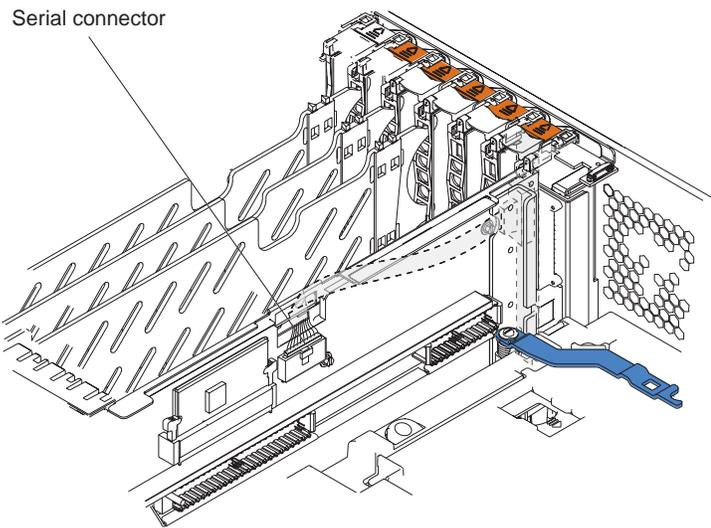
Figure 20. Route the serial port ribbon cable through the slot
