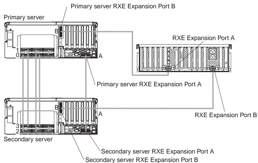
Figure 68. RXE Expansion Port cabling in a 16-way configuration
