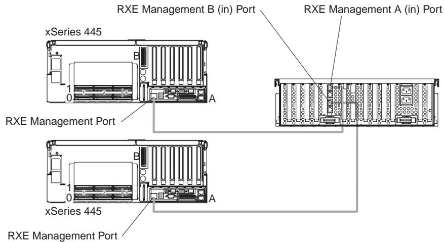
Figure 70. Cabling an RXE Management port - two stand-alone servers
