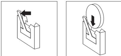
Figure 52. Installing the battery
