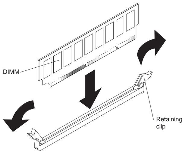
Figure 39. Inserting a DIMM into a DIMM slot
