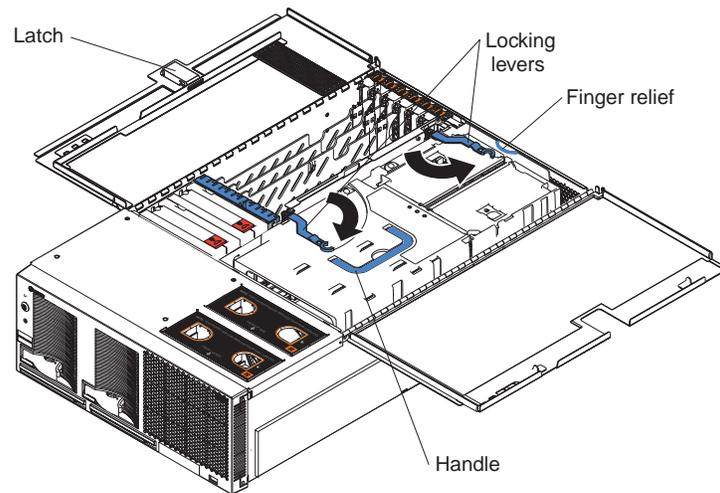
Figure 26. Rotate the locking levers to remove the SMP Expansion Module
