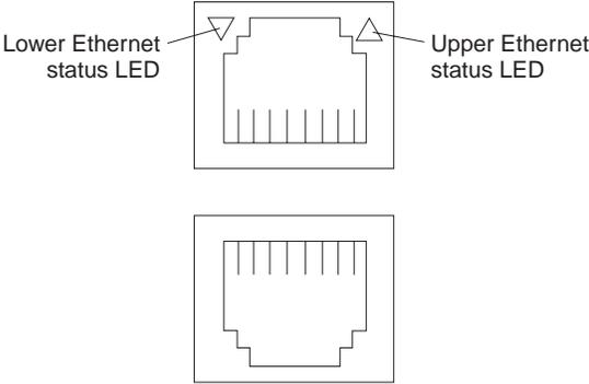
Figure 73. Gigabit Ethernet port
