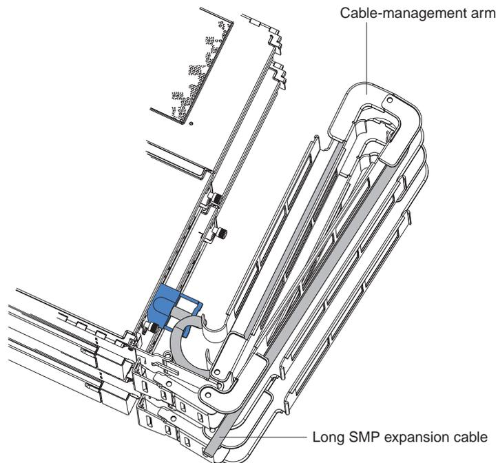
Figure 59. Routing cables through the cable management arm
