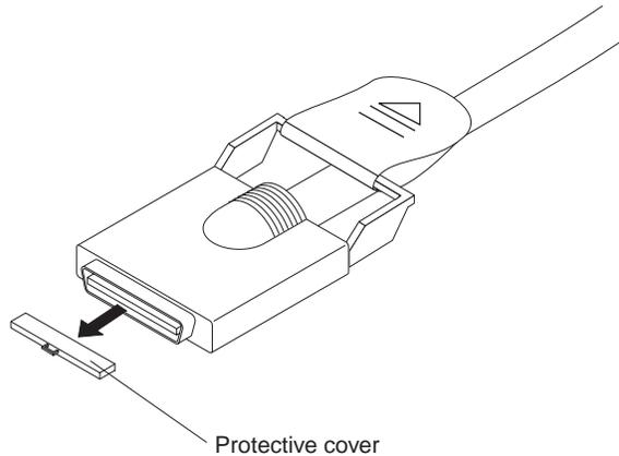
Figure 65. RXE Expansion cable with protective cover
