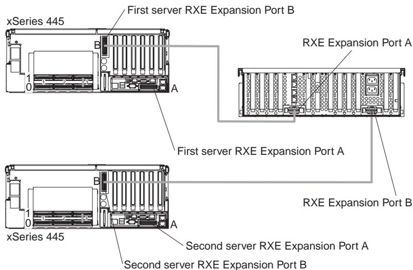
Figure 66. RXE Expansion Port cabling of two stand-alone xSeries 445 servers to a single remote I/O enclosure
