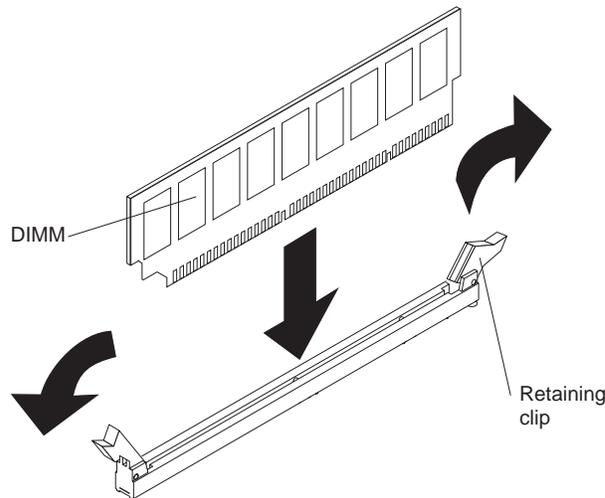
Figure 41. Inserting a DIMM into a DIMM slot
