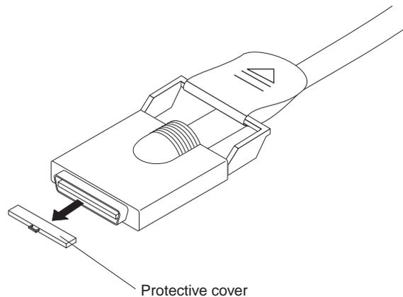
*Figure 57. SMP Expansion cable with protective cover*
