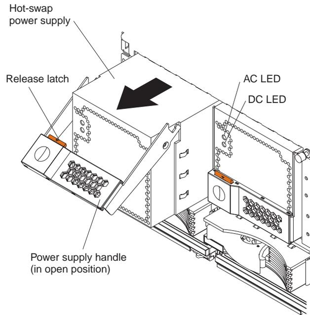
Figure 12. Removing a power supply
