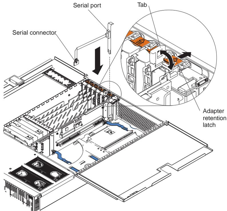
Figure 19. Insert the serial port into PCI-X slot 1
