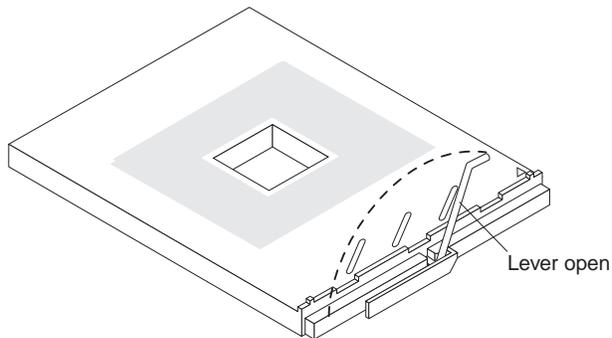
Figure 46. Microprocessor locking lever fully open
