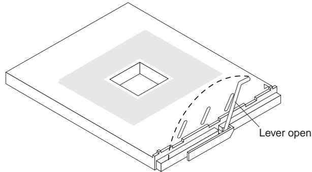
Figure 44. Microprocessor locking lever fully open
