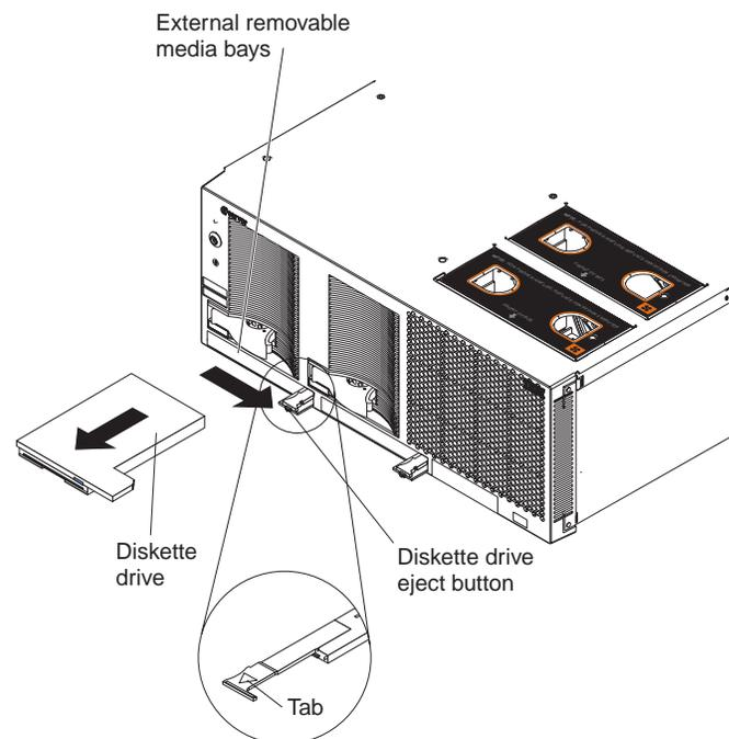
Figure 22. Installing a diskette disk drive
