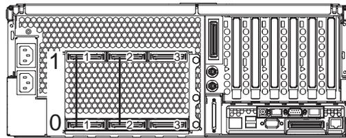
Figure 55. SMP Expansion Module numbering
