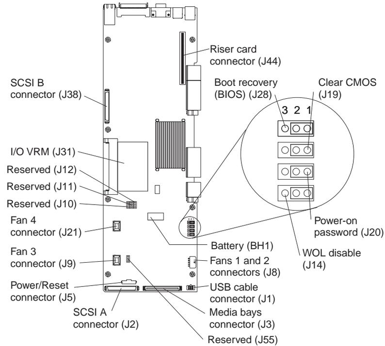
Figure 7. I/O board connectors
