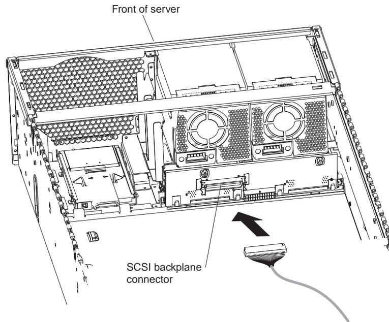
Figure 17. Connecting the SCSI cable to the SCSI backplane
