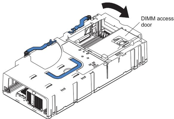
Figure 36. Opening the DIMM access door
