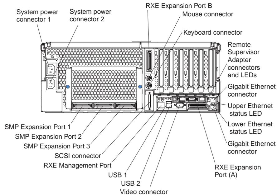
Figure 72. Rear view of xSeries 445
