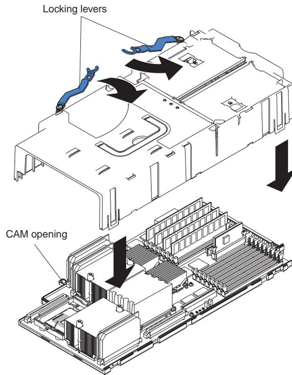
Figure 29. Installing the SMP Expansion Module cover
