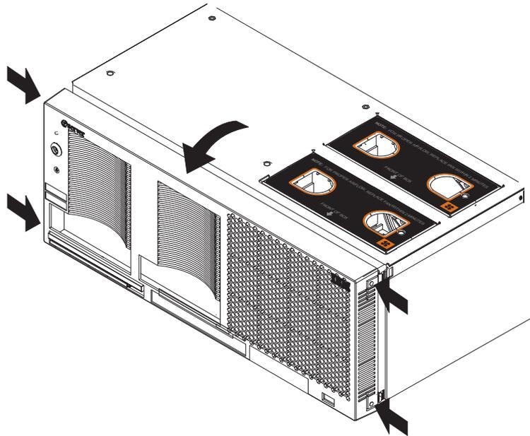
*Figure 10. Removing the bezel*
