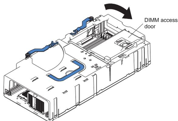
Figure 38. Opening the DIMM access door
