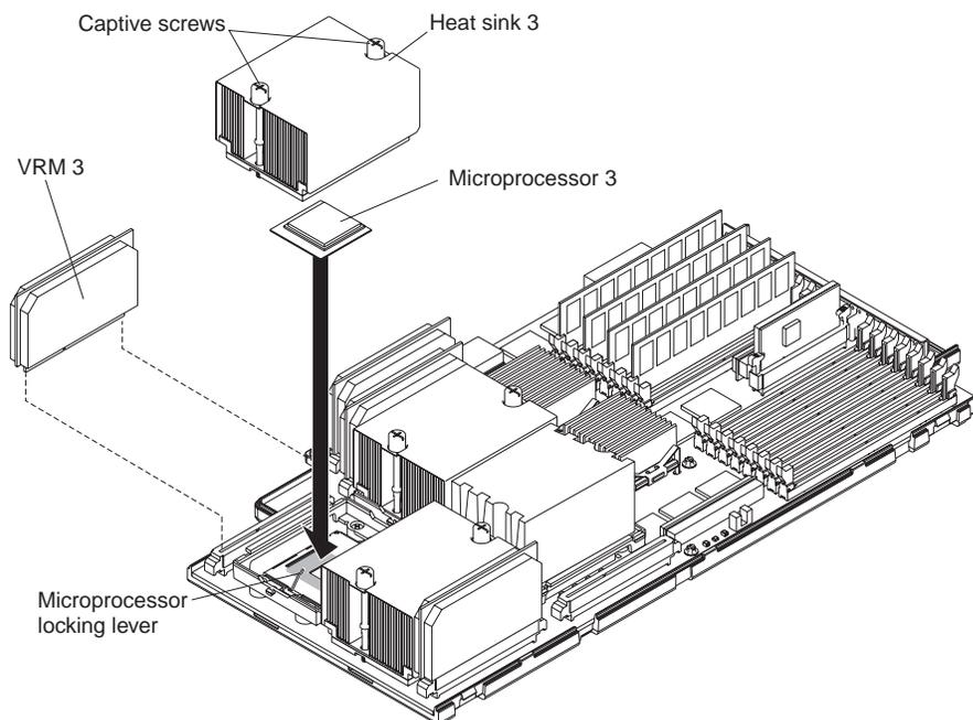
Figure 43. Microprocessor installation
