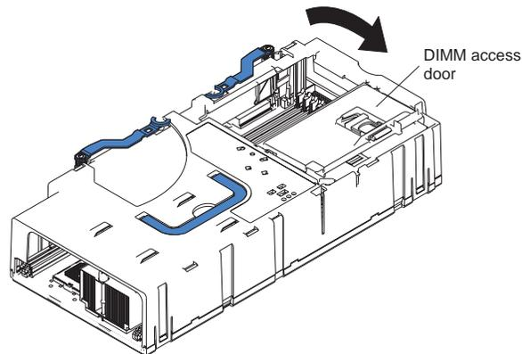
Figure 40. Opening the DIMM access door
