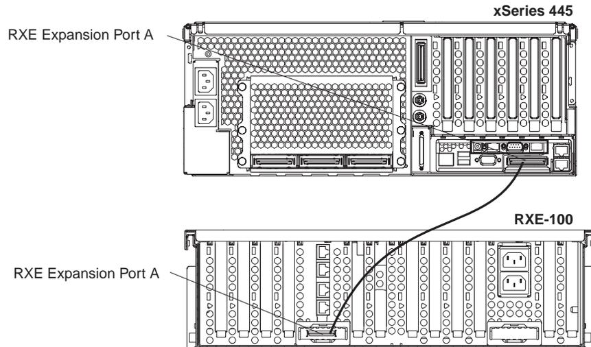
Figure 62. RXE Expansion Port cabling a server with one SMP Expansion Module
