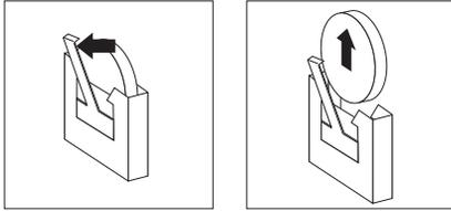
Figure 51. Removing the battery
