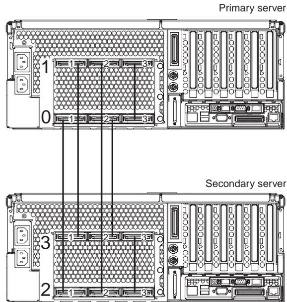
Figure 58. 16-way SMP Expansion port cabling
