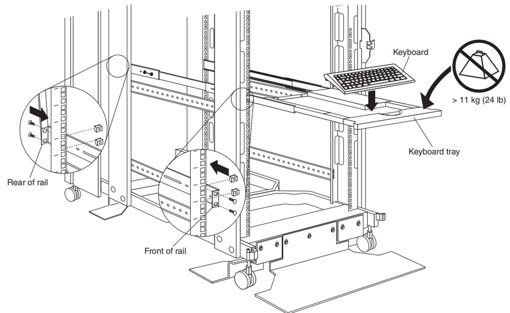
Figure 38. Installing a keyboard tray and keyboard
