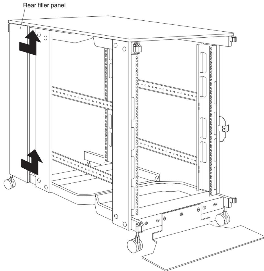
*Figure 9. Removing the NetBAY25 rear filler panels*
