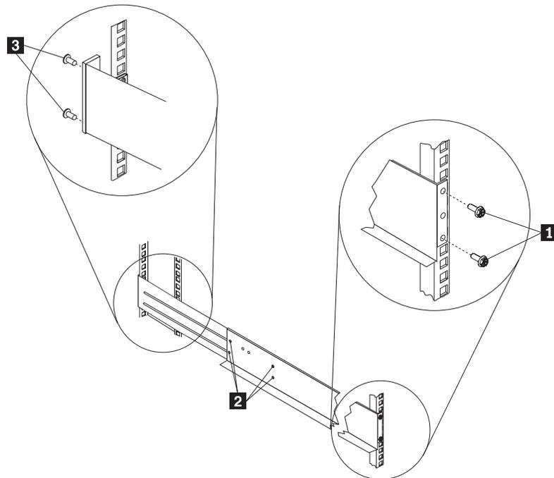
6. Loosely insert one M5 screw **1** into each rail.
