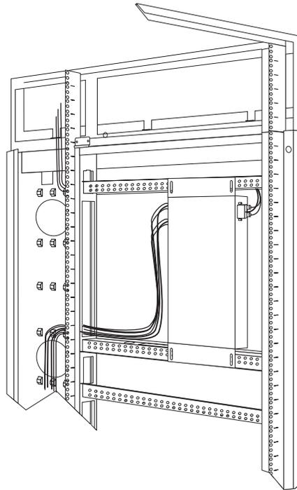
6. Connect the monitor signal cable from your monitor to the blue monitor connector on Port **A** of the console switch; then, tighten the screws on the monitor signal cable.
