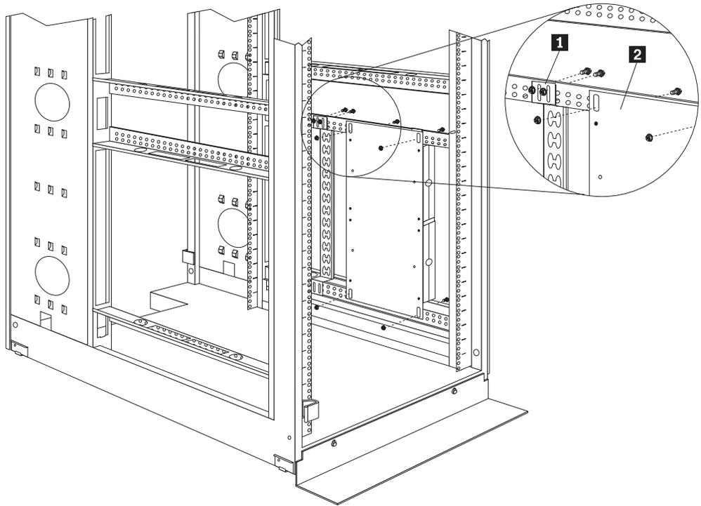
Figure 59. Installing the vertical mounting plate and cable-management bracket
