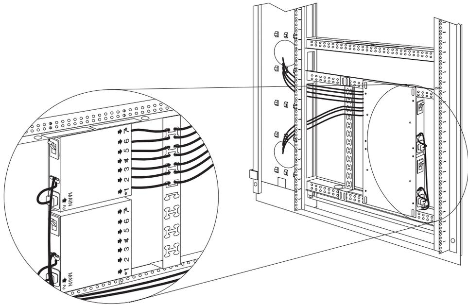
Figure 51. Connecting and routing other power cables to the outlets
