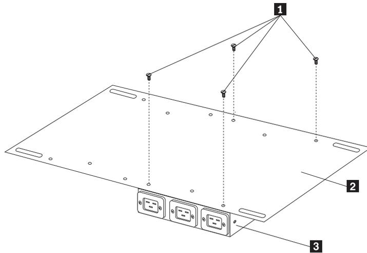
Figure 57. Installing the Rack PDU on the vertical mounting plate
