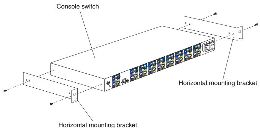
3. Determine the appropriate U level within the EIA mounting space; then, install the console switch in the rear of your rack cabinet using four M6
