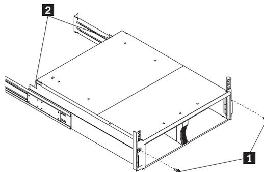
8. Tighten the rear screws **2**.
