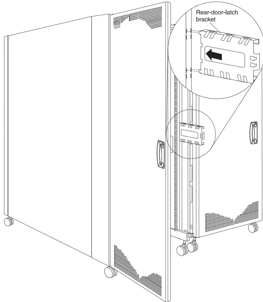
Figure 18. Installing the rear-door-latch-bracket on a rack cabinet
