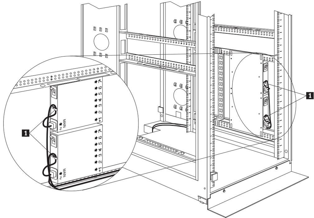
Figure 50. Connecting and routing the line cord
