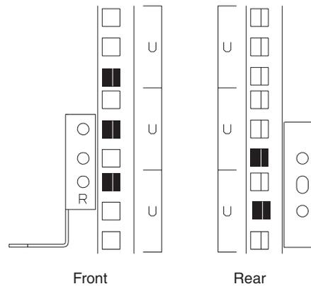
**Note:** Use clip nuts if your rack has circular holes. If your rack has square holes, you can use the rack-insertion tool or a flat-blade screwdriver to install cage nuts.
