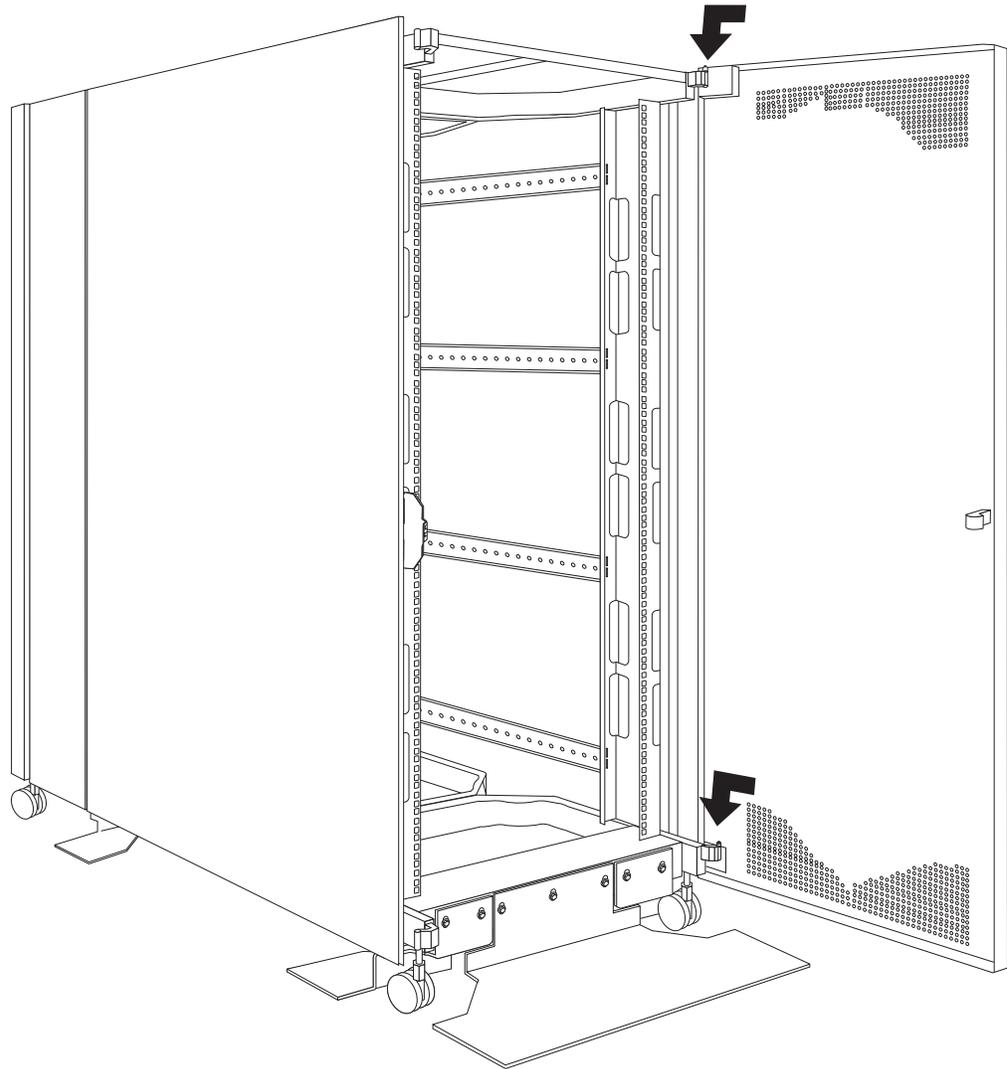
Figure 15. Rotating and installing the door
