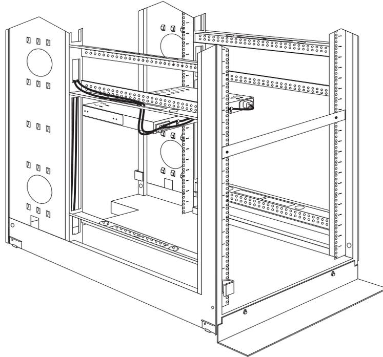
Figure 52. Connecting and routing the line cord
