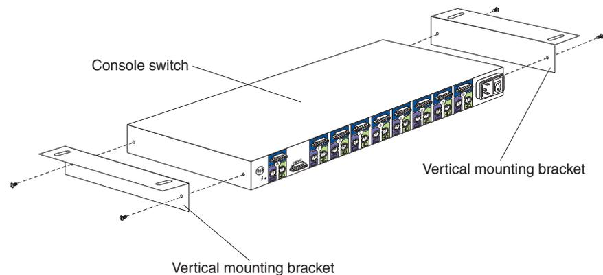
3. Hold the console switch against the side braces, with the rear of the console switch facing the back of your rack cabinet; then, use four M6 screws and nuts
