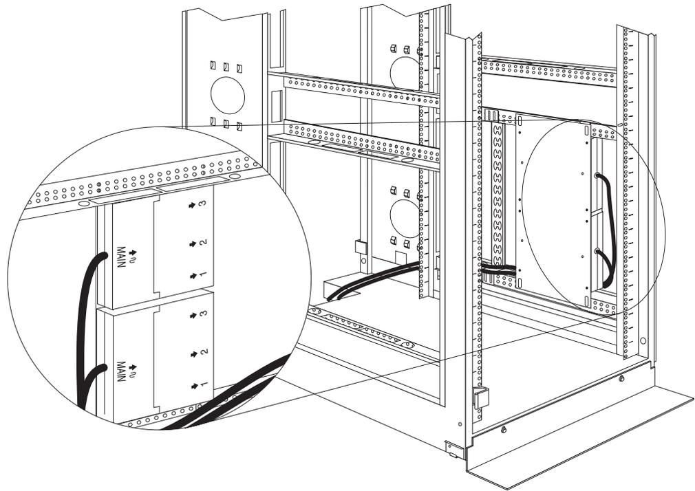
Figure 60. Routing the fixed line cords
