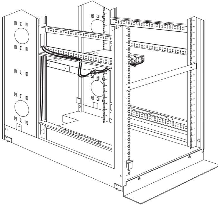
Figure 71. Connecting and routing the line cords
