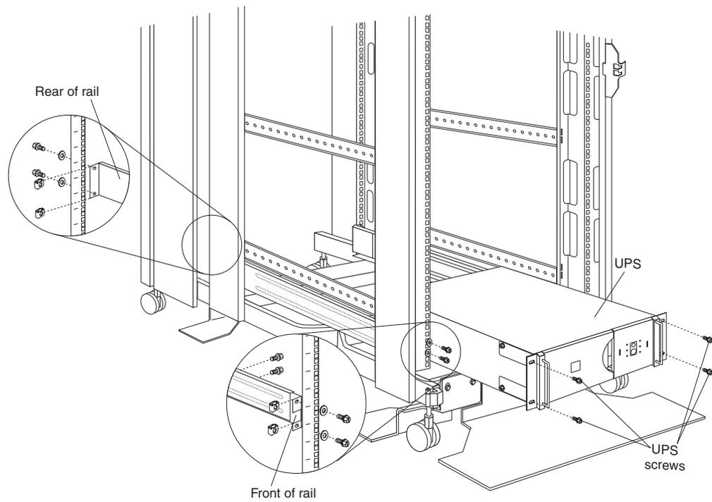
Figure 28. Installing a UPS
