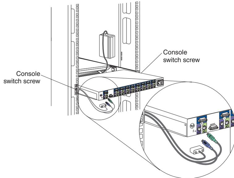
5. Route the keyboard, video, and mouse cables through the slot in the left-side bracket on the console switch; then, connect the keyboard, video, and mouse connectors to the console switch.
