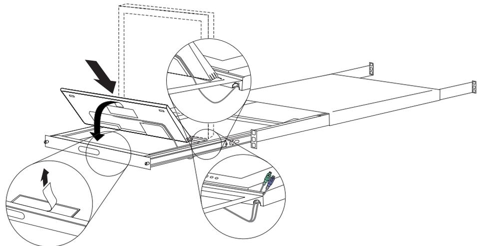
7. To install the keyboard in the tray, align the top slot on the rear of the keyboard with the back edge of the large rectangular opening in the front of the tray; then, carefully rotate the front of the keyboard down and into the tray.
