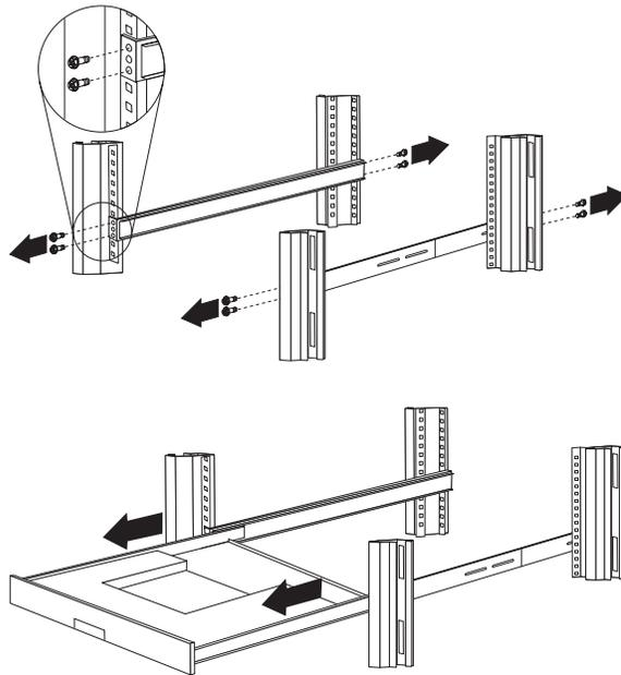
To remove the tray from the side rails, pull up on the left rail tab and push down on the right rail tab.
