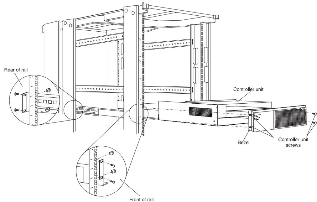
Figure 34. Installing a Fibre Channel RAID controller unit
