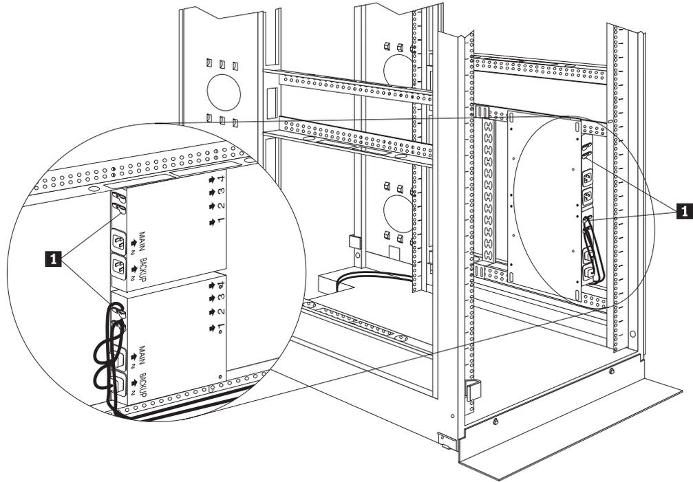
Figure 69. Connecting and routing the line cords
