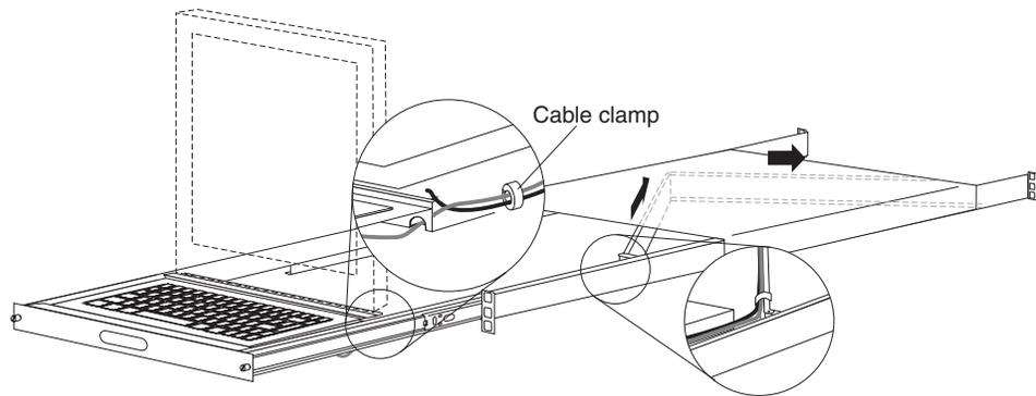
9. Secure the keyboard and mouse cable to the cable-management arm using the existing cable straps; then, install the cable cover that you removed earlier.
