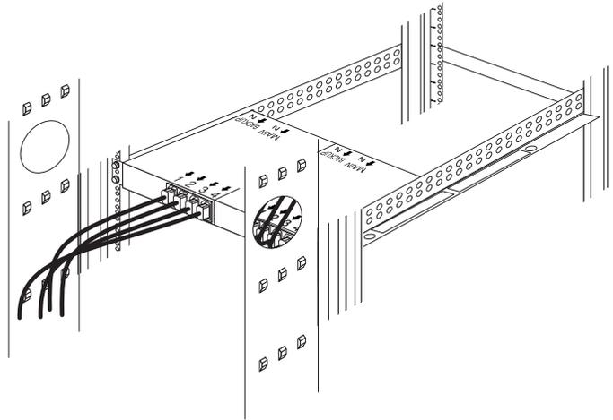
Figure 72. Connecting and routing other power cables to the outlets
