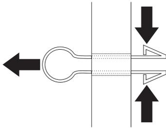
Figure 79. Removing the plastic cable clamp
