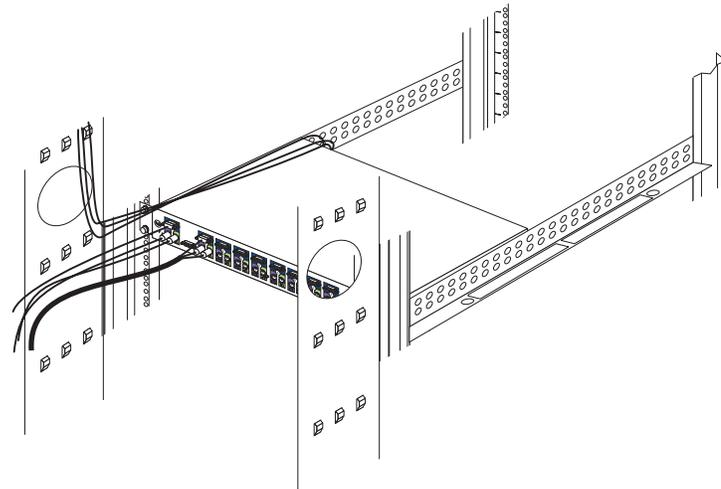
6. Connect the monitor signal cable from your monitor to the blue monitor connector on Port **A** of the console switch; then, tighten the screws on the monitor signal cable.
