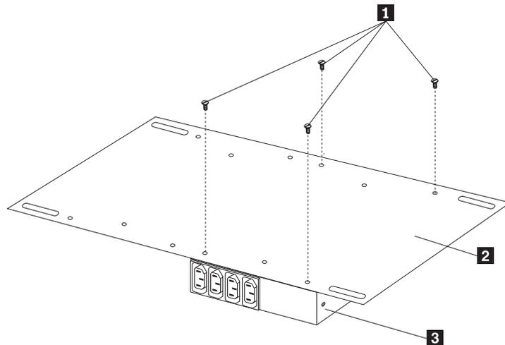
Figure 62. Installing the Rack PDU on the vertical mounting plate
