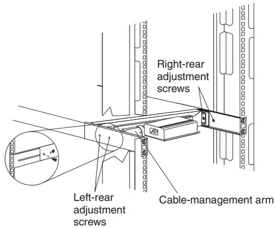
16. To attach the front of the tray to the rack cabinet, pull the tray halfway out of the rack cabinet so that you can access the front of the rails; then, use four of the screws from the miscellaneous hardware kit to secure the slide-rail brackets to the rack cabinet.
