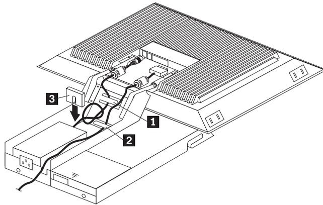
Figure 85. Storing the power supply and routing cables
