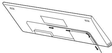
6. Peel the protective strip from the hook-and-loop fastener strip inside the keyboard storage area; then, route the keyboard and mouse connectors through the small round opening on the right side of the tray.
