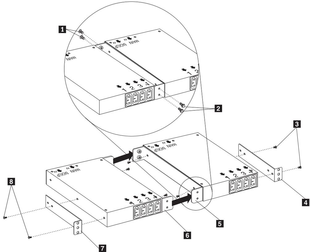
Figure 67. Installing the mounting brackets for two devices
