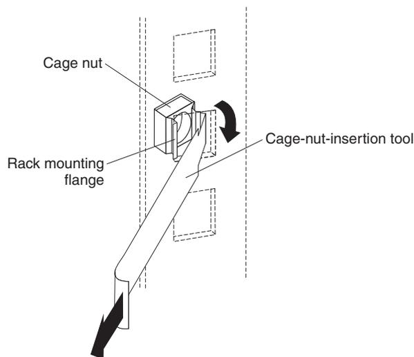
Figure 26. Installing cage nuts with the cage-nut-insertion tool
