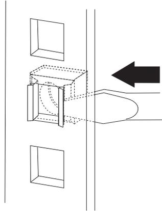
Figure 27. Installing cage nuts with a flat-blade screwdriver
