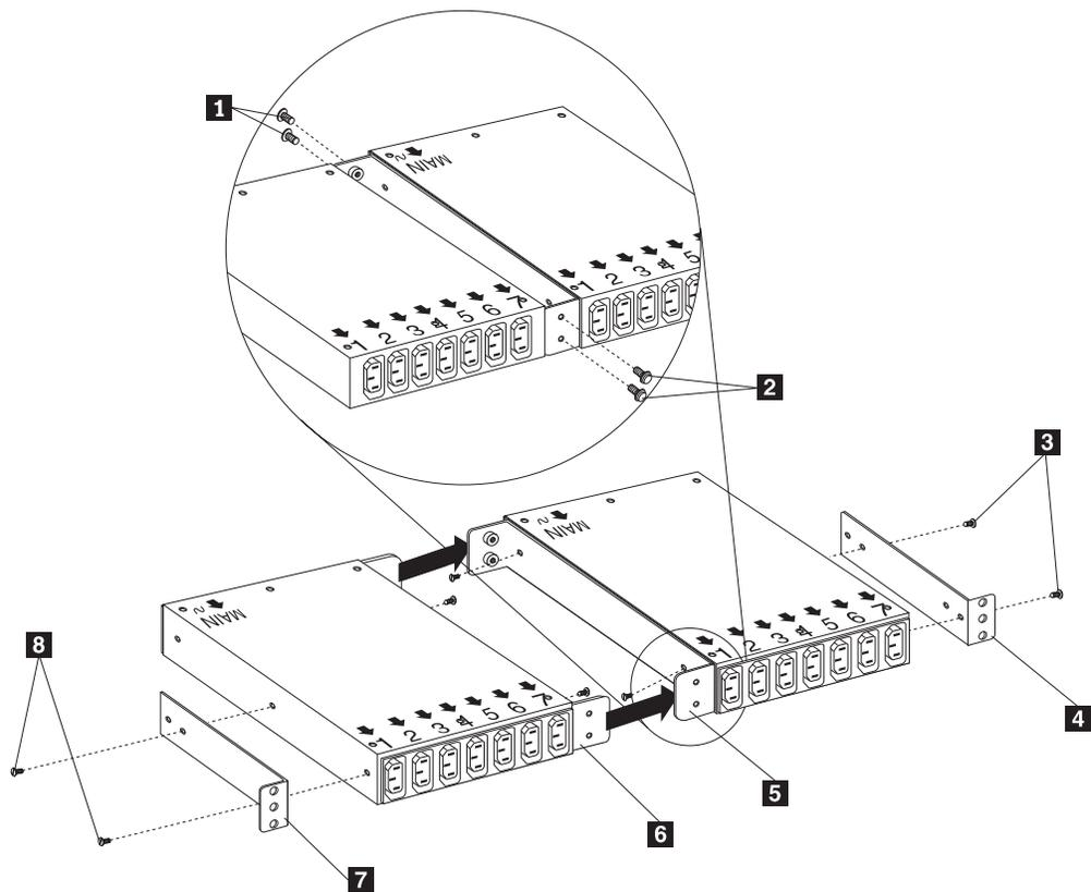
Figure 48. Installing the mounting brackets for two devices
