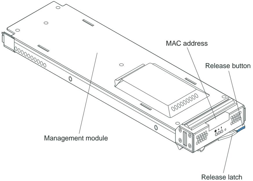
The IBM @server BladeCenter T Management Module is a hot-swap unit that is installed into the front of the BladeCenter T unit. The module contains the video compression boards.
