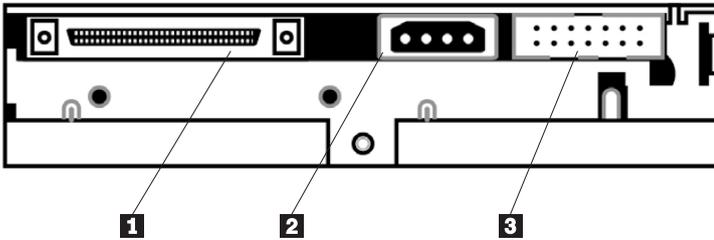
**1** 68-pin high density SCSI connector    **2** Power connector    **3** SCSI ID jumpers
