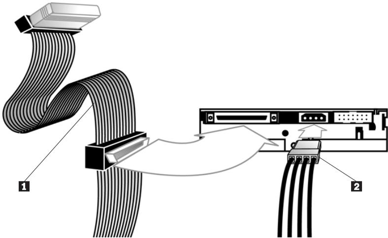
**1** SCSI cable (shown with terminator installed)
