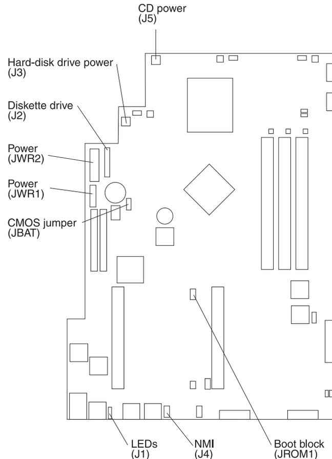
3. Move the JROM1 jumper to the alternate position (pins 1 and 2) to enable the BIOS recovery mode.
