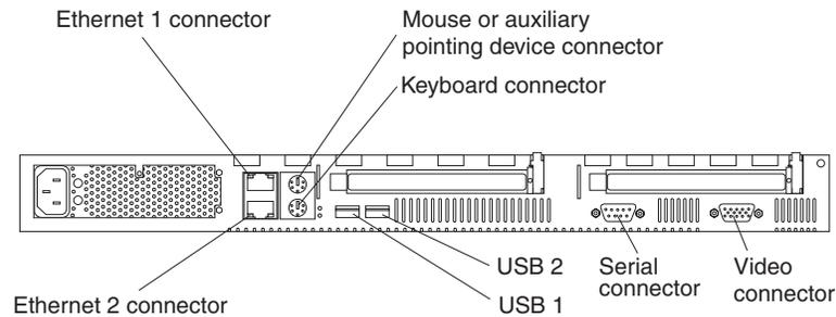
To effectively manage the cables on this server, keep groups of cables secured together, and do not run cables across the back of the server.
