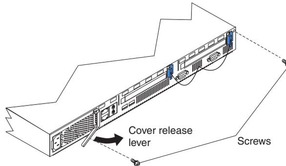
3. Remove the two screws from the rear of the server.
