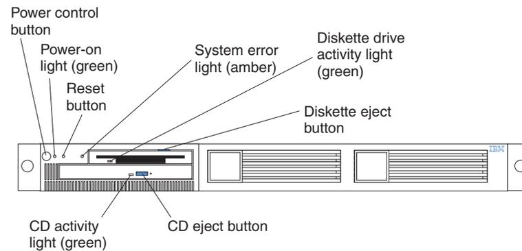
**Power-control button:** Press this button to manually turn the server on or off.
