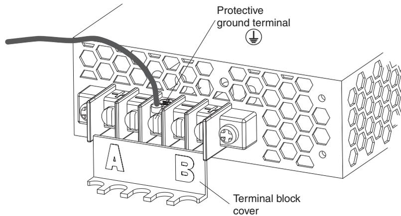
2. Connect the wires to the power supply in the following order:
