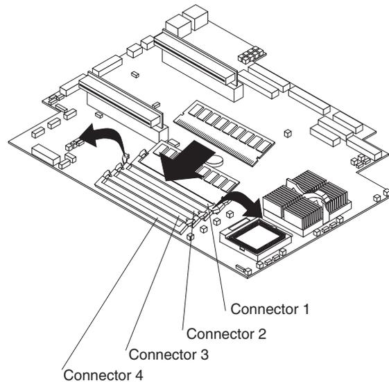
**Attention:** To avoid breaking the retaining clips or damaging the DIMM connectors, handle the clips gently.
