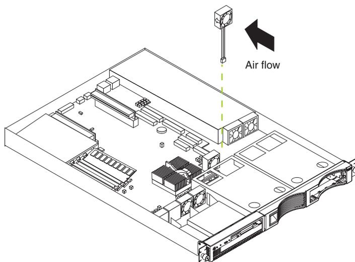
6. Push the replacement fan assembly into the server until it clicks into place.
