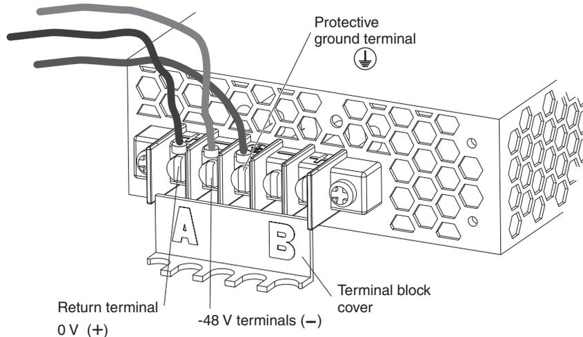
3. Connect the first set of inputs to the A set of terminals as follows:
