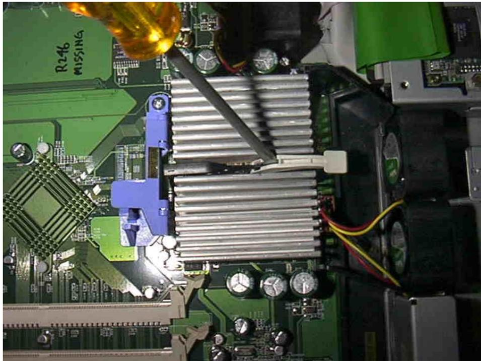
If the handle breaks, remove the handle by placing a screw driver in between both sides of the handle as in the picture above, and twist the screw driver to break off the handle to relieve the pressure from the clip to the heat sink, as in the picture below.
