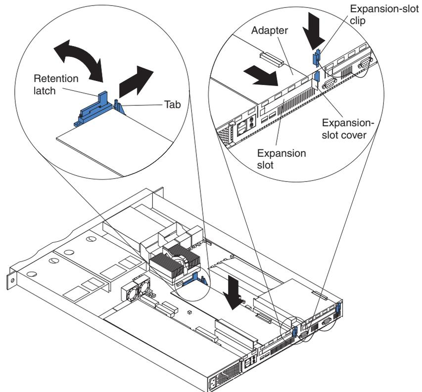
6. Remove the expansion-slot cover.
