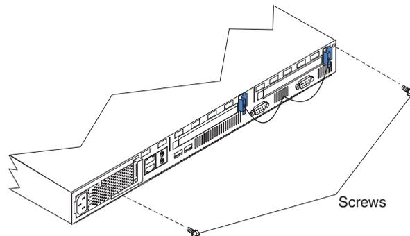
2. Install the screws to secure the cover as shown.
