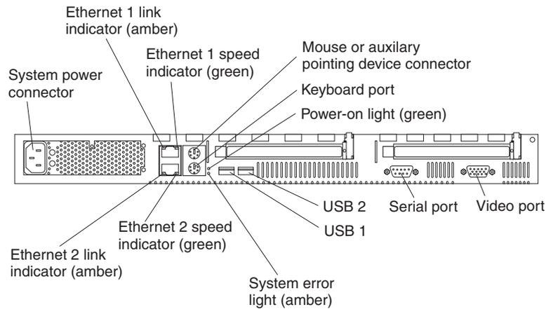
**System power connector:** The system power cord connects here to provide power to the system.
