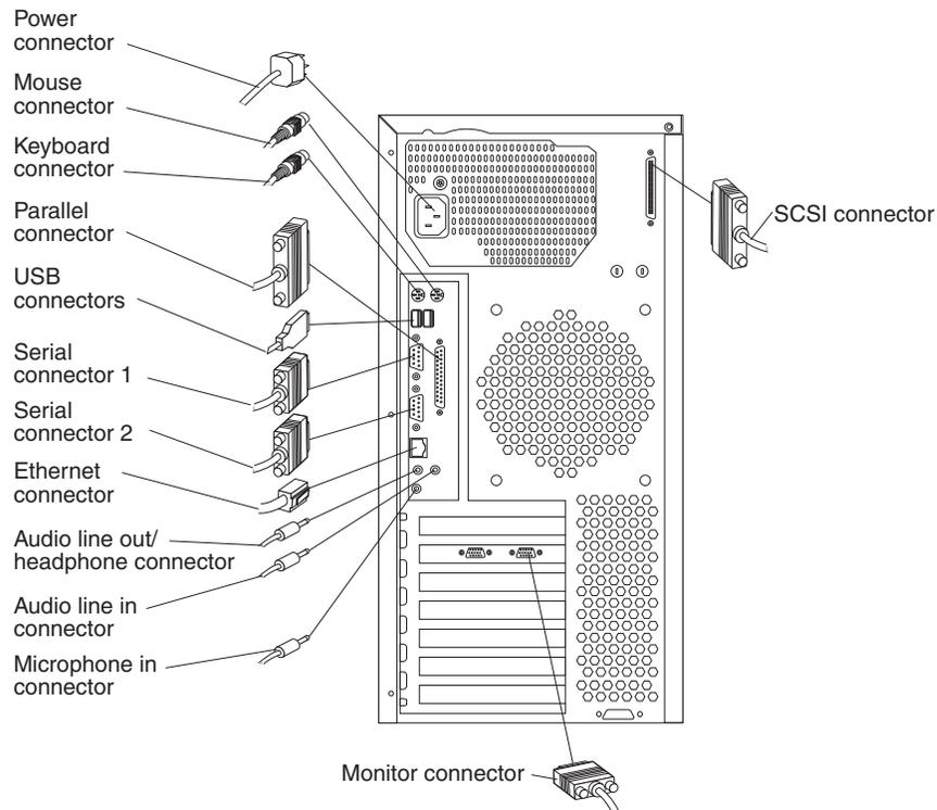
This section provides information about the I/O connectors on the rear of the computer. These connectors include the following:
