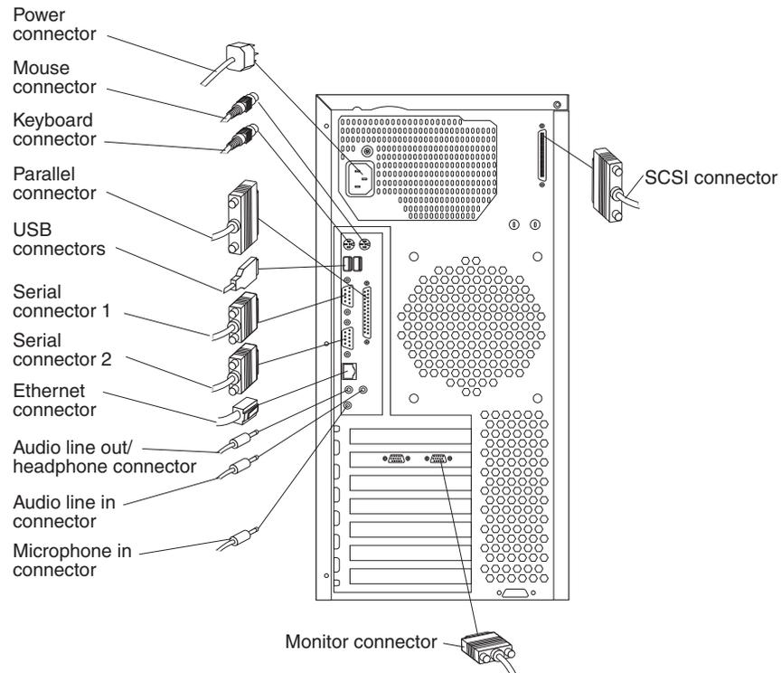
**Note:** The location of the monitor connector is dependent on the video adapter installed on the computer.
