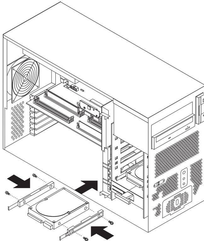
4. Slide the hard disk drive along the rail guides into the drive bay.
