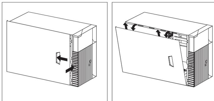
7. Lift the lever at the top of the chassis and pull the front bezel from the front of the computer. You might need to move the computer closer to the edge of the desk to completely rotate the bezel down to remove it.
