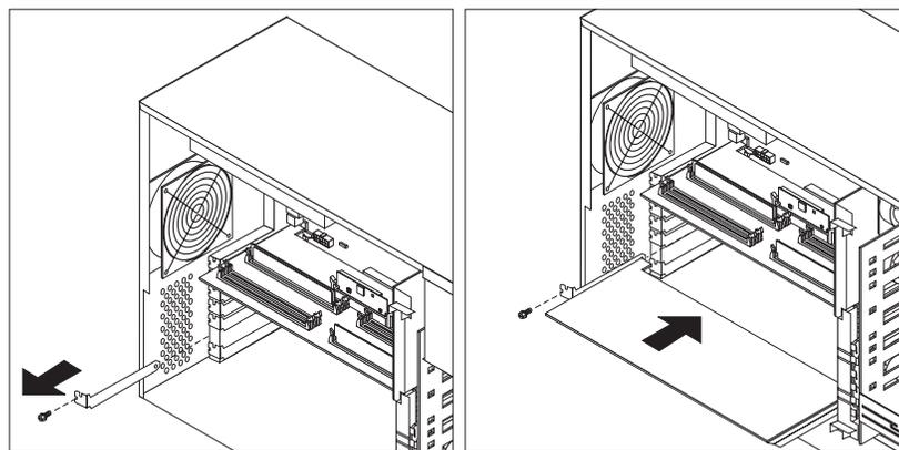
9. Replace the PCI adapter retention bracket or adapter retention screw (depending on the model).
