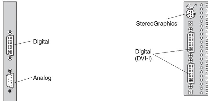
**Note:** The Wildcat III 6110 adapter occupies the AGP slot and the adjacent PCI slot. Be careful when you install an adapter in PCI slot 2 because the space between the Wildcat III 6110 adapter and PCI slot 2 is very limited, which causes the adapters to be very close to each other.
