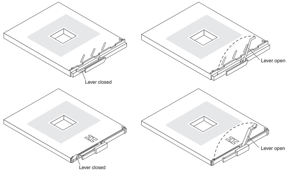
11. Insert the microprocessor in the microprocessor socket, lining pin number 1 up with the microprocessor.
