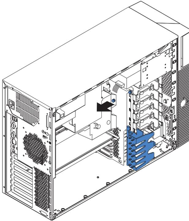
2. Slide the air baffle back slightly and lift it to remove it.
