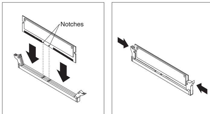
9. Place the memory board into the MEC connector on the system board.
