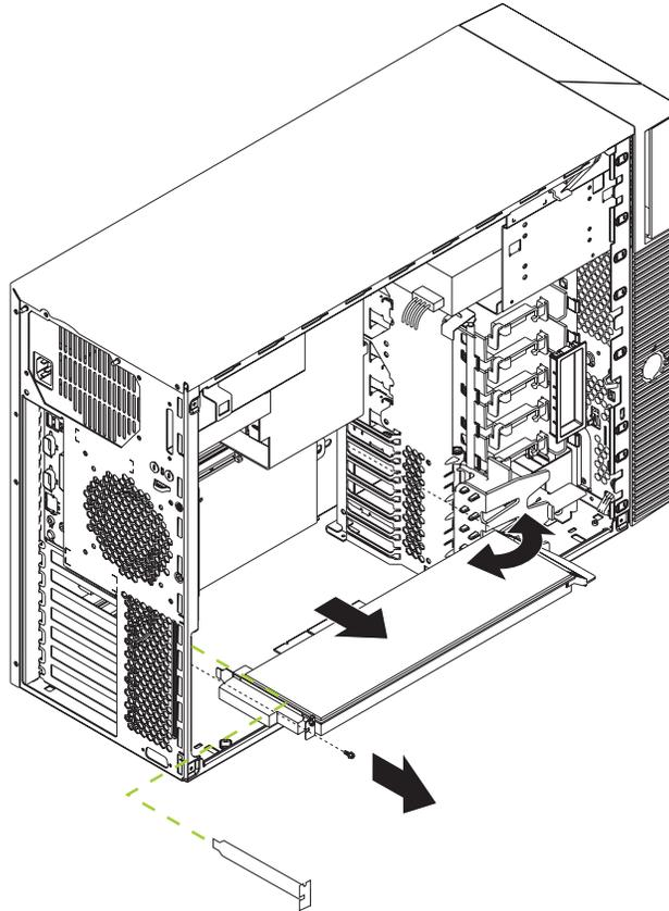
6. Remove the PCI adapter retention bracket or the adapter retention screw (depending on the model) from the rear of the system and remove the expansion slot cover.
