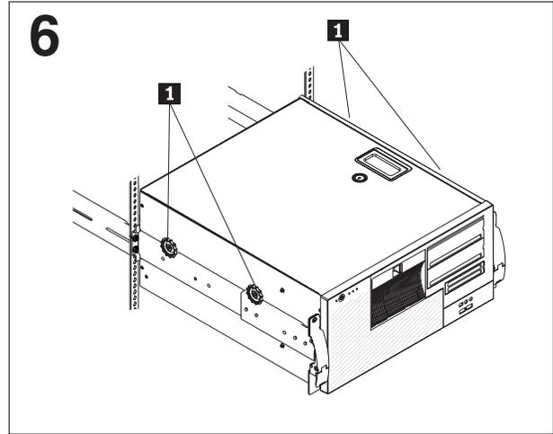
Fully extend the slide rails out of the rack cabinet; then, lift the system above the rails and rest the rack-support wheels **1** on the slide rails.
