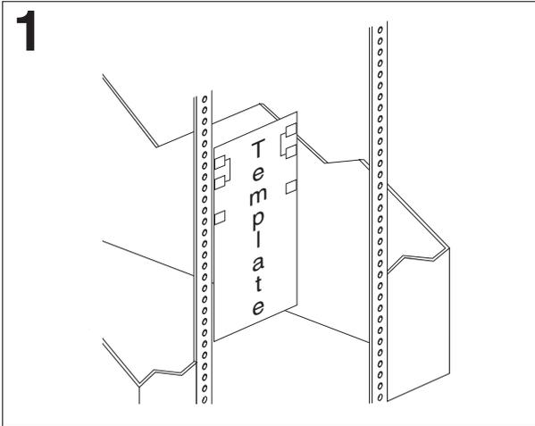
Use a pencil or marker to mark the holes on the front and rear of the rack as indicated by the arrows on the attached template.
