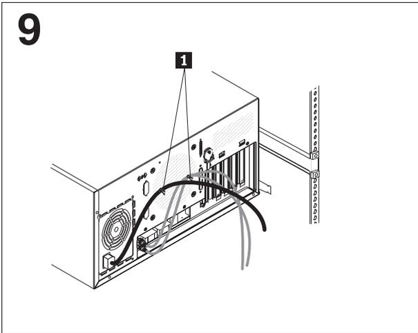
Attach the power, keyboard, mouse, and monitor cables (if required) to the system and route them through the cable clamps **1**; then, attach all other required cables to the system.
