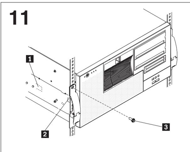
Press in on the safety latch **1** and slide the system into the rack cabinet until the release latches **2** snap into place; then, insert the M6 screws **3** through the release-latch-bracket assembly.
