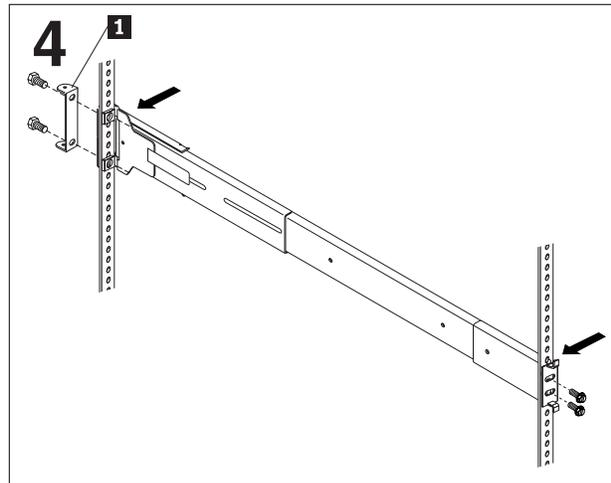
Use two M6 screws to attach the slide rail to the front of the rack cabinet (left-front of the rack cabinet shown in this step); then, use two M6 screws to attach the slide rail and hinge bracket **1** on the right-rear of the rack cabinet.
