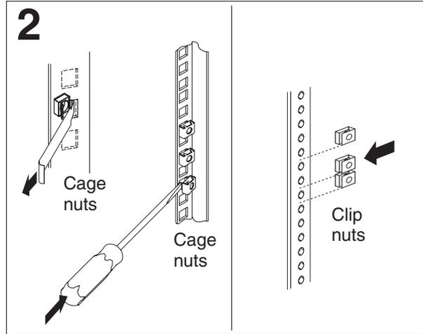
Install cage nuts or clip nuts as required for your rack. Use the cage-nut-insertion tool or a flat-blade screwdriver to install cage nuts.
