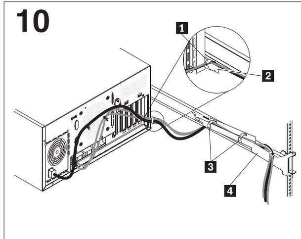
Use a cable strap **1** to attach all of the cables to the cable-retainer bracket **2** on the cable-management arm **4**.
