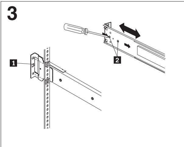
Use the tab **1** on the rear of the slide rails to align the slide rail to the rear of the rack cabinet. If it is necessary to adjust the length of the slide rail, loosen the screws **2** on the rear of the rail.
