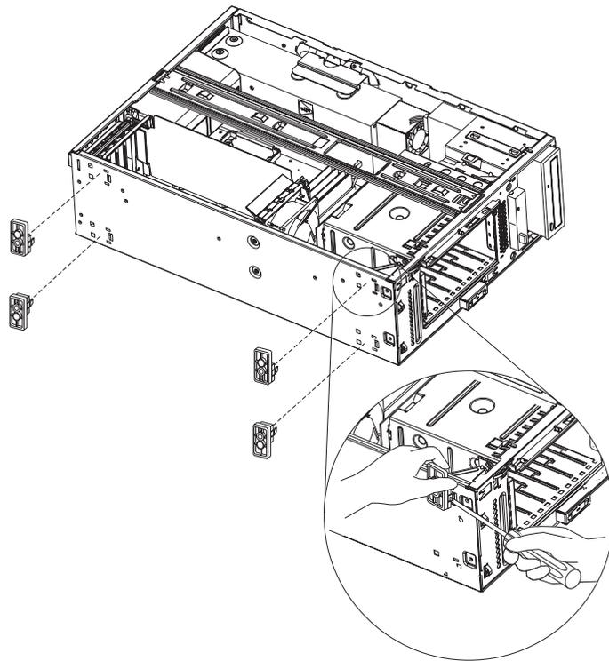
Figure 4. Removing the system feet
