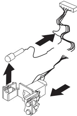
Figure 7. Rerouting the LED cable
