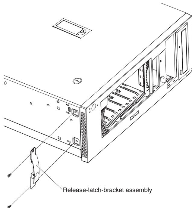
*Figure 15. Installing the release-latch-bracket assemblies*
