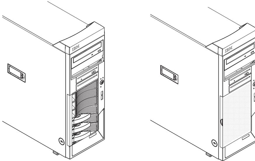
1. If hot-swap hard disk drives are installed in the system, note the hard disk drive locations; then, remove them according to the documentation that comes with your system and remove the drive-bay filler panels.
