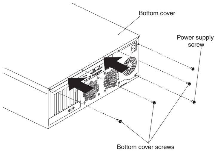
Figure 13. Installing the new bottom cover
