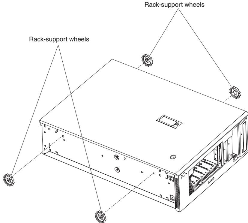
*Figure 16. Attaching the rack-support wheels*
