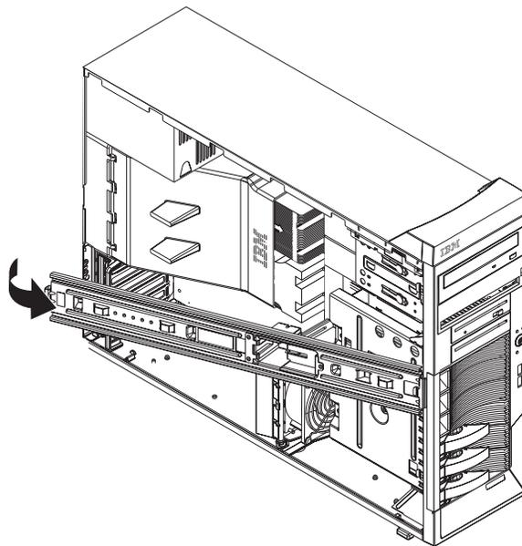
Figure 2. Removing the frame-support bracket
