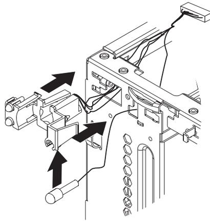
*Figure 8. Installing the power-switch and LED assembly in the rack-mount position*
