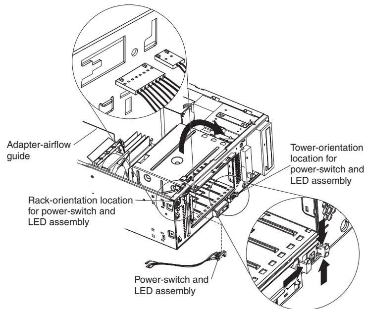
Figure 5. Relocating the power-switch and LED assembly
