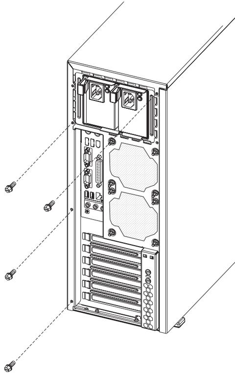
Figure 12. Removing the right-side cover
