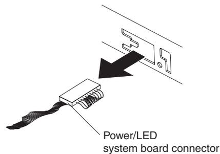
7. Fold the connector sideways onto the cable so that it will pass through the opening in the chassis; then, gently pull the power-switch and LED panel cable out of the chassis.
