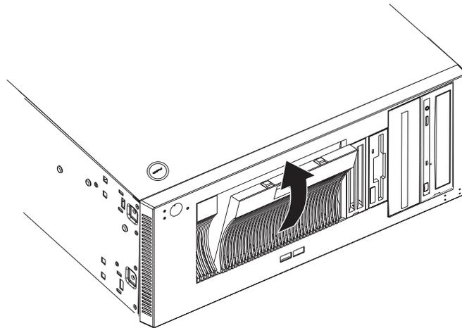
10. Install the release-latch-bracket assemblies on the system:
