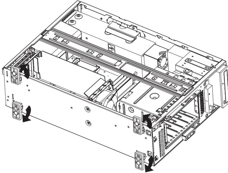
*Figure 3. Rotating the system feet*
