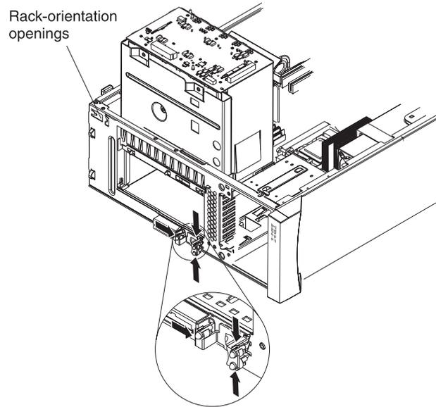
*Figure 6. Relocating the power-switch and LED assembly*
