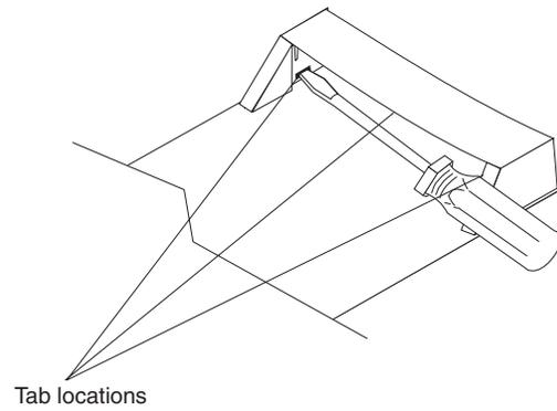
*Figure 10. Removing the plastic cover from the handle*
