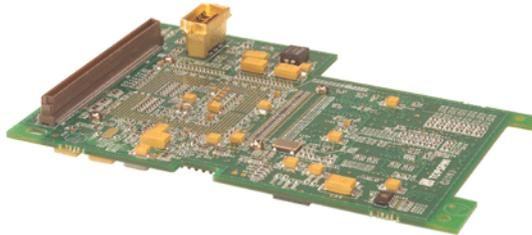
**Figure 1-1:** Infiniband Host Channel Adapter Expansion Card for IBM eServer BladeCenter
