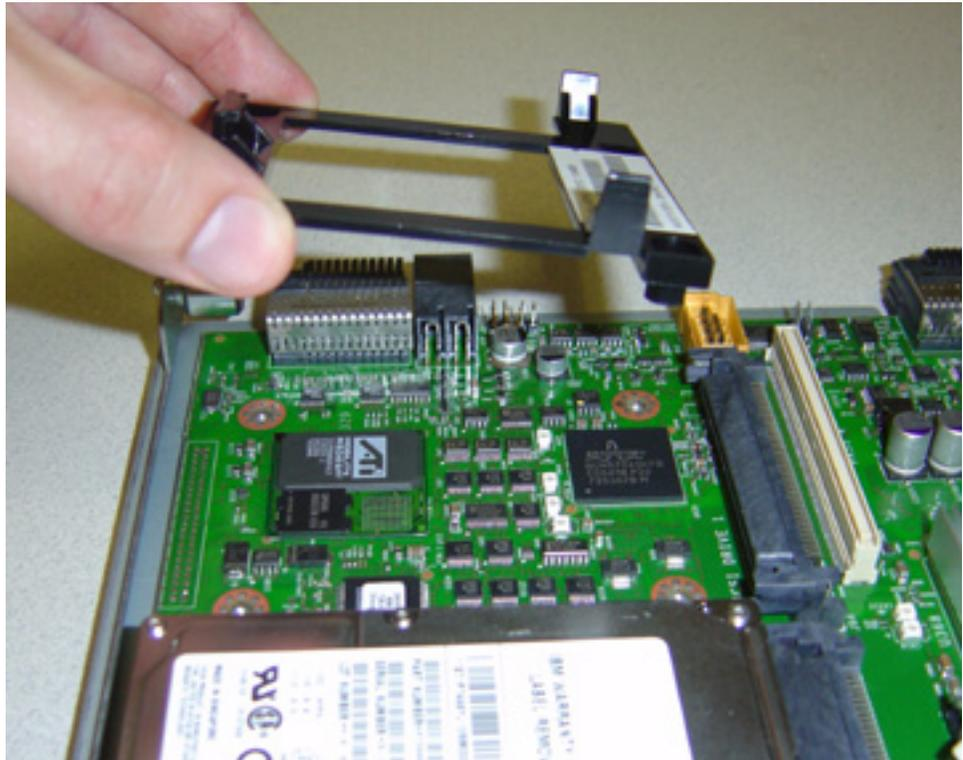
2. Secure the HCA Expansion Card tray to the blade server with the screws provided.
