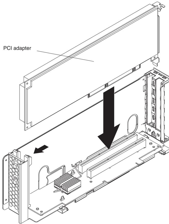
7. If you removed the PCI low-profile-card cage to install the adapter, press the PCI low-profile-card cage *firmly* into the connector until the retention latch locks.
