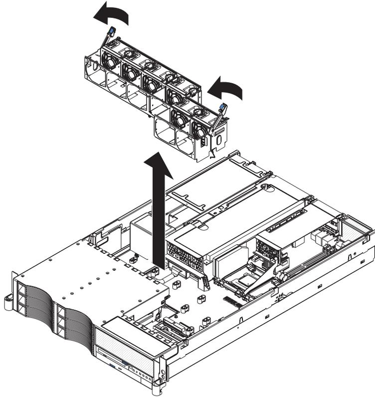
6. Remove the fan bracket from the server.
