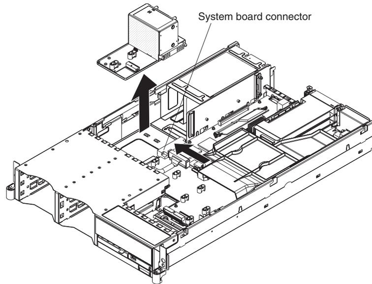
8. Remove the power cage assembly from the server.
