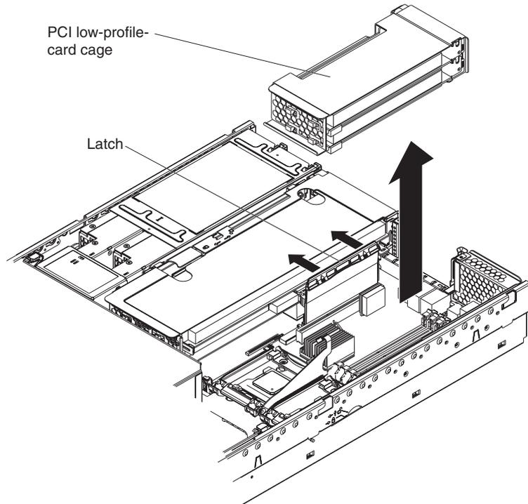
If you are installing an adapter in PCI slot 3 or 4, remove the PCI riser-card cage.
