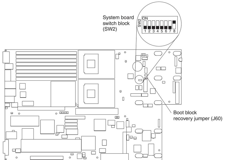
4. Move the jumper from pins 1 and 2 to pins 2 and 3 to enable the BIOS recovery mode.
