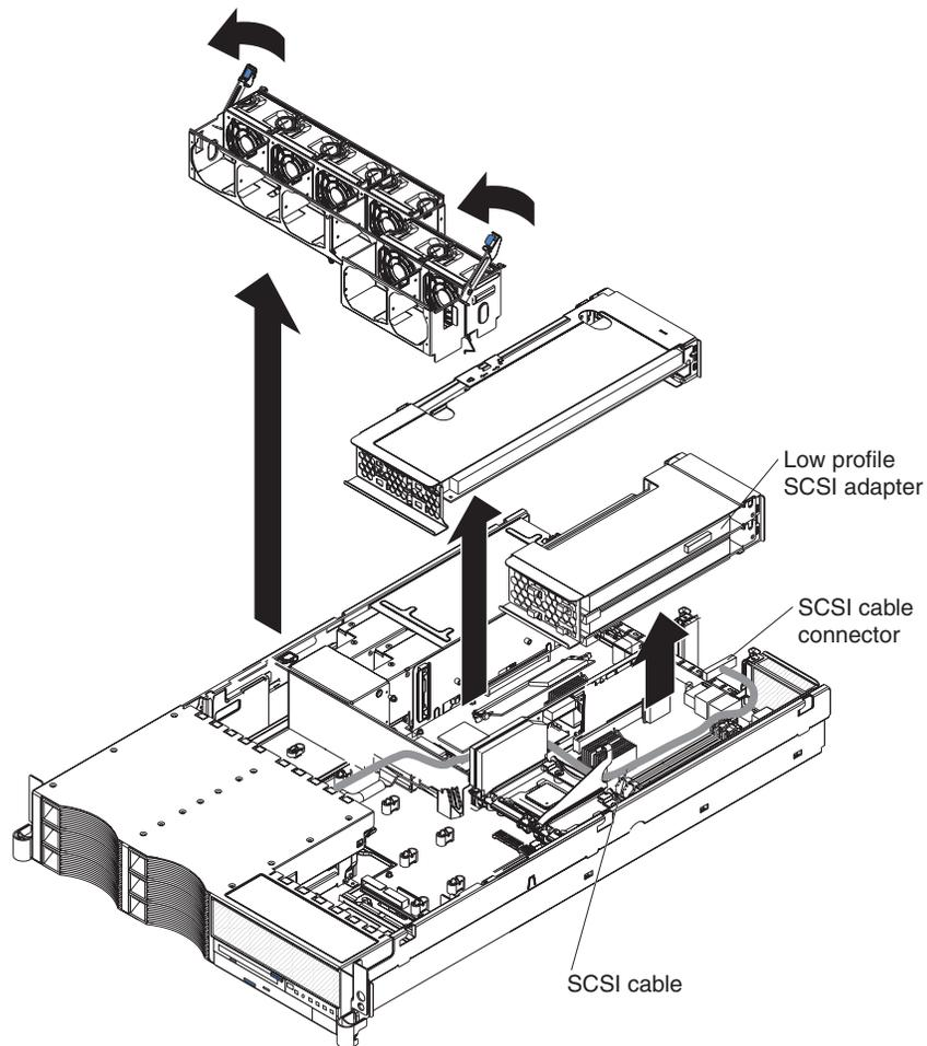
The following illustration shows the cable routing for an adapter installed in the PCI riser-card cage.
