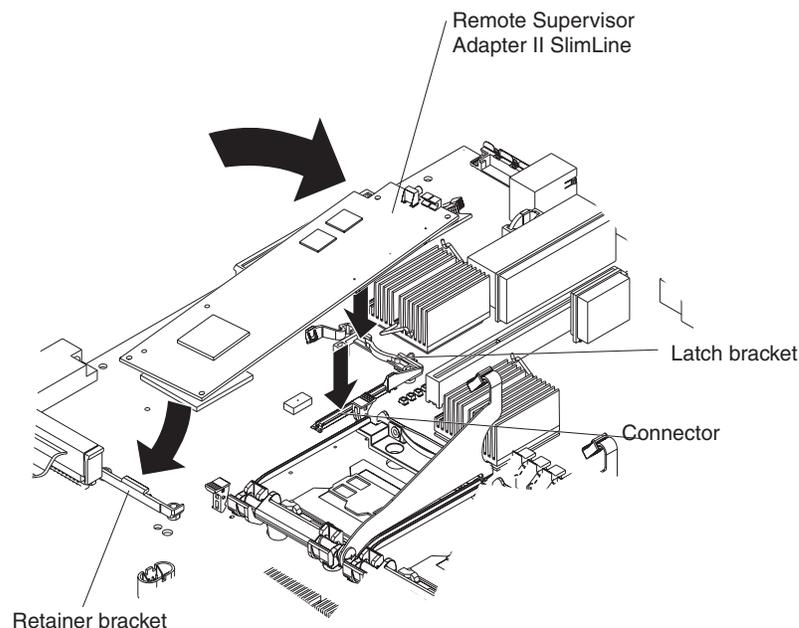
Slip the free end of the card under the tab on the retainer bracket; then, press the card in the connector and make sure that all tabs on the latch bracket secure the card in place.
