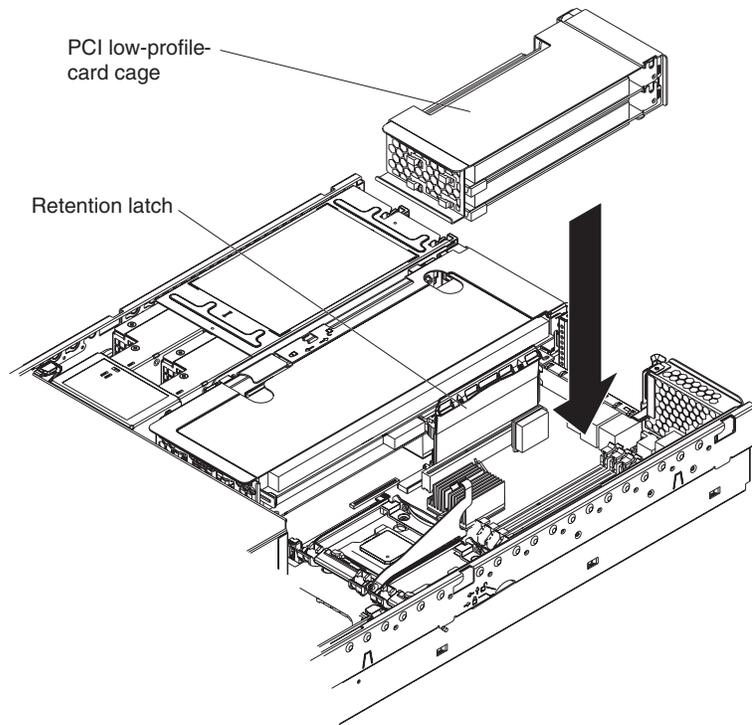
If you removed the PCI riser-card cage to install the adapter, press the PCI riser-card cage *firmly* into the connector and close the latch.
