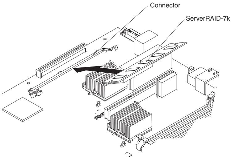
**Note:** If there is a gap between the card and the retaining clips, the card has not been properly installed. In this case, open the retaining clips and remove the card; then, reinsert the card.
