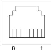
Connect a Category 3, 4, or 5 unshielded twisted-pair cable to this connector. 100BASE-TX and 1000BASE-T Fast Ethernet standards require Category 5 or higher cabling.
