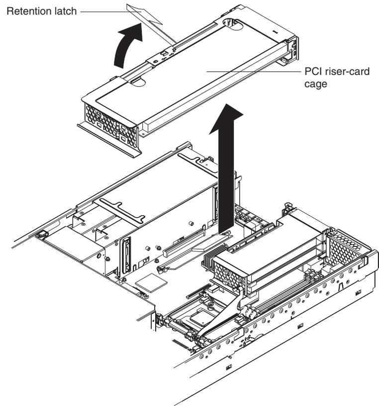
5. Slide the expansion-slot cover out of the PCI low-profile-card cage or PCI riser-card cage.
