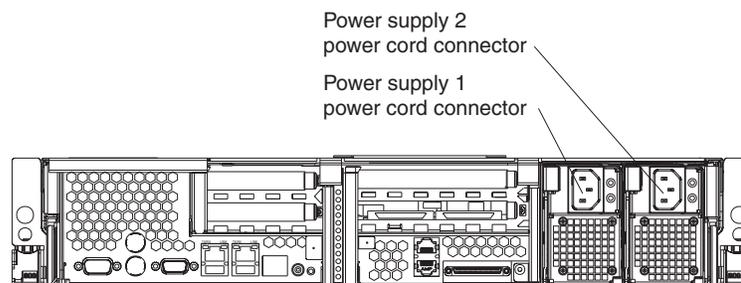
5. Connect the power cord to a properly grounded electrical outlet.
