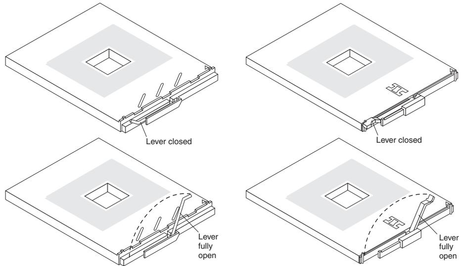
7. **Attention:** Do not use excessive force when removing the microprocessor from the socket.
