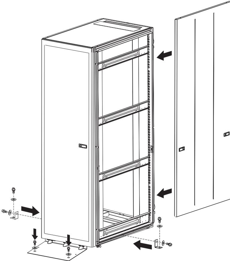
Figure 7. Installing the side stabilizer brackets
