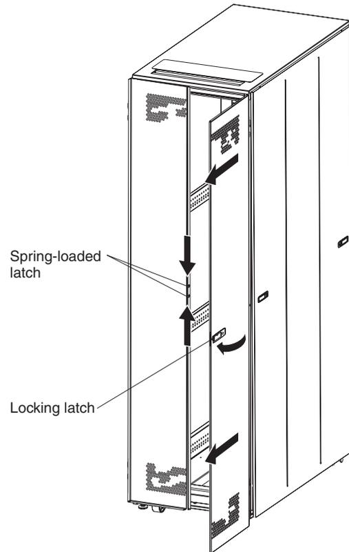
Figure 11. Opening and removing the rear doors
