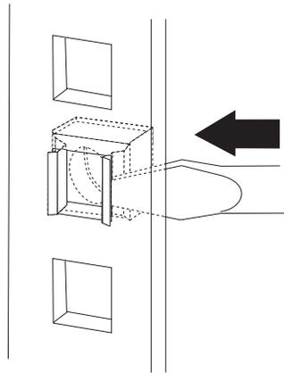
Figure 18. Installing cage nuts with a flat-blade screwdriver
