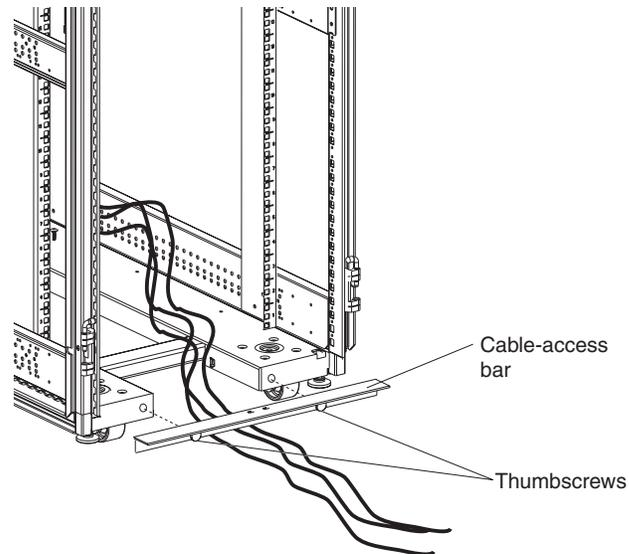
*Figure 20. Routing cables using the cable-access bar*
