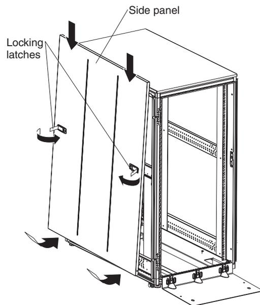
Figure 9. Installing a side panel
