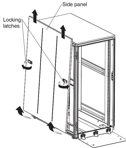
Figure 8. Removing a side panel
