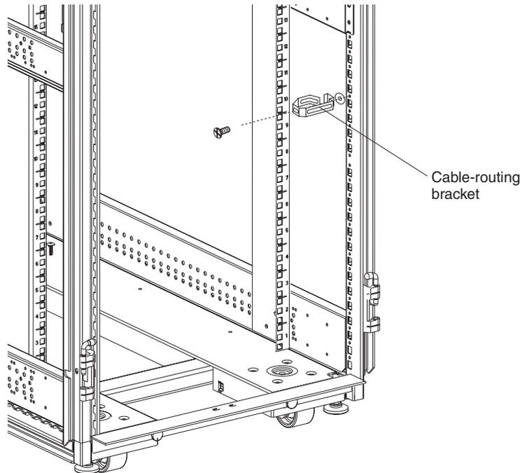
Figure 19. Cable-routing bracket
