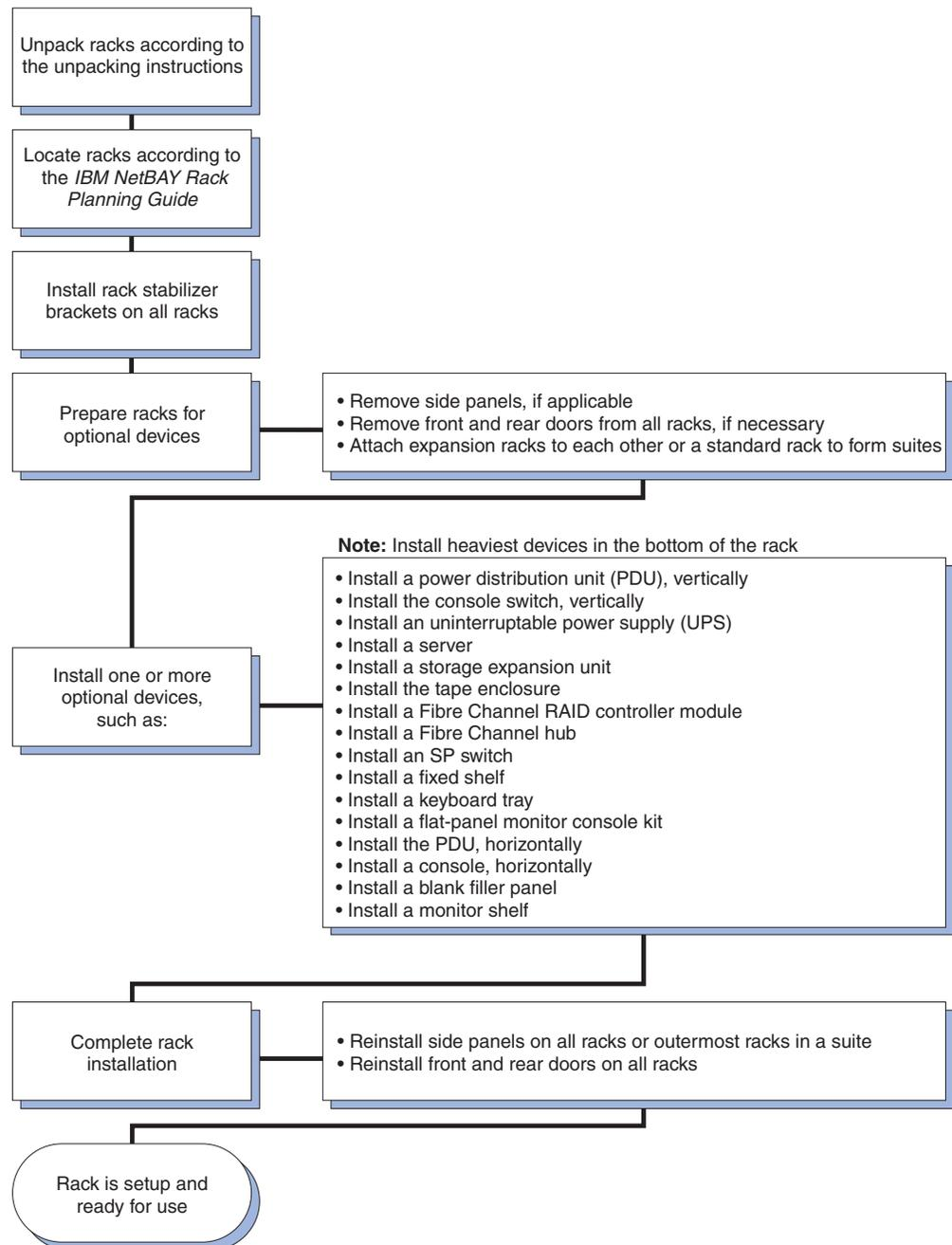
Figure 1. Installing the rack and devices overview
