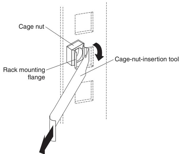
Figure 17. Installing cage nuts with the cage-nut-insertion tool
