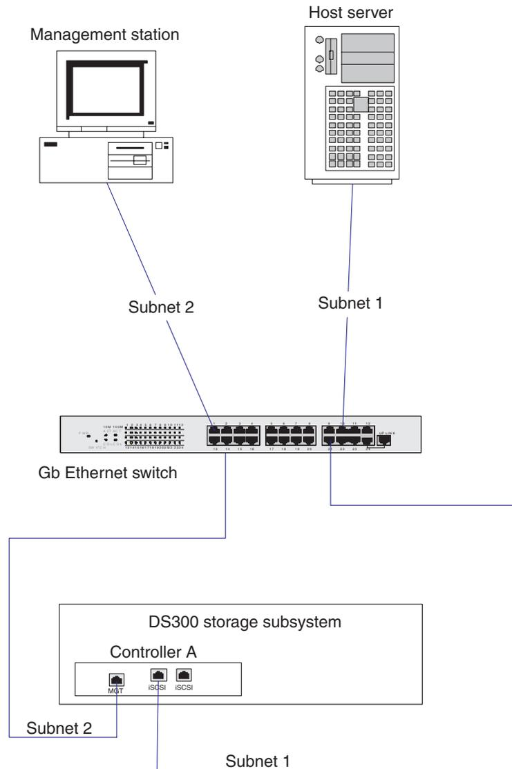
Figure 8. Single port, single server configuration (DS300)
