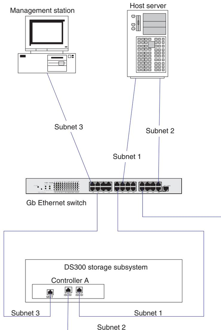
Figure 9. Multiple port, single server configuration (DS300)
