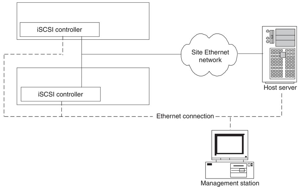
Figure 7. Direct management of iSCSI storage subsystems
