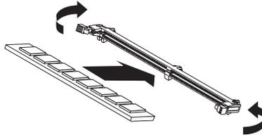
Figure 40. Inserting a DIMM into the connector
