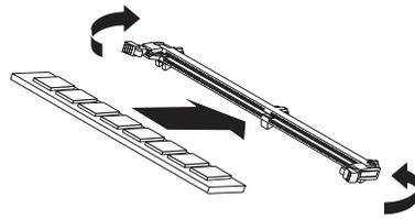
Figure 45. Inserting a DIMM into the connector
