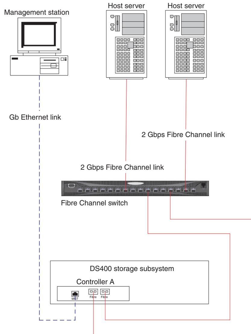
Figure 14. Multiple server, single storage subsystem configuration (DS400)
