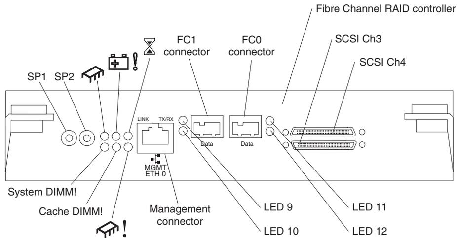
Figure 30. Fibre Channel RAID controller LEDs and connectors
