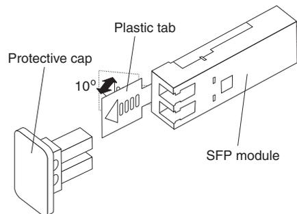
Figure 19. Unlocking an SFP module - plastic tab
