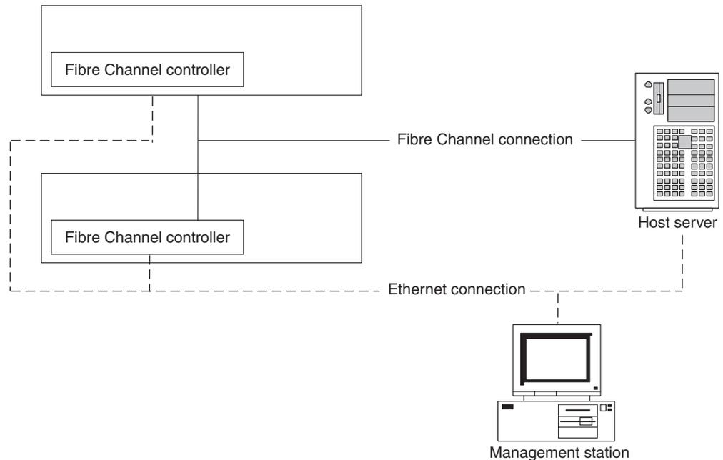
Figure 6. Direct management of Fibre Channel storage subsystems
