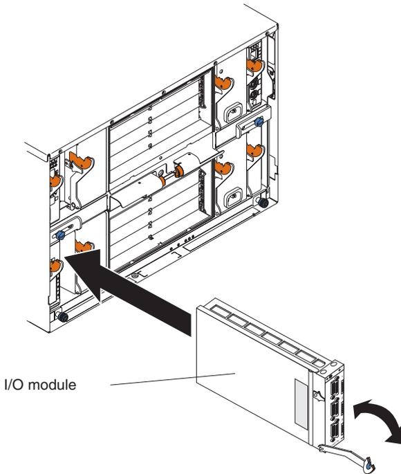
Complete the following steps to install a copper pass-thru module:
