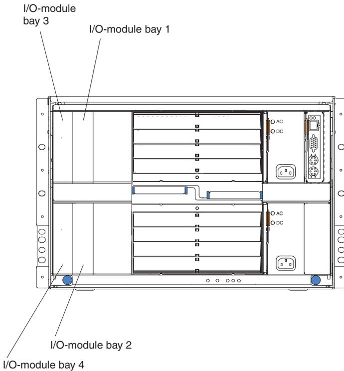
**Attention:** To maintain proper system cooling and performance, each module bay must contain either a module or a filler module; each blade bay must contain either a blade server, expansion unit, or a filler blade.
