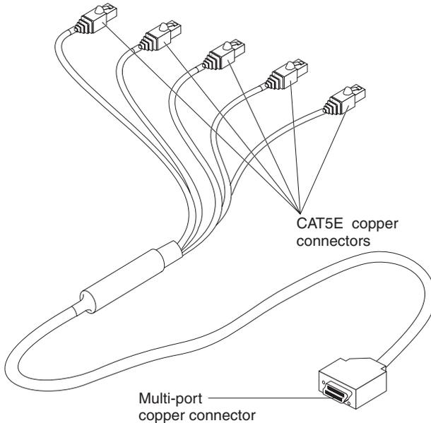
The CAT5E cable connectors that are attached to your network infrastructure are numbered to identify their port channel. See Table 1 on page 22 for blade-server-to-port mapping information.
