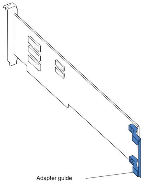
6. Press the adapter *firmly* into the expansion slot, lower the adapter-retention latch, and make sure that the latch is in the locked (closed) position.
