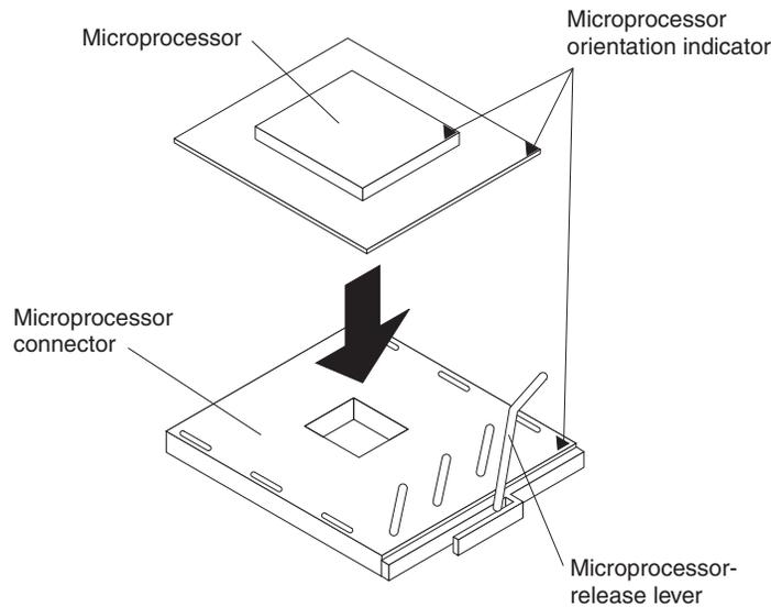
d. Close the microprocessor release lever to secure the microprocessor.
