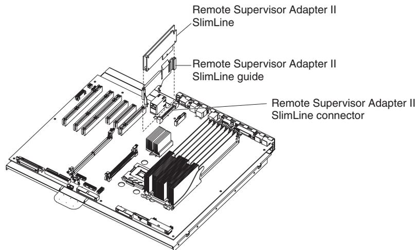
5. Position the entire adapter assembly so that the edge connector on the Interposer card is at the rear of the server.
