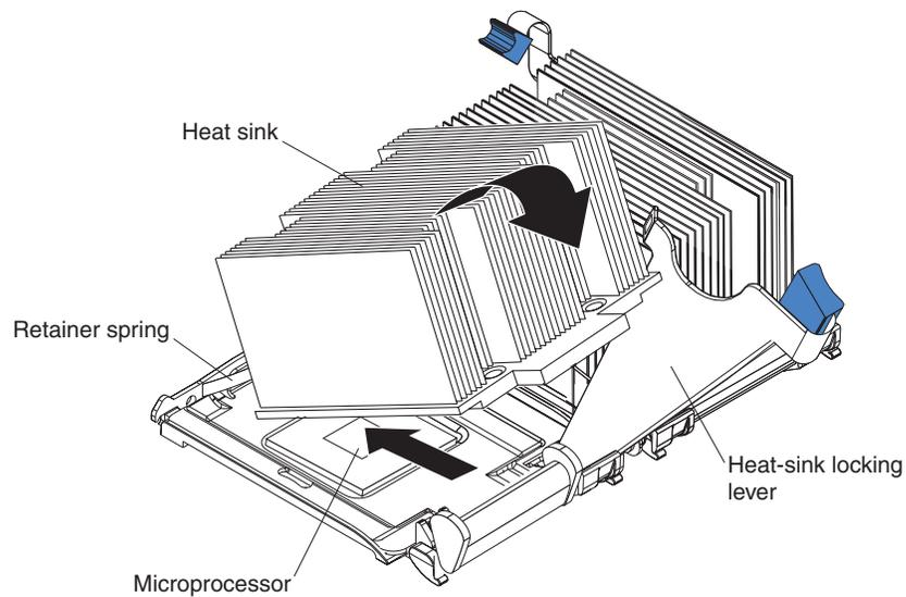
7. Open the heat-sink release lever and install a heat sink on the microprocessor; then, close the release lever.
