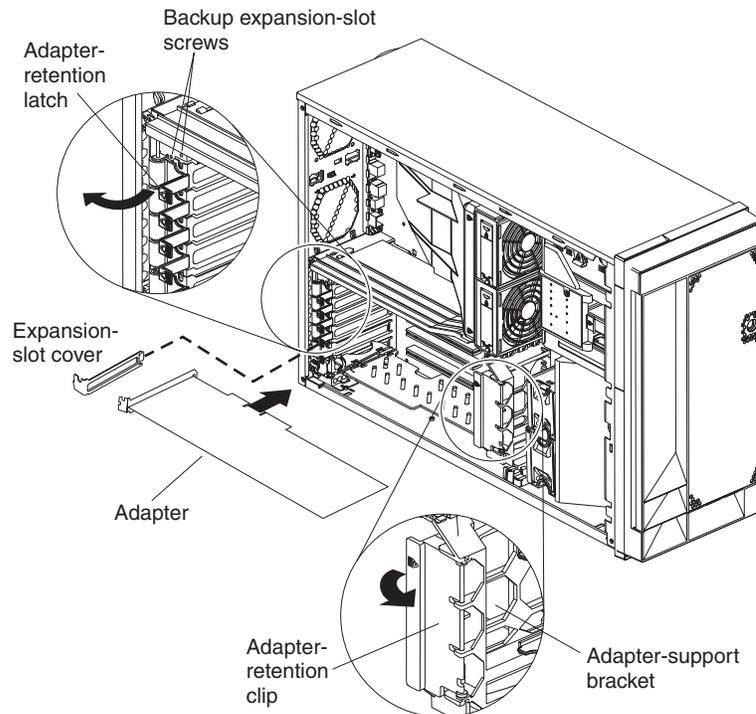
5. If you are installing a full-length adapter, remove the blue adapter guide (if any) from the end of the adapter; then, lift the adapter-retention clip on the adapter-support bracket. Otherwise, continue with the next step.
