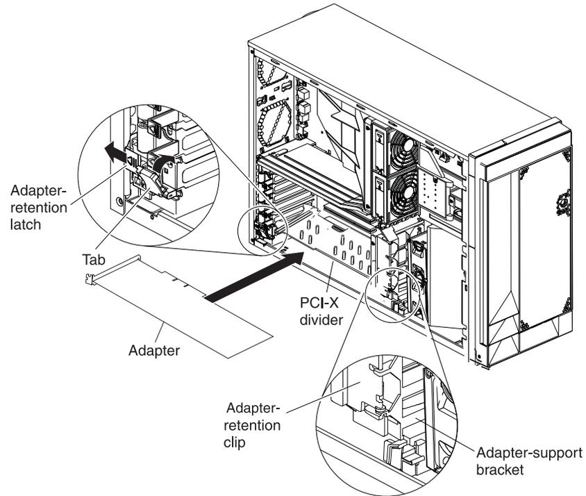
Complete the following steps to install a hot-plug PCI or PCI-X adapter:
